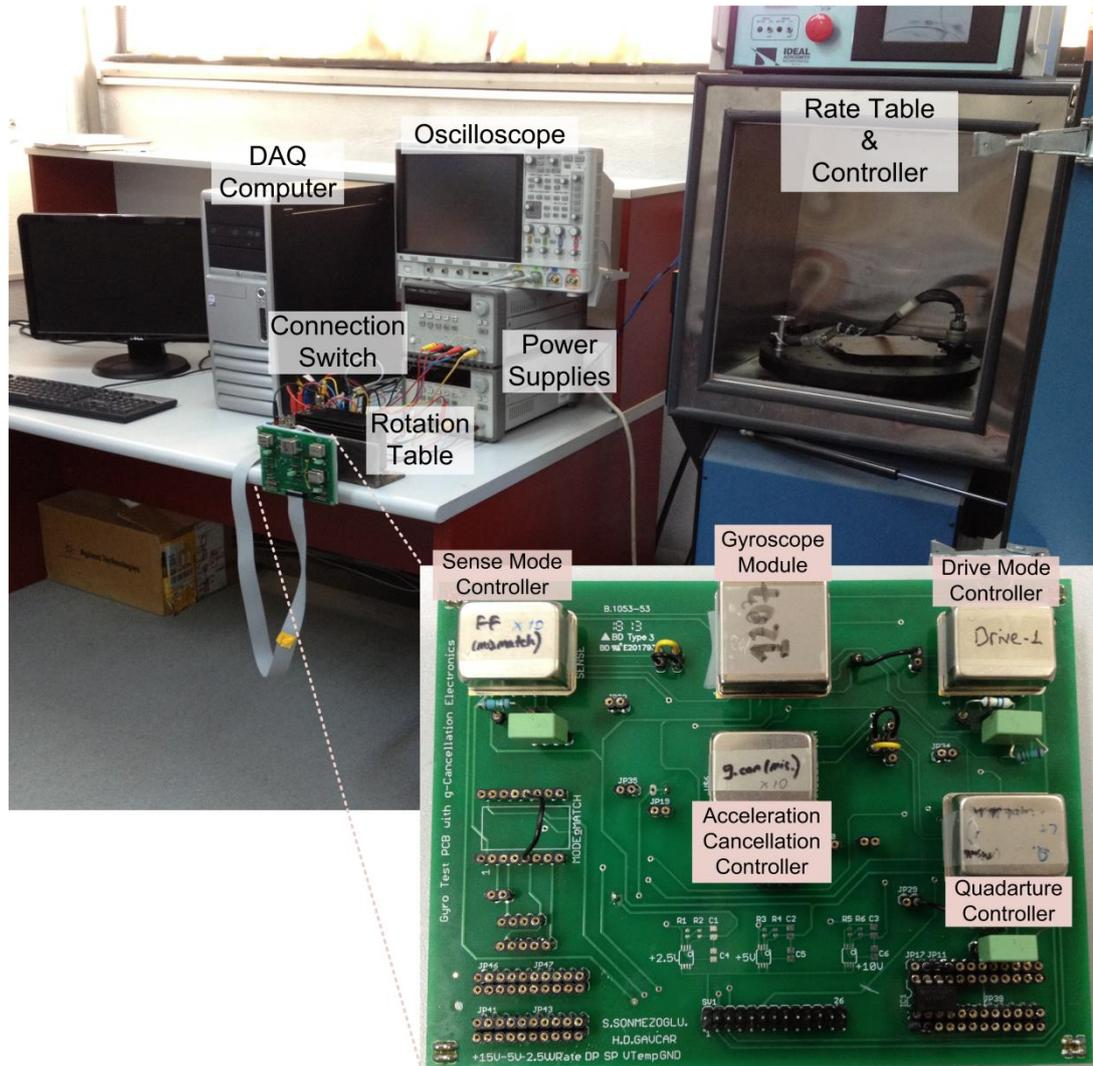
Figure 5.3: Test setup for the system level tests.
