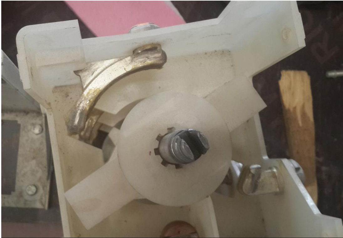
Figure 18: The photo of rotating central axis that the rotation of the mechanism moves around
