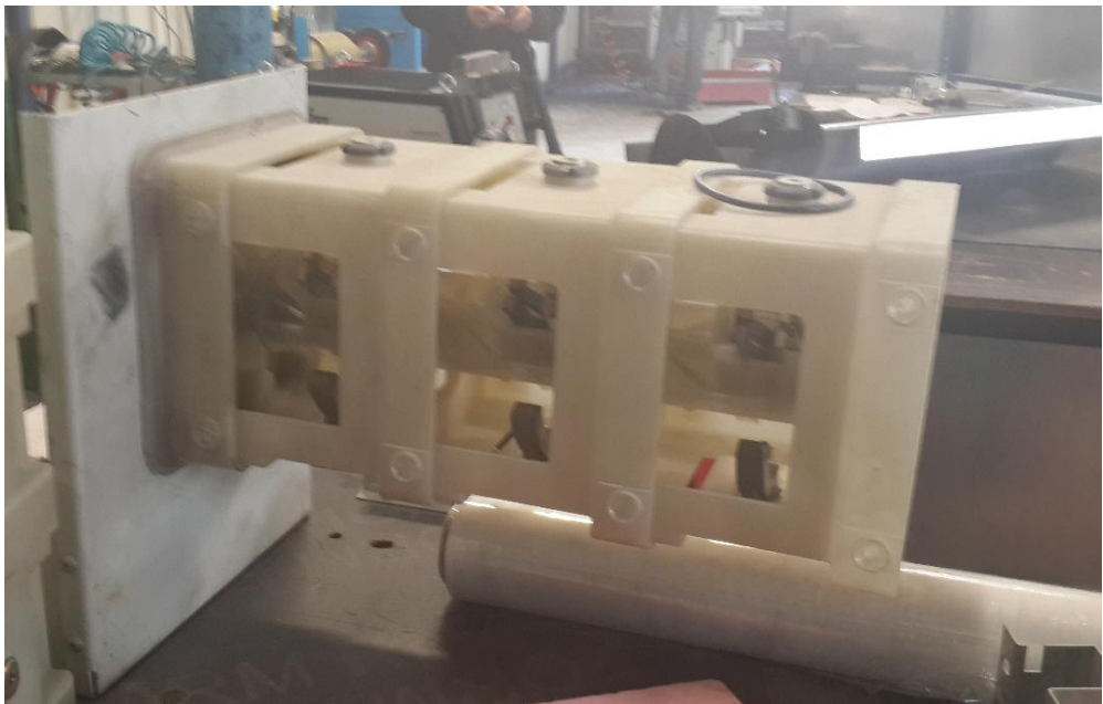
Figure 23: The photo of load break switch with the contacts and the mechanism
