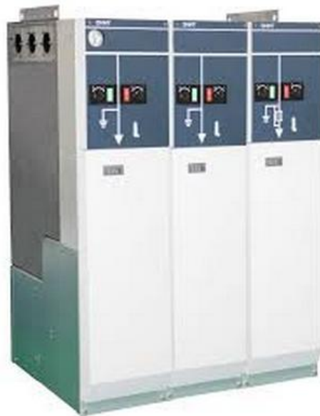
Figure 2: 12 kV Modular type gas insulated switchgear as incoming and outgoing feeder with load break switch and transformer protection with load break switch and fuse combination
