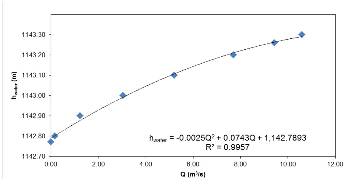
Figure 3.13 Stage - Discharge curve for the weir
