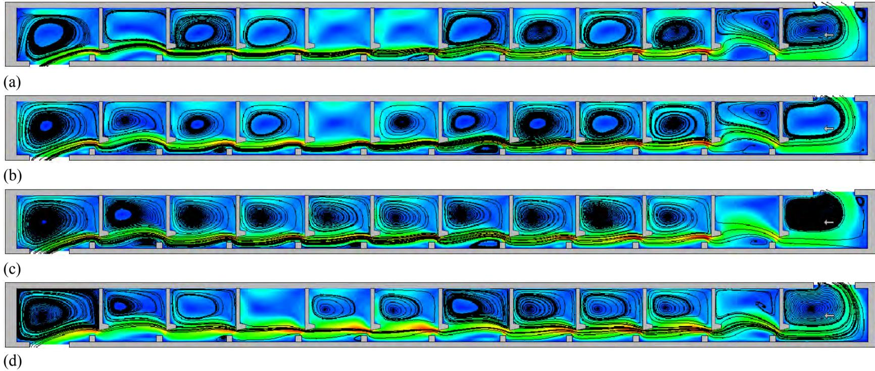
Figure 3.24 Velocity magnitude contours and streamlines of Type I for the maximum flow case at flow depths of: (a)  $0.10h_u$ ; (b)  $0.25h_u$ ; (c)  $0.50h_u$ ; (d)  $0.75h_u$
