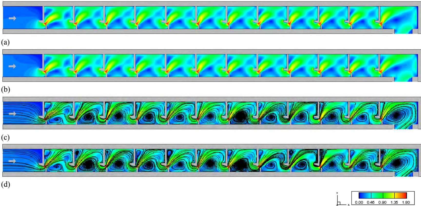
Figure 3.18 (a) Velocity contours (mesh size 0.03 m.) (b) Velocity contours (mesh size 0.035 m.) (c) Velocity streamlines (mesh size 0.03 m.) (d) Velocity streamlines (mesh size 0.035 m.) (all sections are taken from the middle of the water depth)
