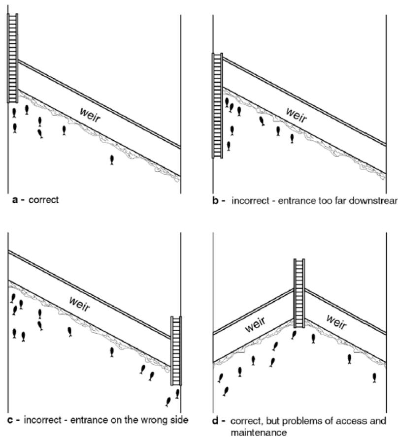
Figure 2.3 Schematic plans of correct location of fishway entrance (Larinier, 1992d)
