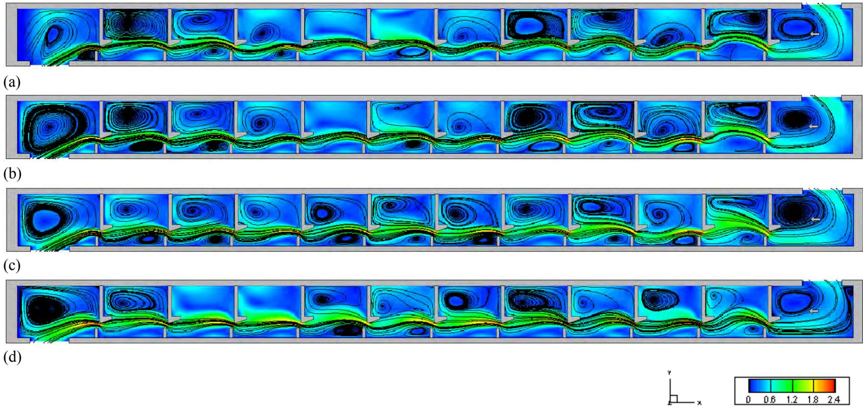
Figure 3.36 Velocity magnitude contours and streamlines of Type III for the maximum flow case at flow depths of: (a)  $0.10h_u$ ; (b)  $0.25h_u$ ; (c)  $0.50h_u$ ; (d)  $0.75h_u$
