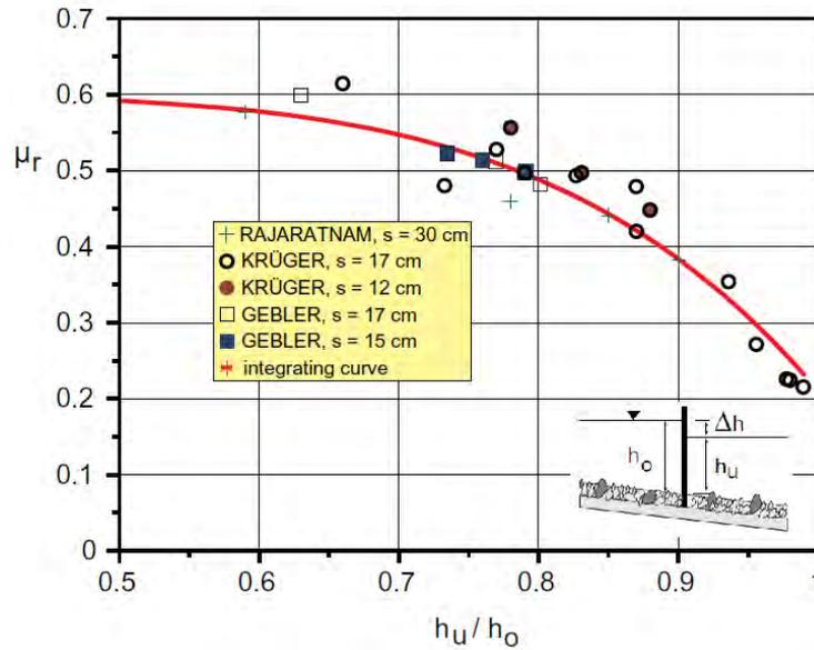
Figure 2.14 Discharge coefficient  $\mu_r = f(h_u / h_o)$  (DVWK, 1996)
