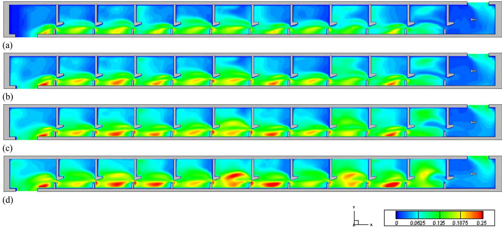
Figure 3.37 Turbulent kinetic energy contours of Type III for the maximum flow case at flow depths of: (a)  $0.10h_u$ ; (b)  $0.25h_u$ ; (c)  $0.50h_u$ ; (d)  $0.75h_u$
