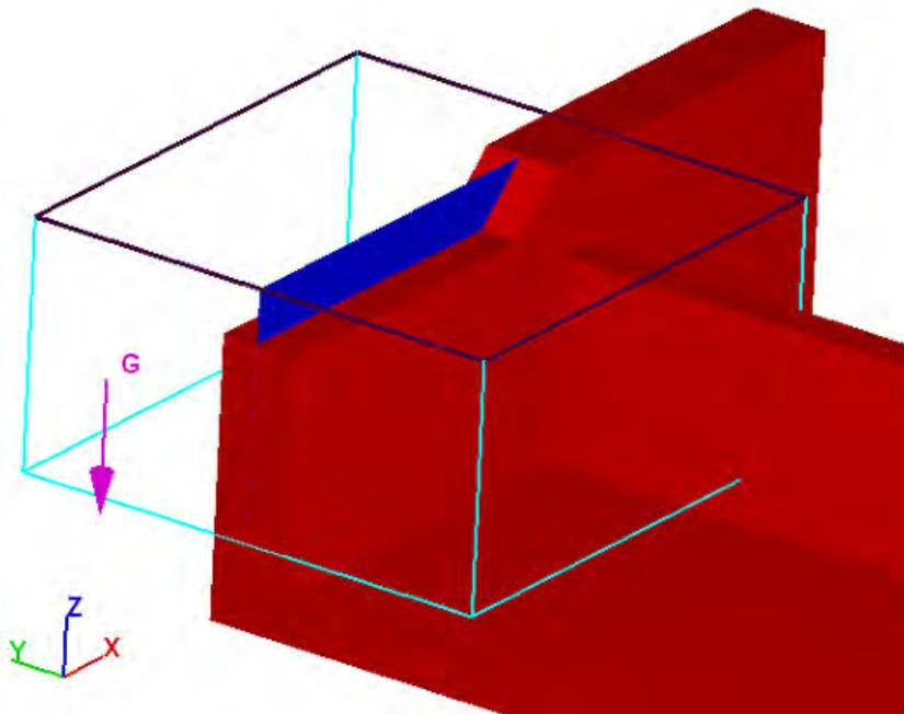
Figure 3.12 Computational domain of the weir
