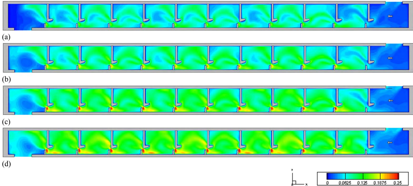
Figure 3.31 Turbulent kinetic energy contours of Type II for the maximum flow case at flow depths of: (a)  $0.10h_u$ ; (b)  $0.25h_u$ ; (c)  $0.50h_u$ ; (d)  $0.75h_u$
