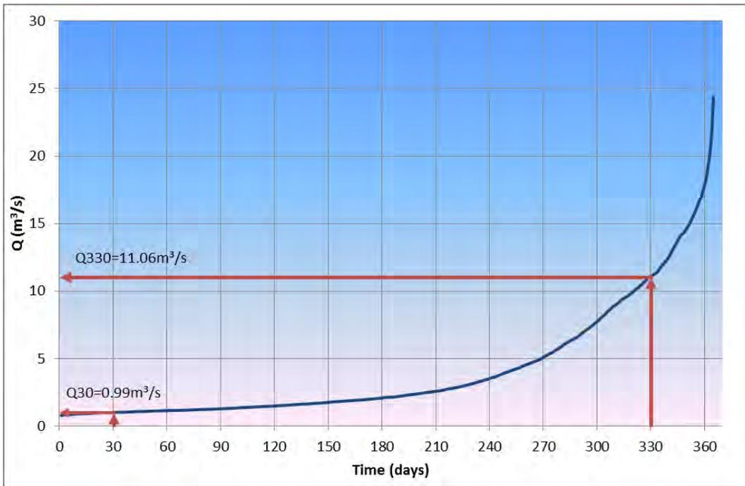
Figure 3.7 Discharge rating curve of 22-07 Haldizen Station
