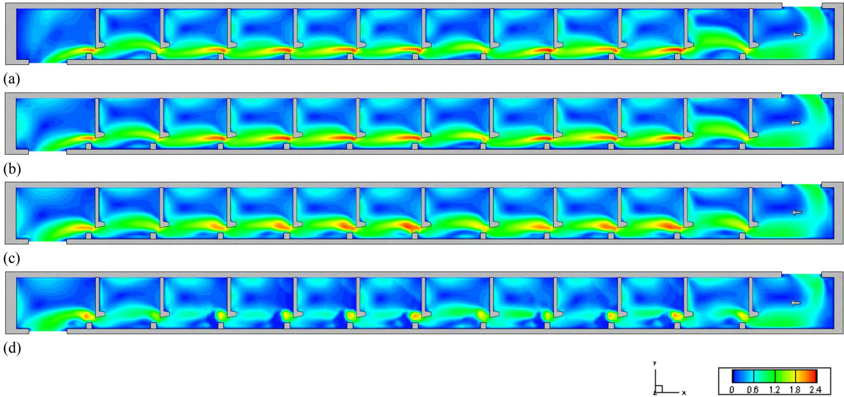
Figure 3.20 Velocity magnitude contours of Type I for the minimum flow case at flow depths of: (a)  $0.10h_u$ ; (b)  $0.25h_u$ ; (c)  $0.50h_u$ ; (d)  $0.75h_u$
