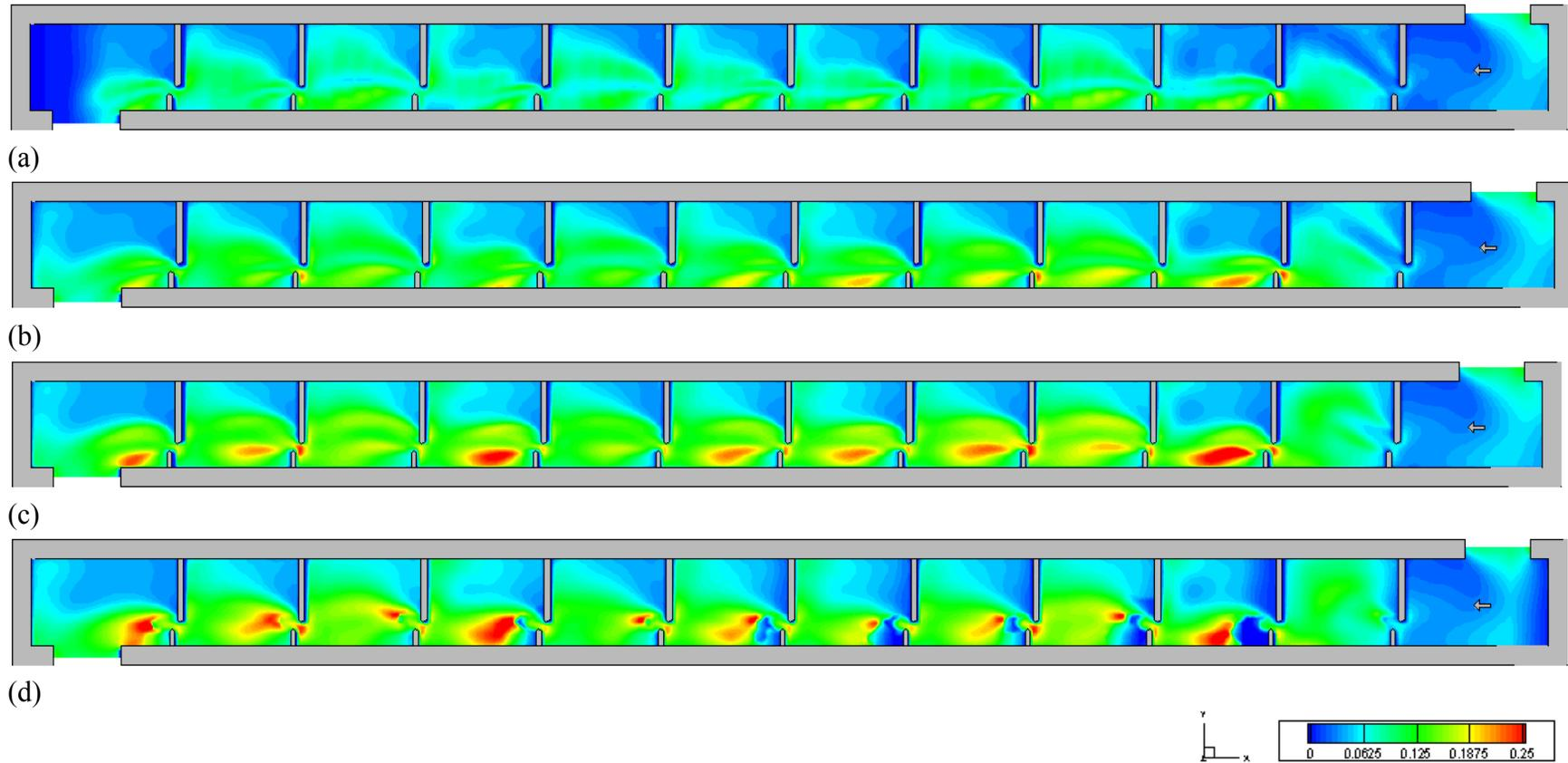
Figure 3.41 Turbulent kinetic energy contours of Type IV for the minimum flow case at flow depths of: (a)  $0.10h_u$ ; (b)  $0.25h_u$ ; (c)  $0.50h_u$ ; (d)  $0.75h_u$
