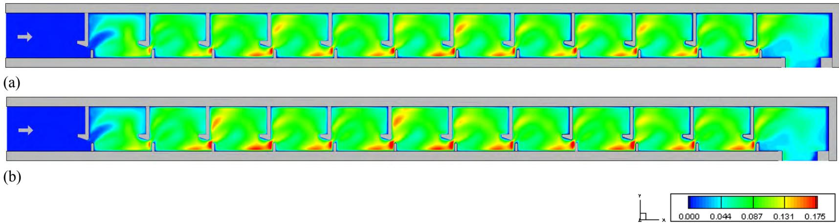
Figure 3.19 (a) Turbulent kinetic energy contours (mesh size 0.03 m.) (b) Turbulent kinetic energy contours (mesh size 0.035 m.) (all sections are taken from the middle of the water depth)
