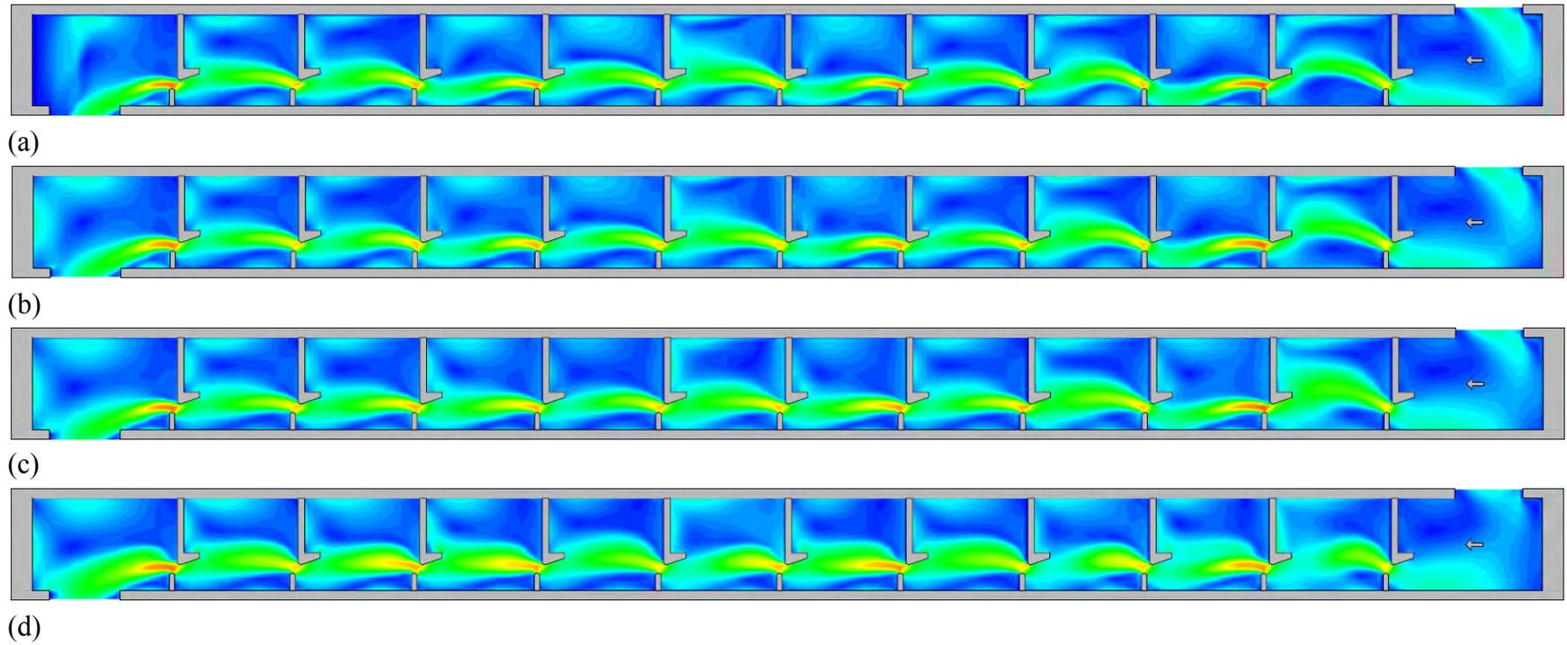
Figure 3.35 Velocity magnitude contours of Type III for the maximum flow case at flow depths of: (a)  $0.10h_u$ ; (b)  $0.25h_u$ ; (c)  $0.50h_u$ ; (d)  $0.75h_u$
