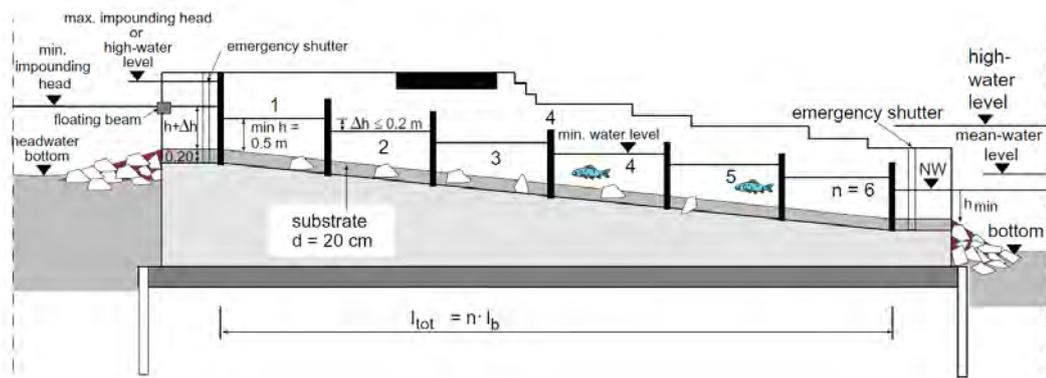
Figure 2.13 Longitudinal section of vertical slot pass (DVWK, 1996)
