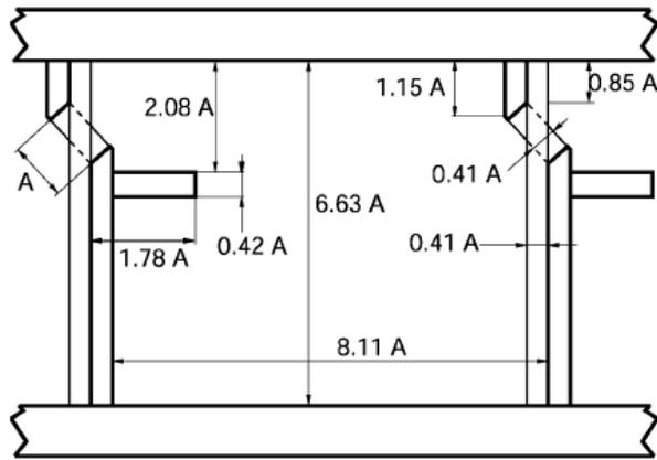
Figure 2.12 Characteristics of a simplified vertical slot fishway (Lenne, 1990)
