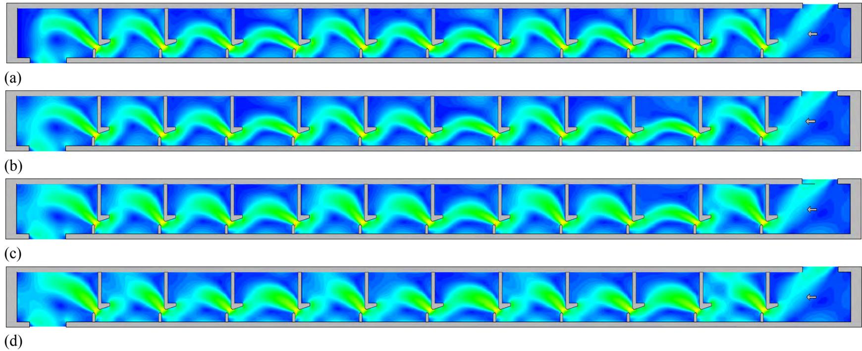
Figure 3.29 Velocity magnitude contours of Type II for the maximum flow case at flow depths of: (a)  $0.10h_u$ ; (b)  $0.25h_u$ ; (c)  $0.50h_u$ ; (d)  $0.75h_u$
