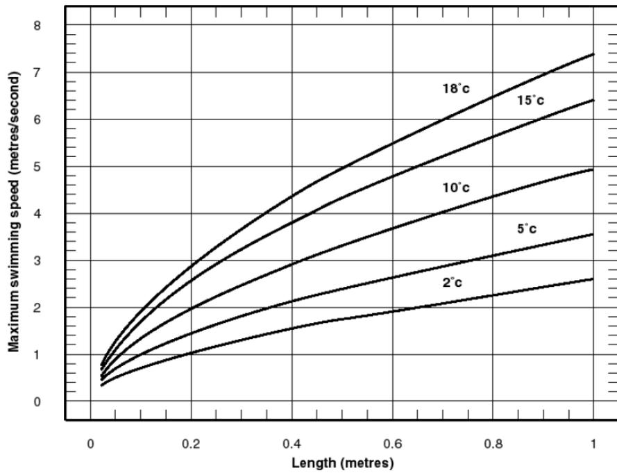
Figure 2.1 Maximum swimming speed for different fish sizes (Beach, 1984)
