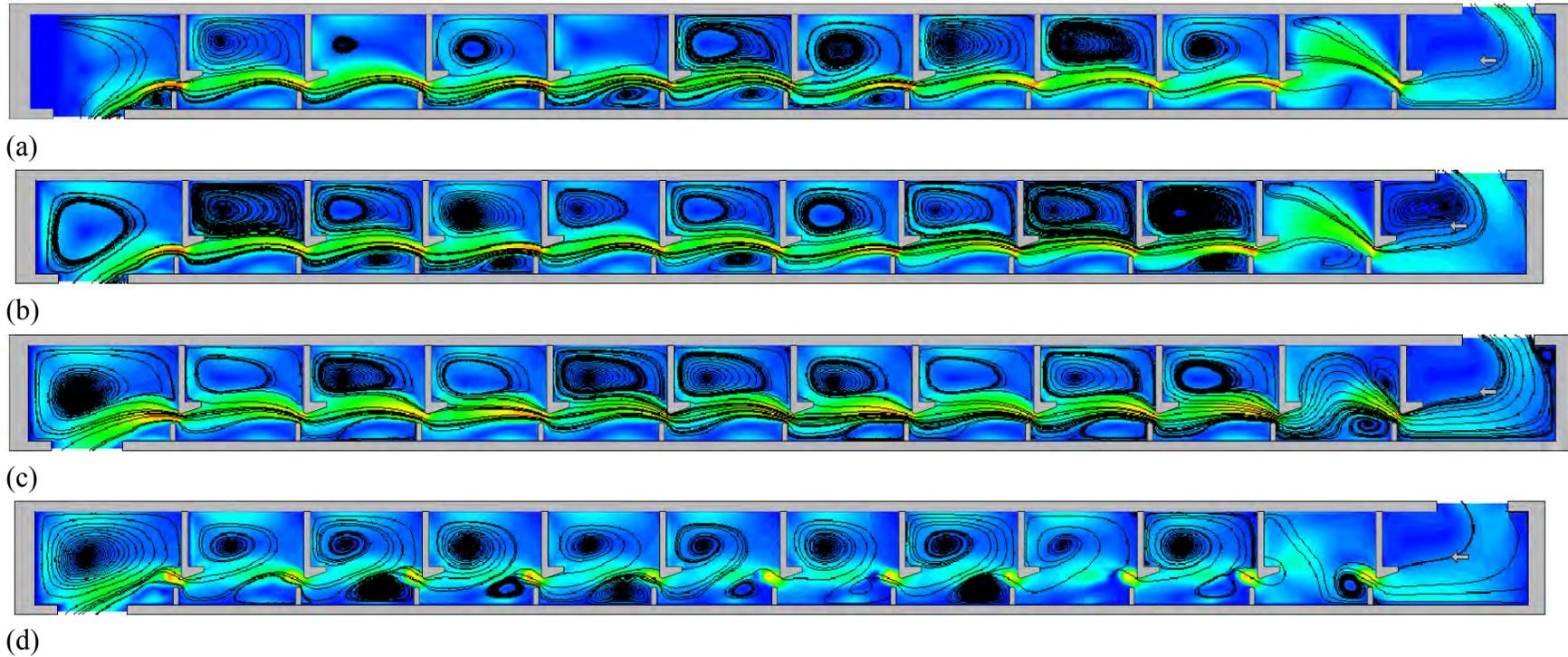
Figure 3.33 Velocity magnitude contours and streamlines of Type III for the minimum flow case at flow depths of: (a)  $0.10h_u$ ; (b)  $0.25h_u$ ; (c)  $0.50h_u$ ; (d)  $0.75h_u$
