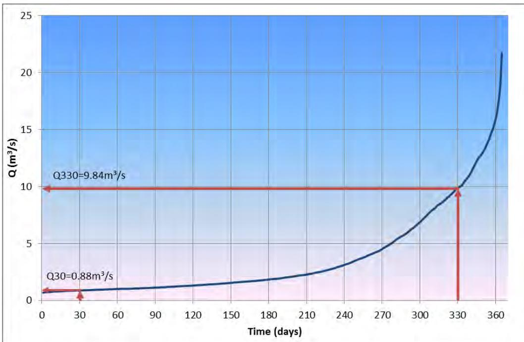
Figure 3.8 Discharge rating curve of Uzungöl
