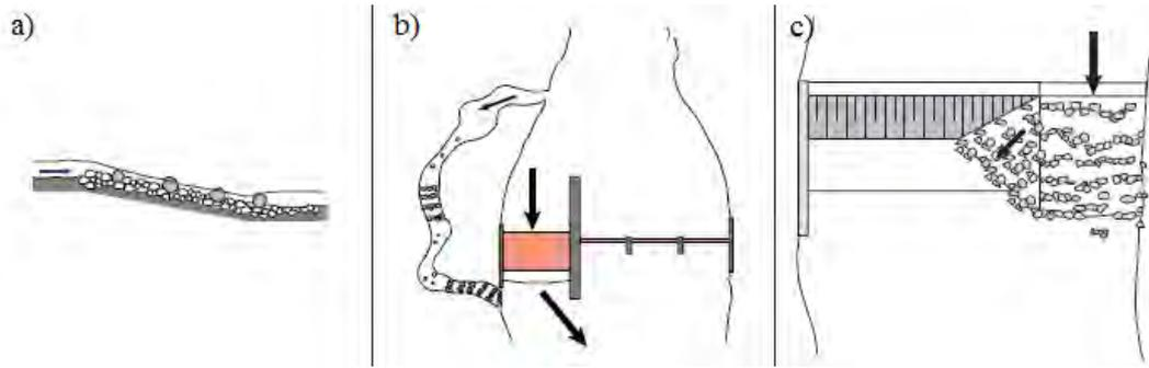
Figure 2.8 The three types of close-to-nature types of fish pass (DVWK, 1996)
