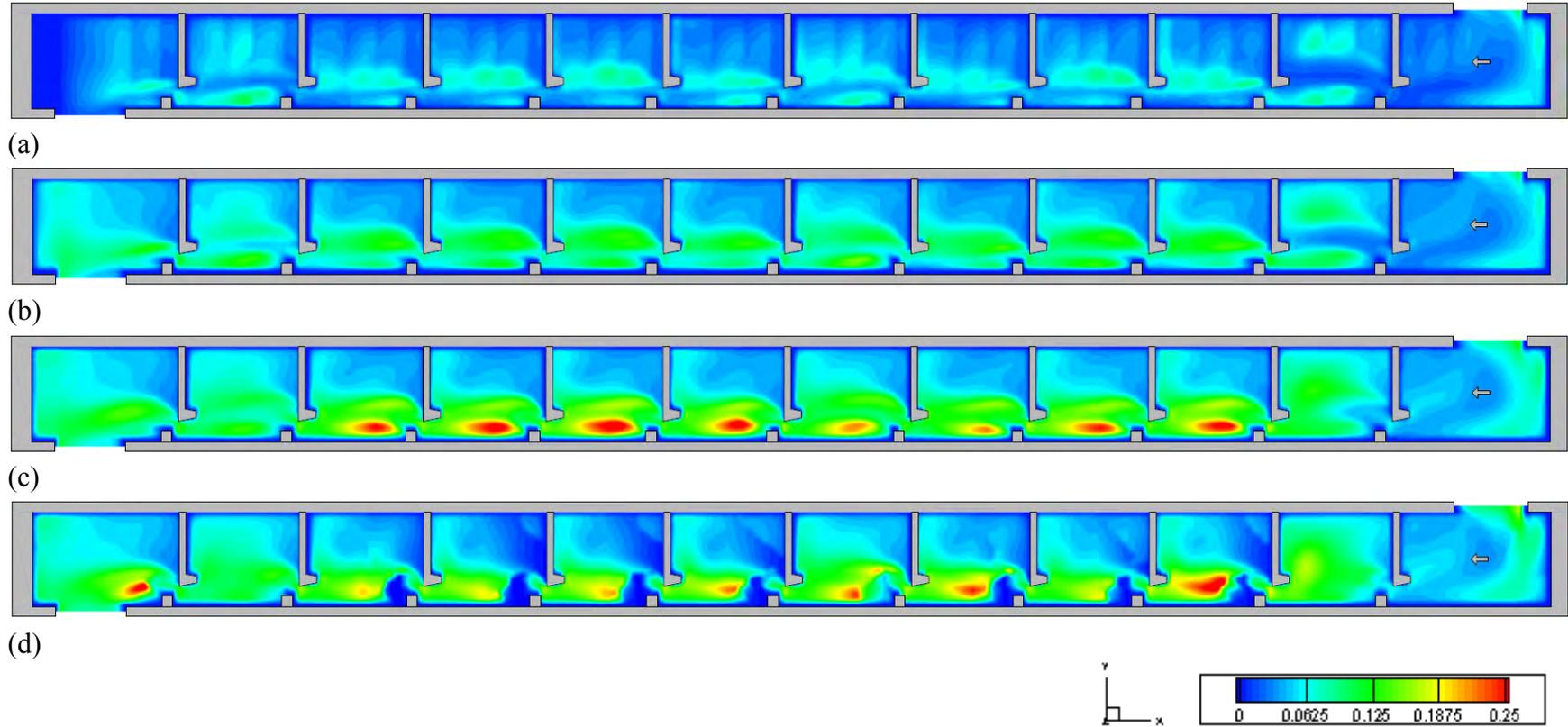
Figure 3.22 Turbulent kinetic energy contours of Type I for the minimum flow case at flow depths of: (a)  $0.10h_u$ ; (b)  $0.25h_u$ ; (c)  $0.50h_u$ ; (d)  $0.75h_u$
