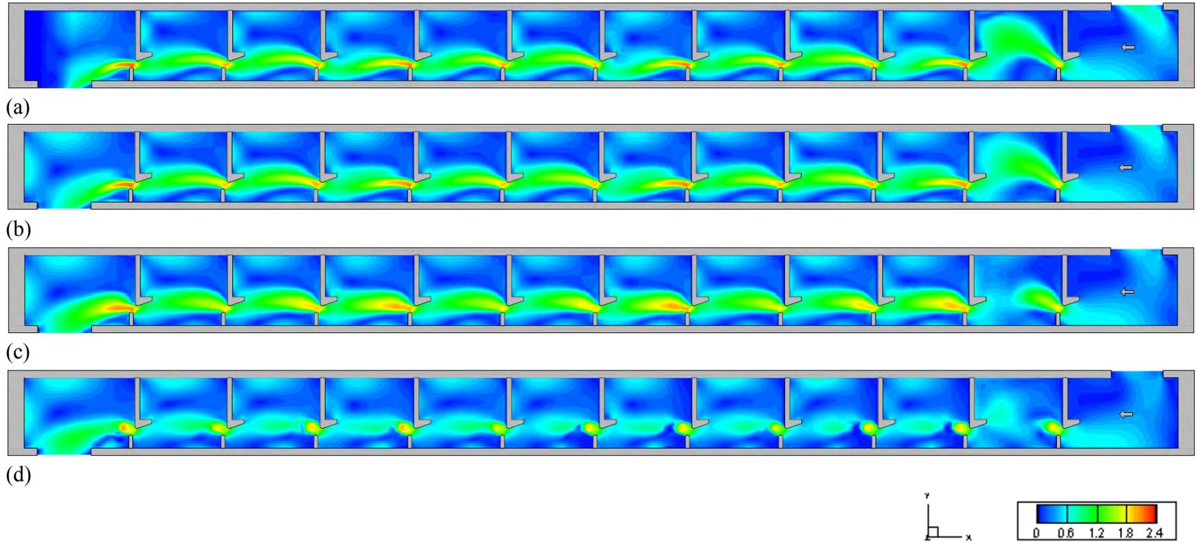
Figure 3.32 Velocity magnitude contours of Type III for the minimum flow case at flow depths of: (a)  $0.10h_u$ ; (b)  $0.25h_u$ ; (c)  $0.50h_u$ ; (d)  $0.75h_u$
