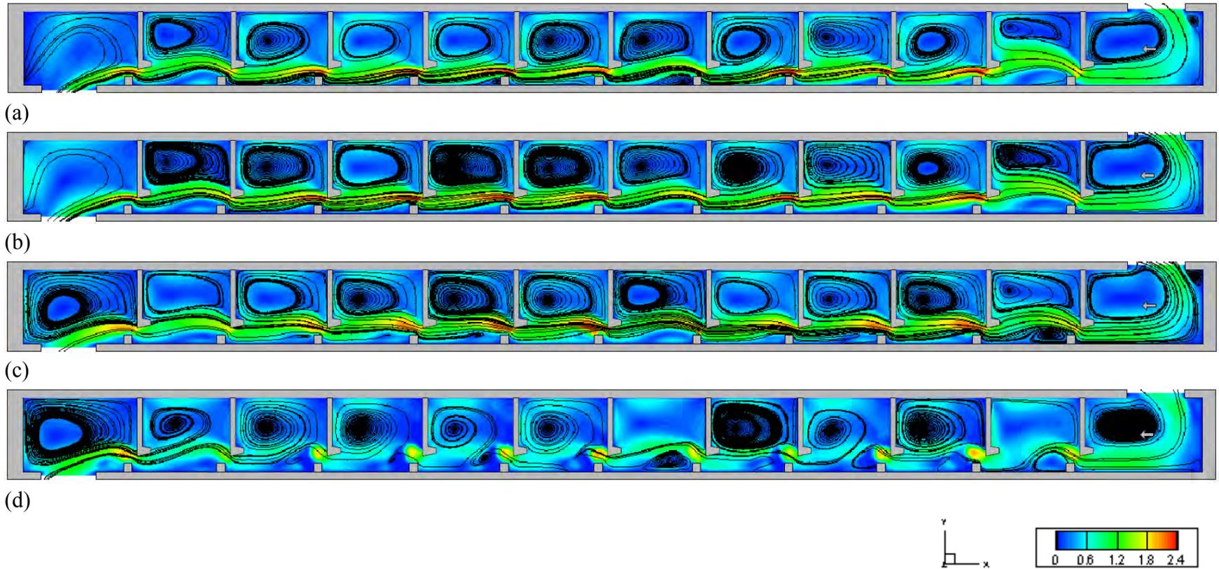
Figure 3.21 Velocity magnitude contours and streamlines of Type I for the minimum flow case at flow depths of: (a)  $0.10h_u$ ; (b)  $0.25h_u$ ; (c)  $0.50h_u$ ; (d)  $0.75h_u$
