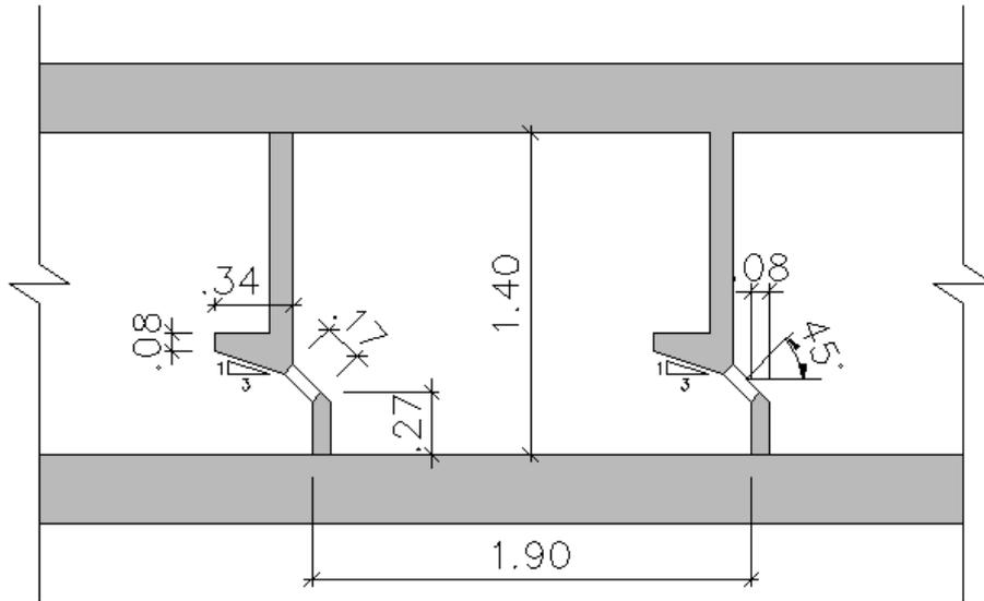
Figure 3.10 The dimensions of “Type II” in meter
