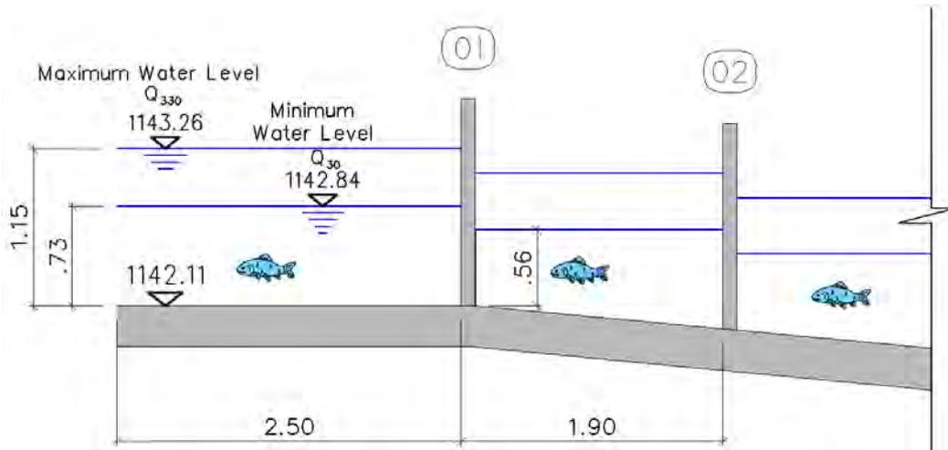
Figure 3.14 The sketch of the exit of the fish pass
