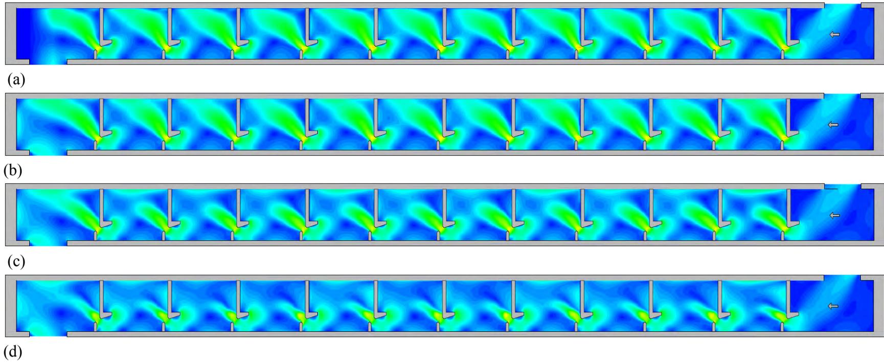
Figure 3.26 Velocity magnitude contours of Type II for the minimum flow case at flow depths of: (a)  $0.10h_u$ ; (b)  $0.25h_u$ ; (c)  $0.50h_u$ ; (d)  $0.75h_u$
