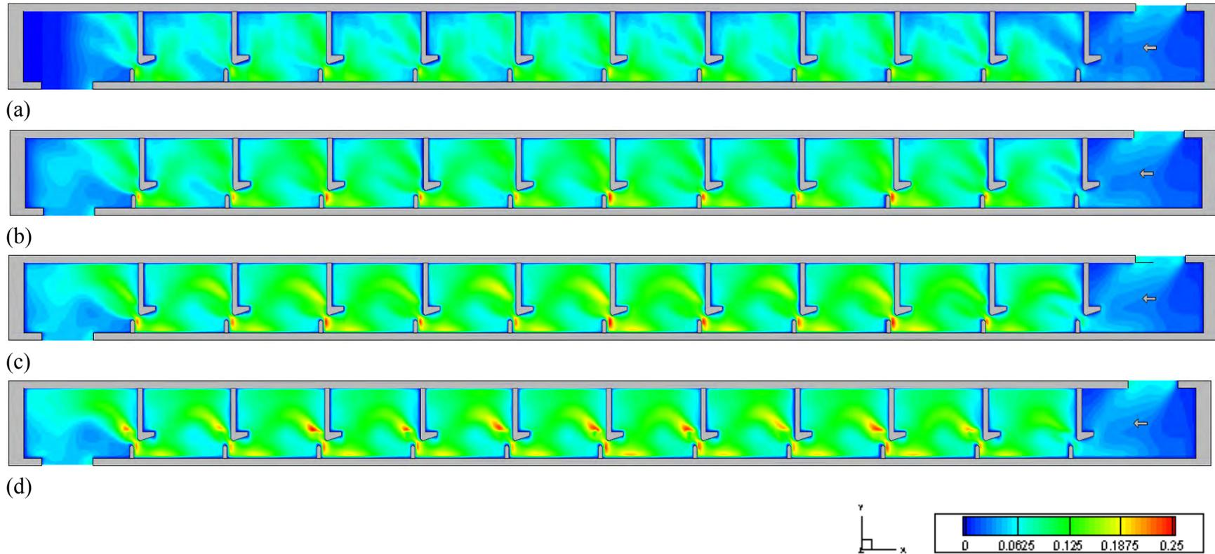
Figure 3.28 Turbulent kinetic energy contours of Type II for the minimum flow case at flow depths of: (a)  $0.10h_u$ ; (b)  $0.25h_u$ ; (c)  $0.50h_u$ ; (d)  $0.75h_u$
