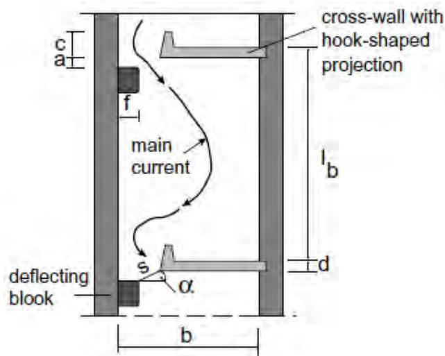
Figure 2.10 Dimensions and terminology for slot passes with one slot only (DWVK, 1996)
