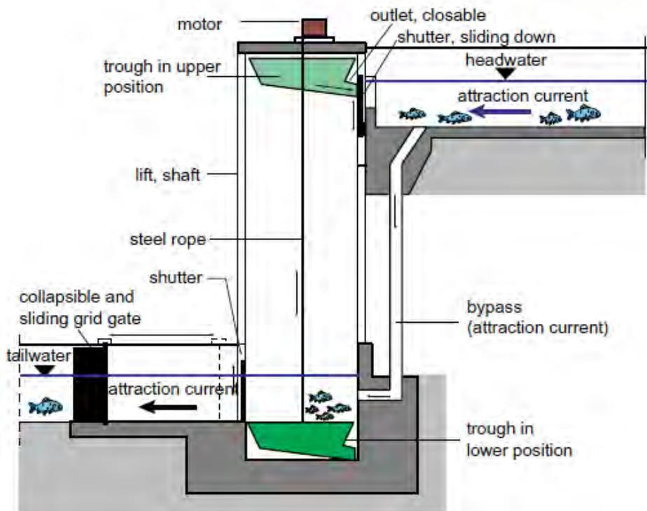
Figure 2.18 Schematic view of the structure of a fish lift (DVWK, 1996)
