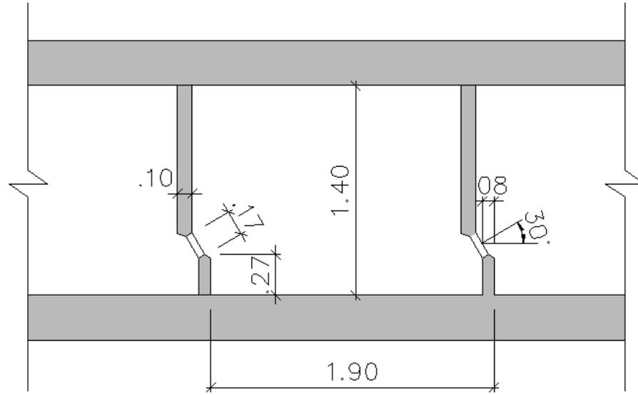
Figure 3.38 The dimensions of “Type IV” in meter
