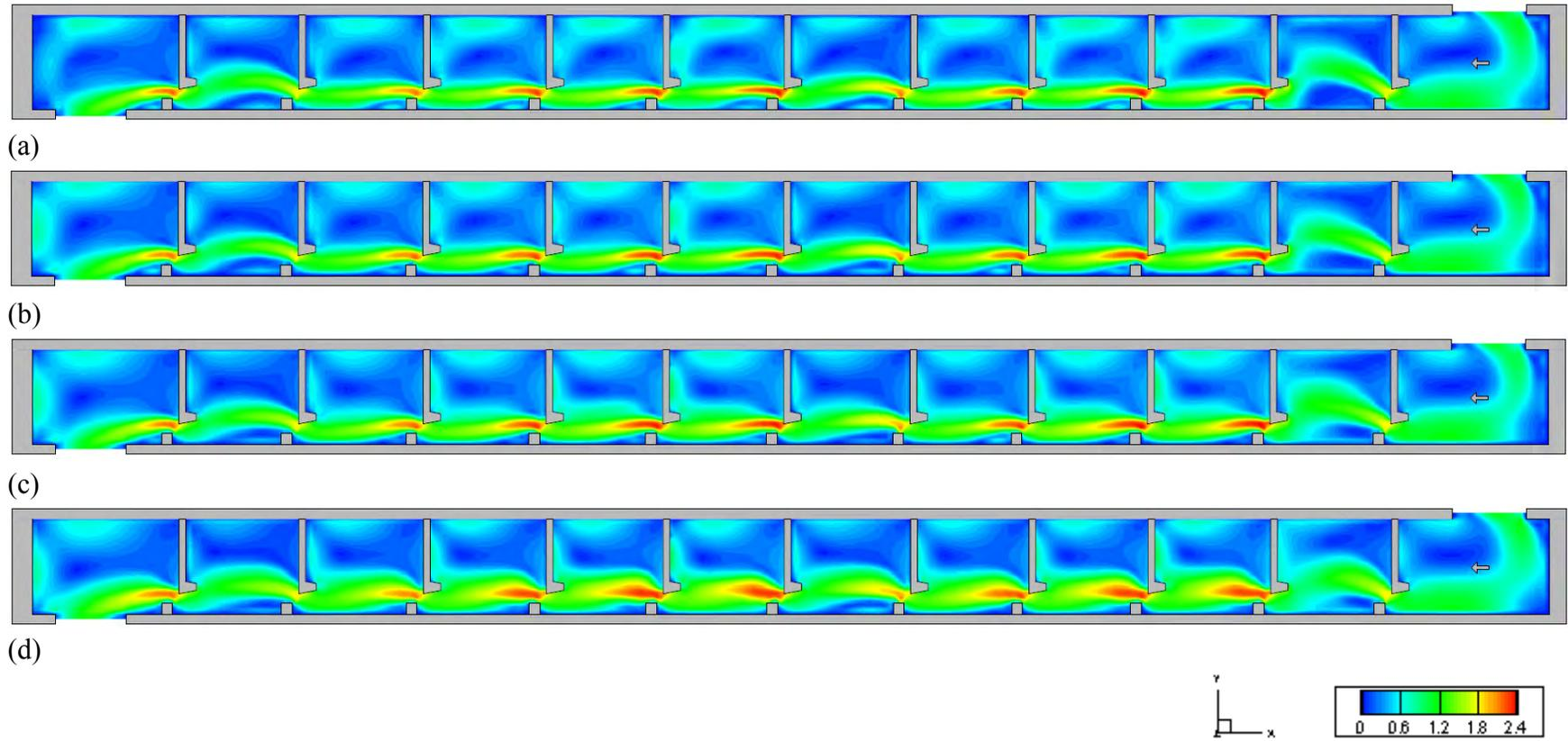
Figure 3.23 Velocity magnitude contours of Type I for the maximum flow case at flow depths of: (a)  $0.10h_u$ ; (b)  $0.25h_u$ ; (c)  $0.50h_u$ ; (d)  $0.75h_u$
