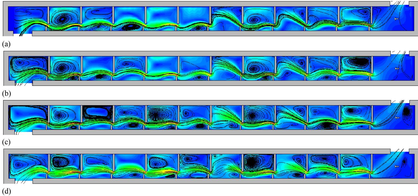
Figure 3.43 Velocity magnitude contours and streamlines of Type IV for the maximum flow case at flow depths of: (a)  $0.10h_u$ ; (b)  $0.25h_u$ ; (c)  $0.50h_u$ ; (d)  $0.75h_u$
