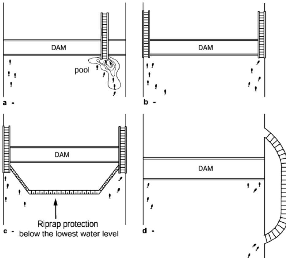
Figure 2.4 Schematic plans of different combination of fishway location (Larinier, 1992d)
