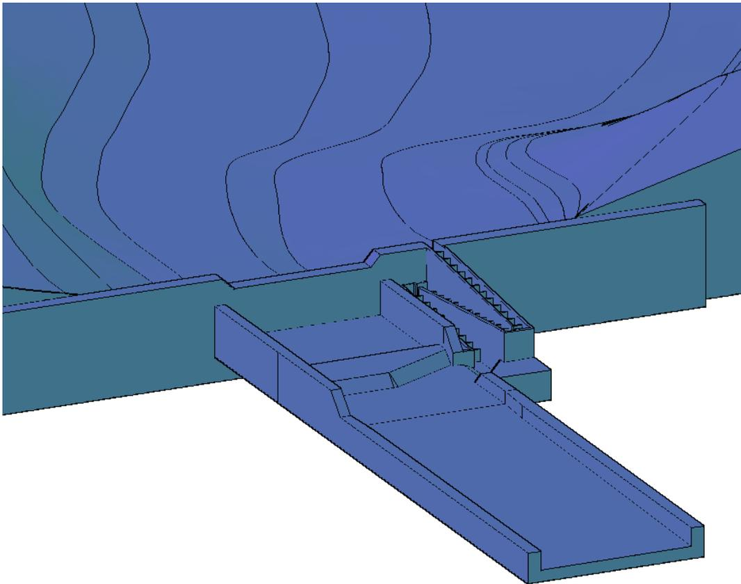
Figure 3.16 3D model of Uzungöl Weir-1
