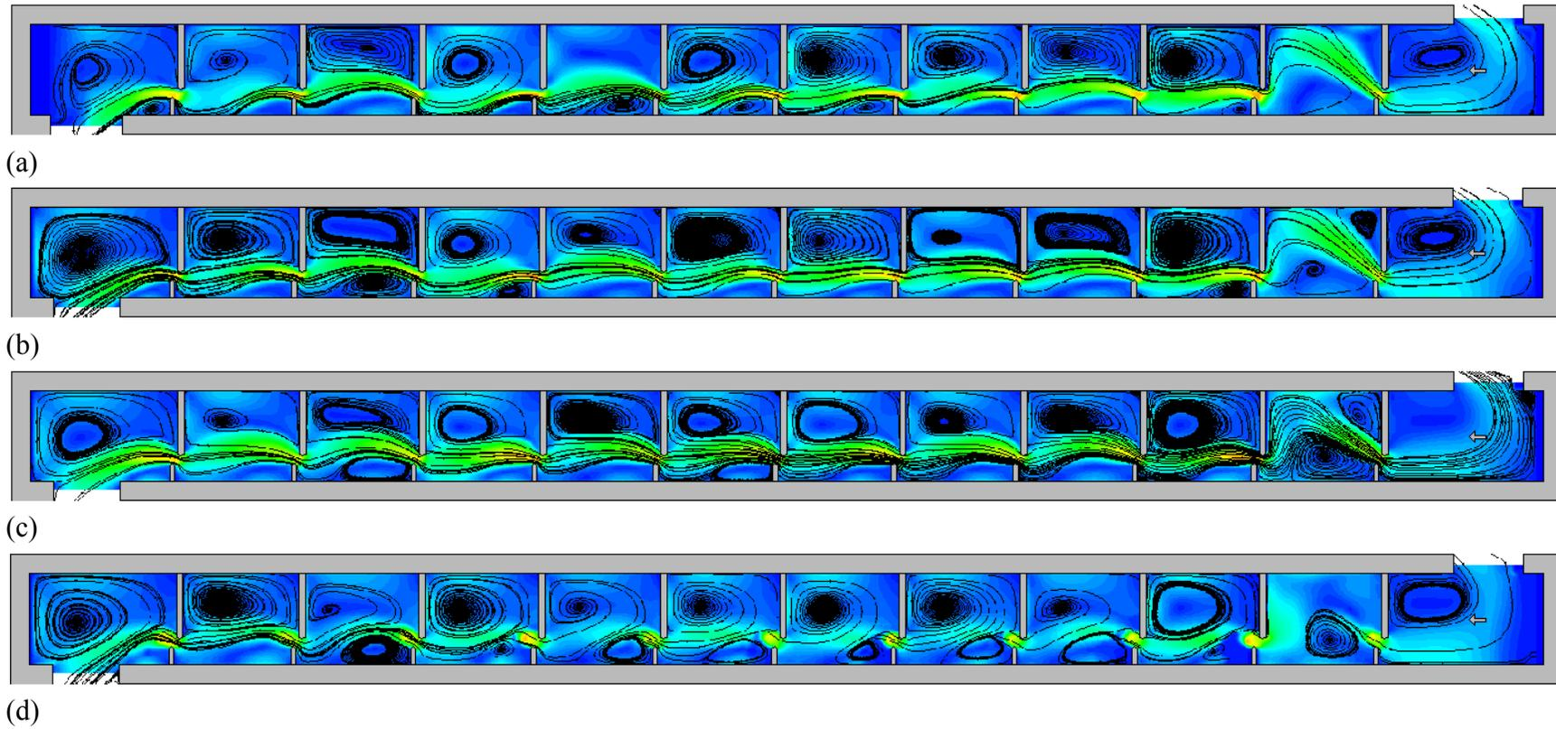
Figure 3.40 Velocity magnitude contours and streamlines of Type IV for the minimum flow case at flow depths of: (a)  $0.10h_u$ ; (b)  $0.25h_u$ ; (c)  $0.50h_u$ ; (d)  $0.75h_u$
