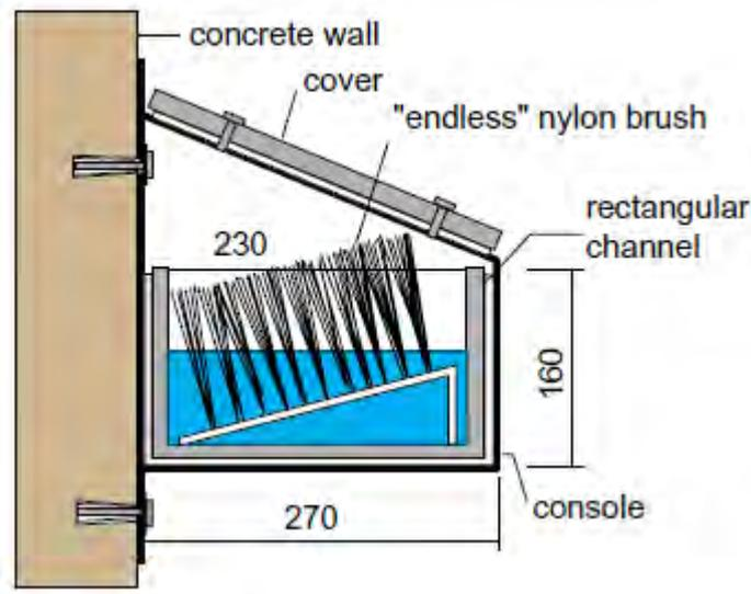
Figure 2.17 The eel ladder at the Zeltingen dam on the Moselle (Rhineland-Palatinate) (DVWK, 1996)
