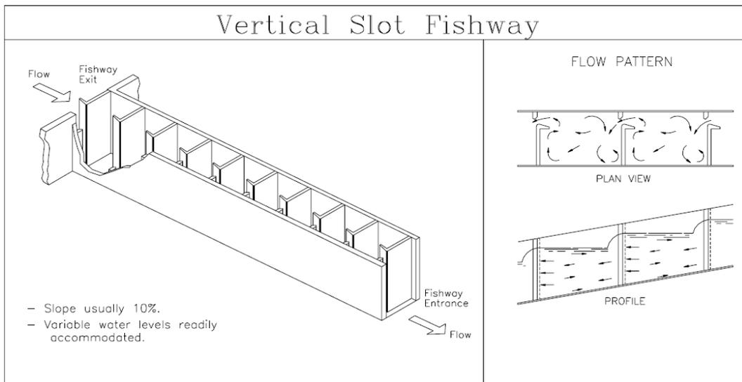
Figure 2.9 Vertical Slot Passes (Katopodis, 1992)
