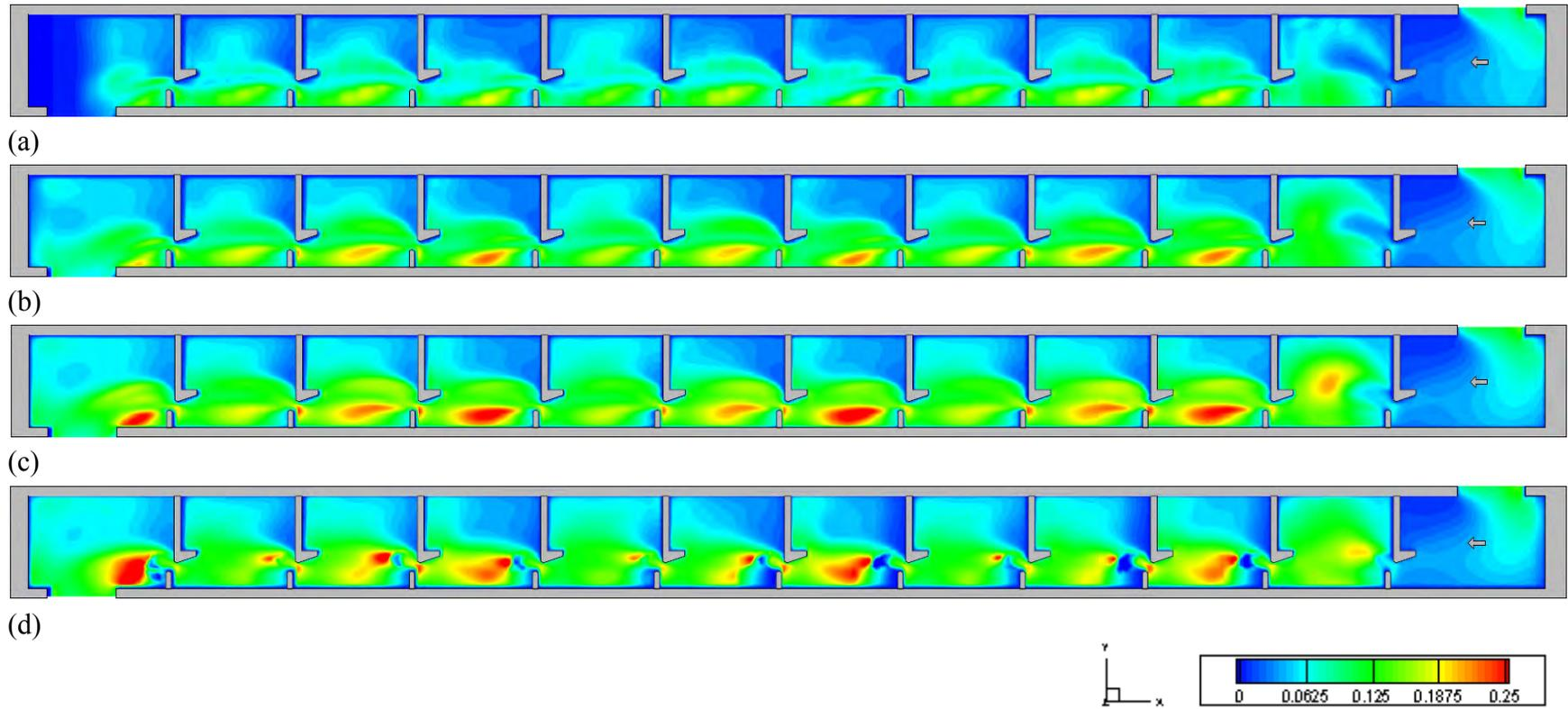
Figure 3.34 Turbulent kinetic energy contours of Type III for the minimum flow case at flow depths of: (a)  $0.10h_u$ ; (b)  $0.25h_u$ ; (c)  $0.50h_u$ ; (d)  $0.75h_u$
