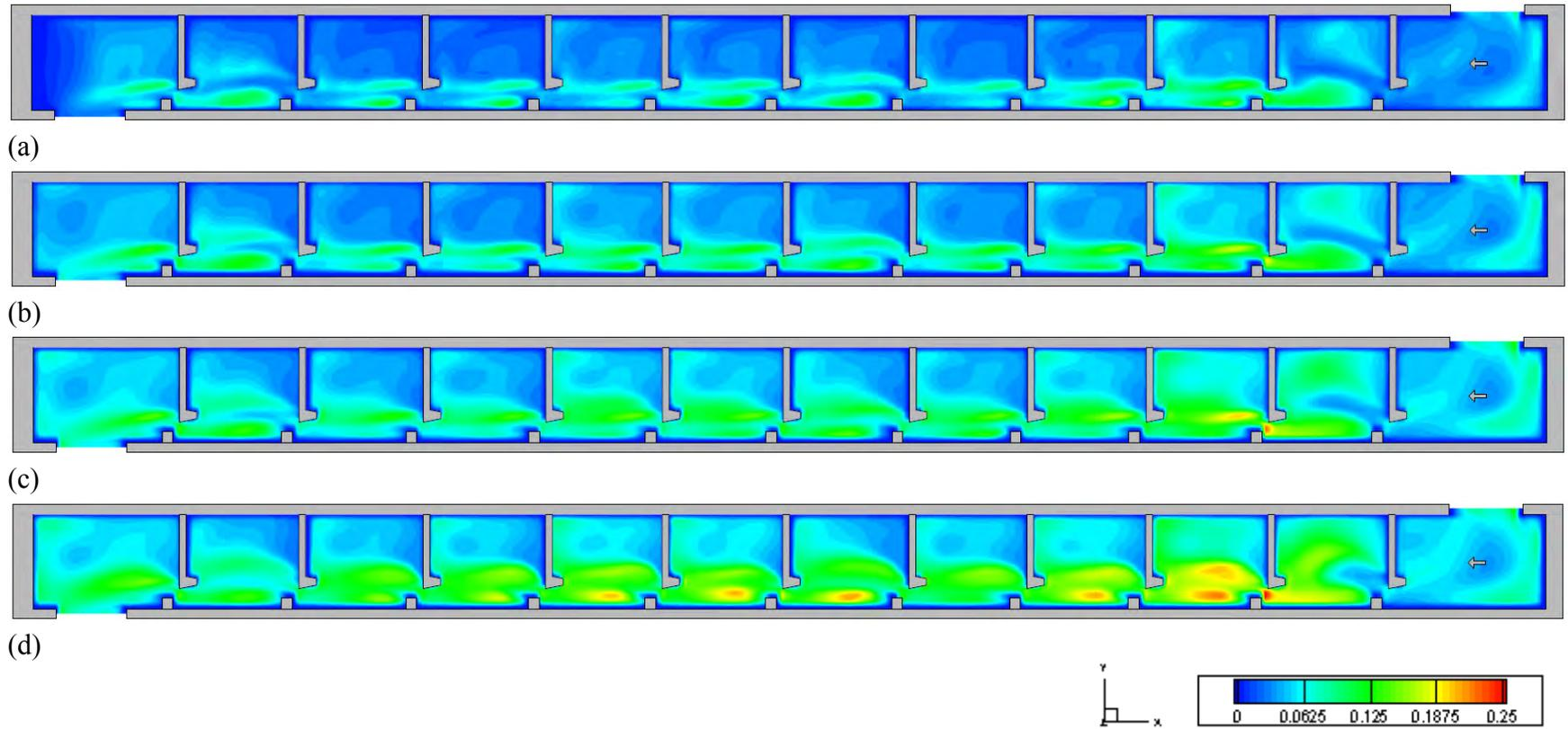
Figure 3.25 Turbulent kinetic energy contours of Type I for the maximum flow case at flow depths of: (a)  $0.10h_u$ ; (b)  $0.25h_u$ ; (c)  $0.50h_u$ ; (d)  $0.75h_u$
