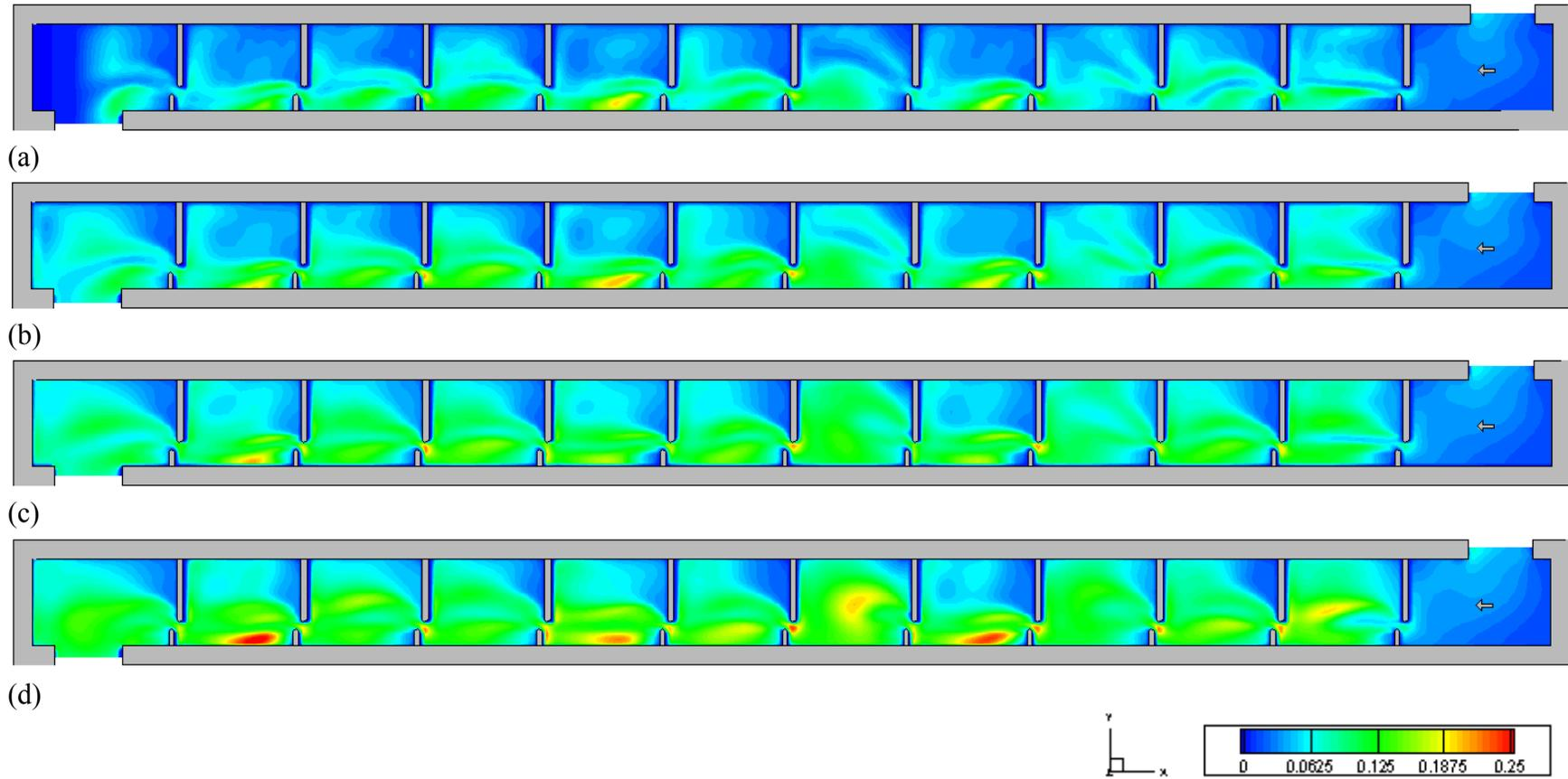
Figure 3.44 Turbulent kinetic energy contours of Type IV for the maximum flow case at flow depths of: (a)  $0.10h_u$ ; (b)  $0.25h_u$ ; (c)  $0.50h_u$ ; (d)  $0.75h_u$
