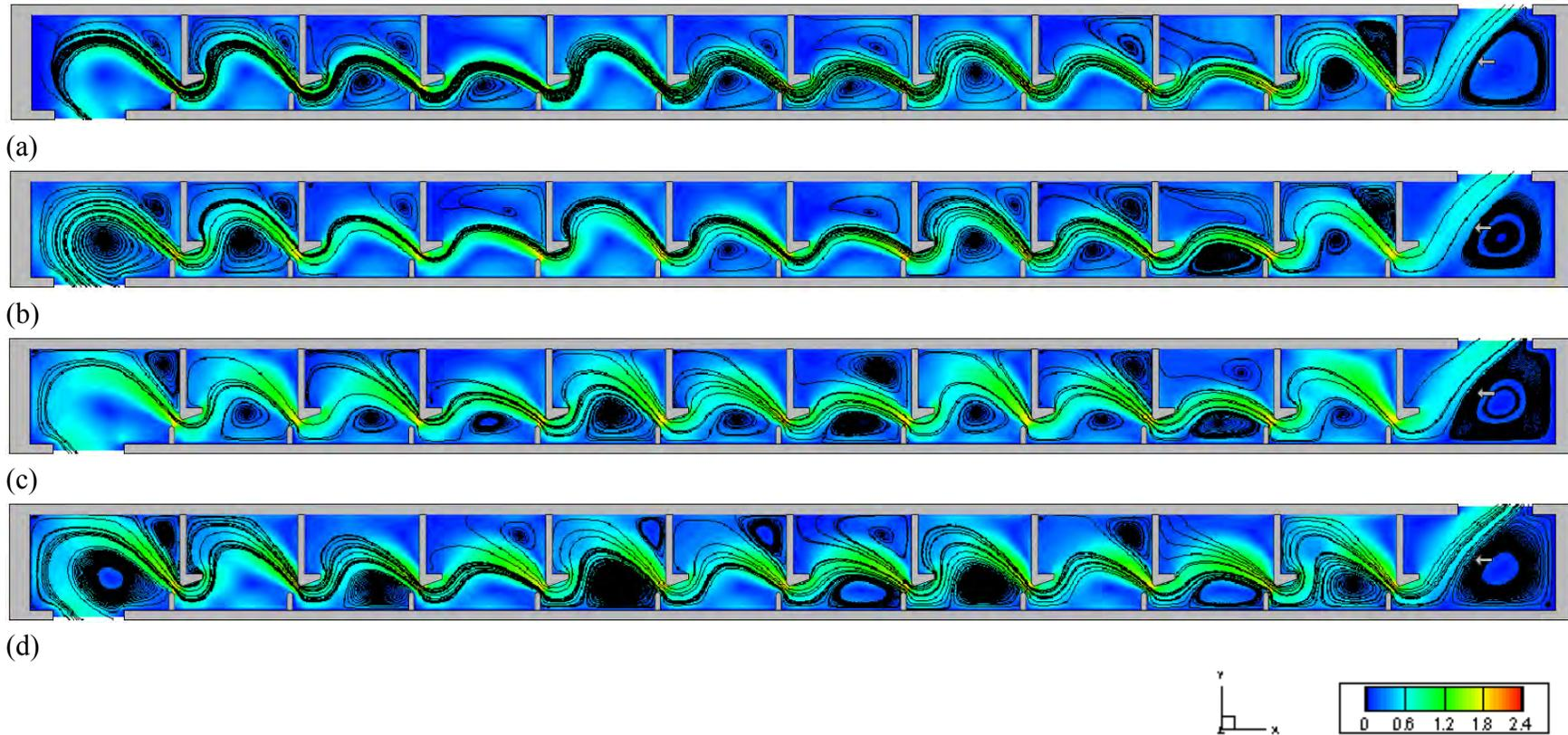
Figure 3.30 Velocity magnitude contours and streamlines of Type II for the maximum flow case at flow depths of: (a)  $0.10h_u$ ; (b)  $0.25h_u$ ; (c)  $0.50h_u$ ; (d)  $0.75h_u$
