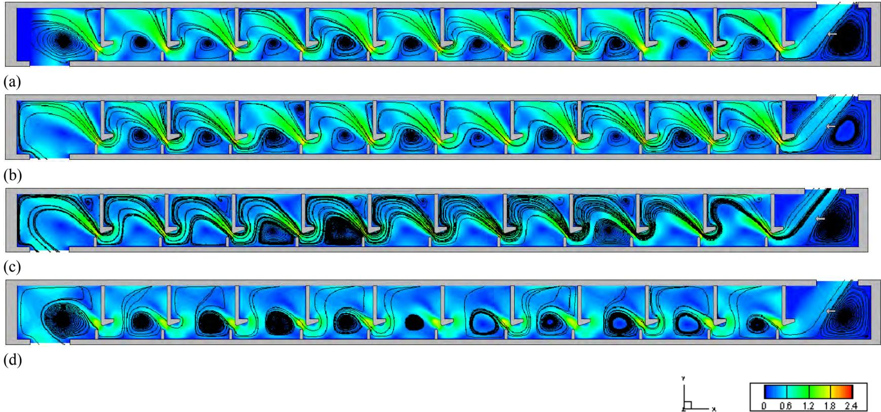
Figure 3.27 Velocity magnitude contours and streamlines of Type II for the minimum flow case at flow depths of: (a)  $0.10h_u$ ; (b)  $0.25h_u$ ; (c)  $0.50h_u$ ; (d)  $0.75h_u$
