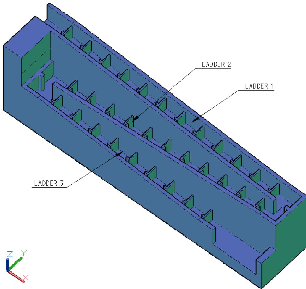
Figure 3.17 3D model of the fish pass
