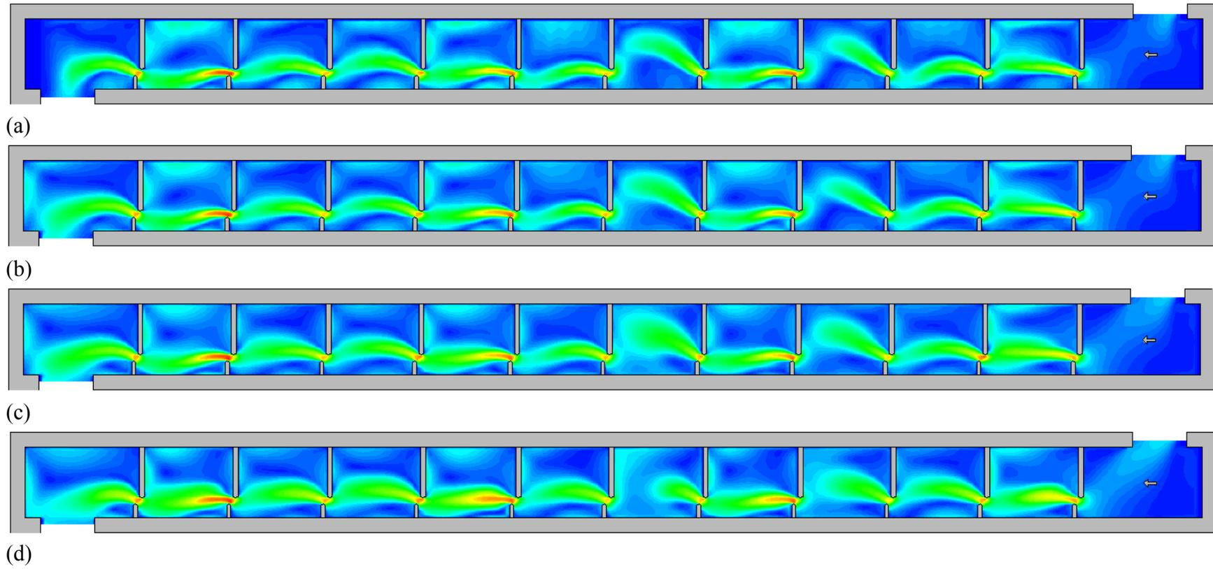
Figure 3.42 Velocity magnitude contours of Type IV for the maximum flow case at flow depths of: (a)  $0.10h_u$ ; (b)  $0.25h_u$ ; (c)  $0.50h_u$ ; (d)  $0.75h_u$
