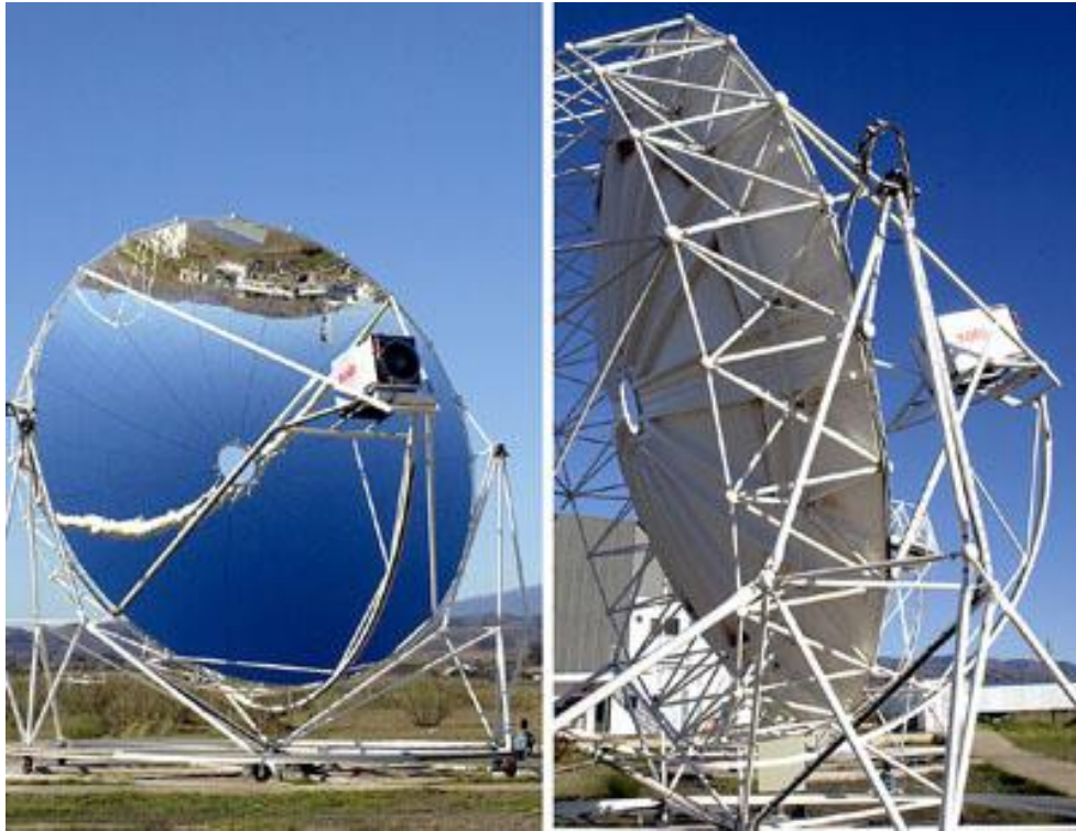
Figure 1.3 Front and Back Views of EUROdishes, (Plataforma Solar de Almería, 2014)
