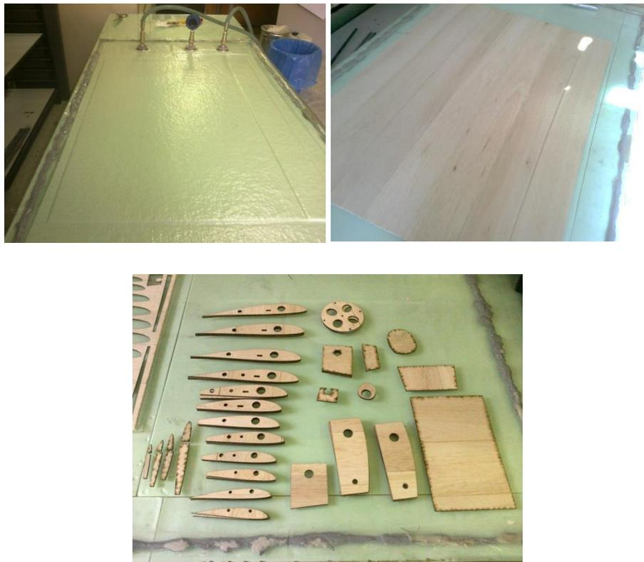
*Figure 4.14 Manufacturing of the Inner Structural Frames*
