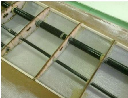
*Figure 4.18 Preparing the Upper Wing Surface*
