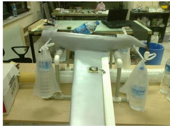
*Figure E.0.6 Static Loading of Motor Booms*
