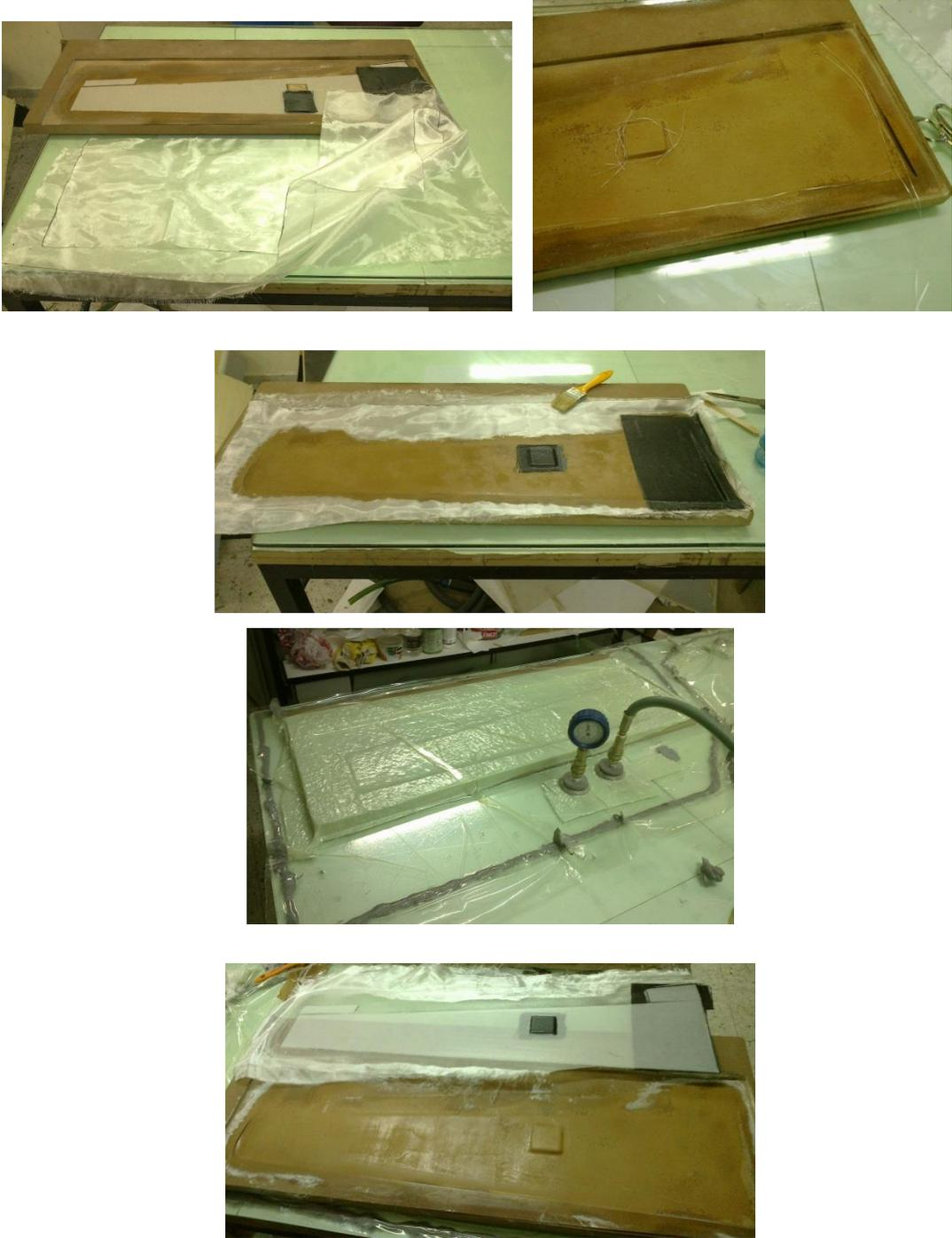
*Figure 4.12 Manufacturing of the Wing Skins*
