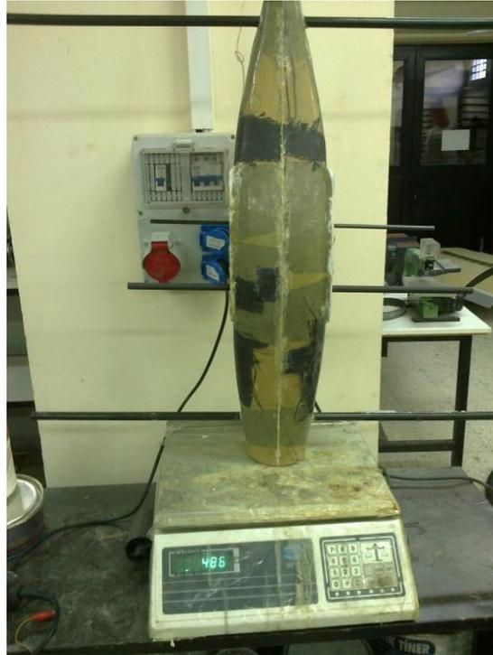
*Figure 4.16 Assembled Fuselage*
