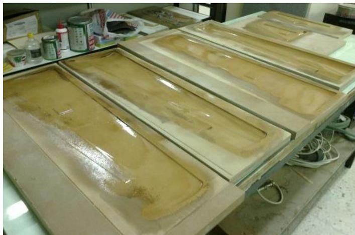
*Figure 4.9 Scenes from Surface Finishing Treatments (Polyester putty on fuselage mold, applying primer on wing molds and varnished molds)*
