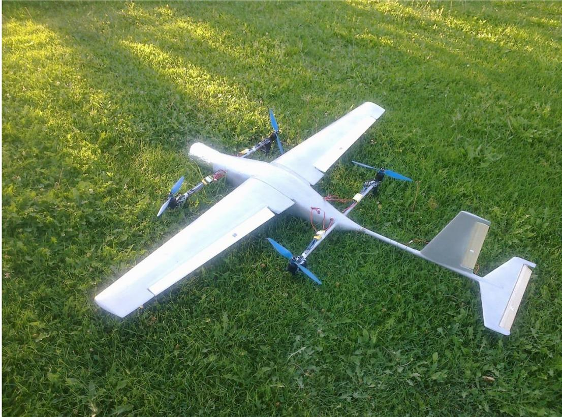
*Figure 4.28 View of the Equipped Aircraft (Fixed Wing Mode) for R/C Flight*
