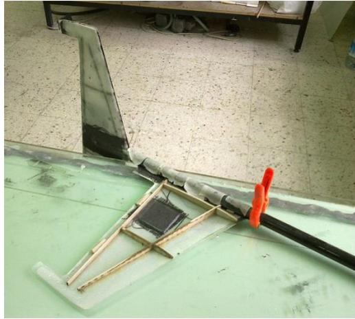
*Figure 4.22 Positioning and Adhering the Vertical Tail*
