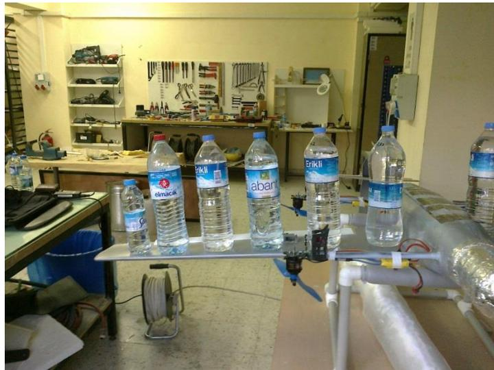
*Figure E.0.5 Wing Deformation in 1g Static Wing Loading Test*
