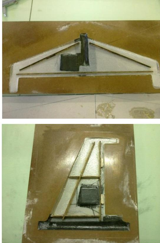
*Figure 4.20 Inner Structure of the Tail Surfaces*
