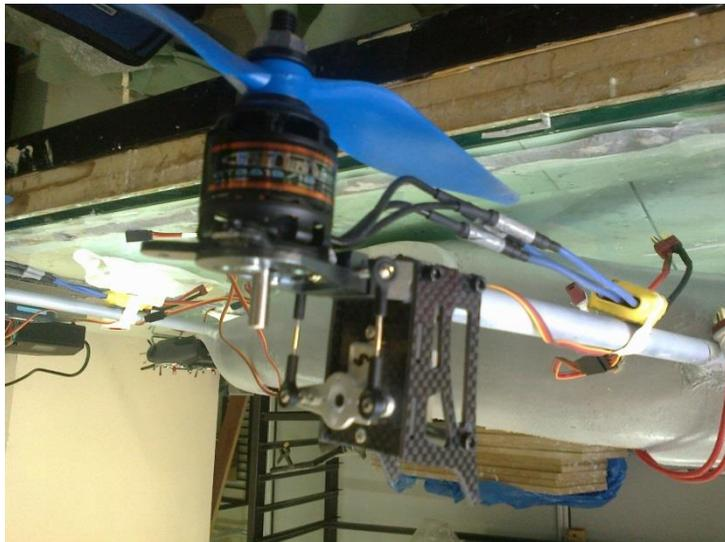
*Figure 4.27 Tilt Mechanism Installed on the Aircraft*
