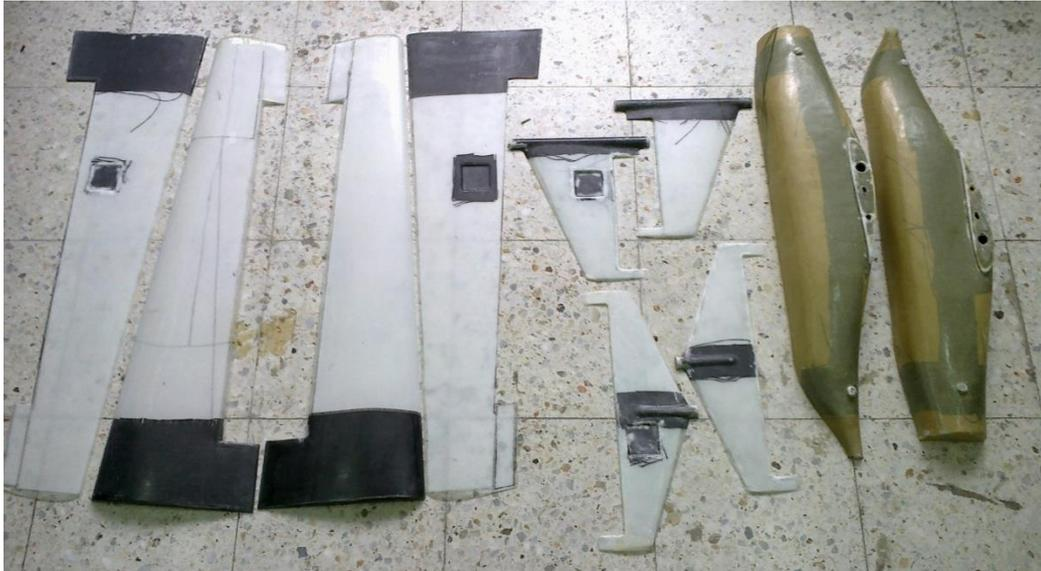
*Figure 4.13 All of the Composite Skins Parts of the Aircraft*
