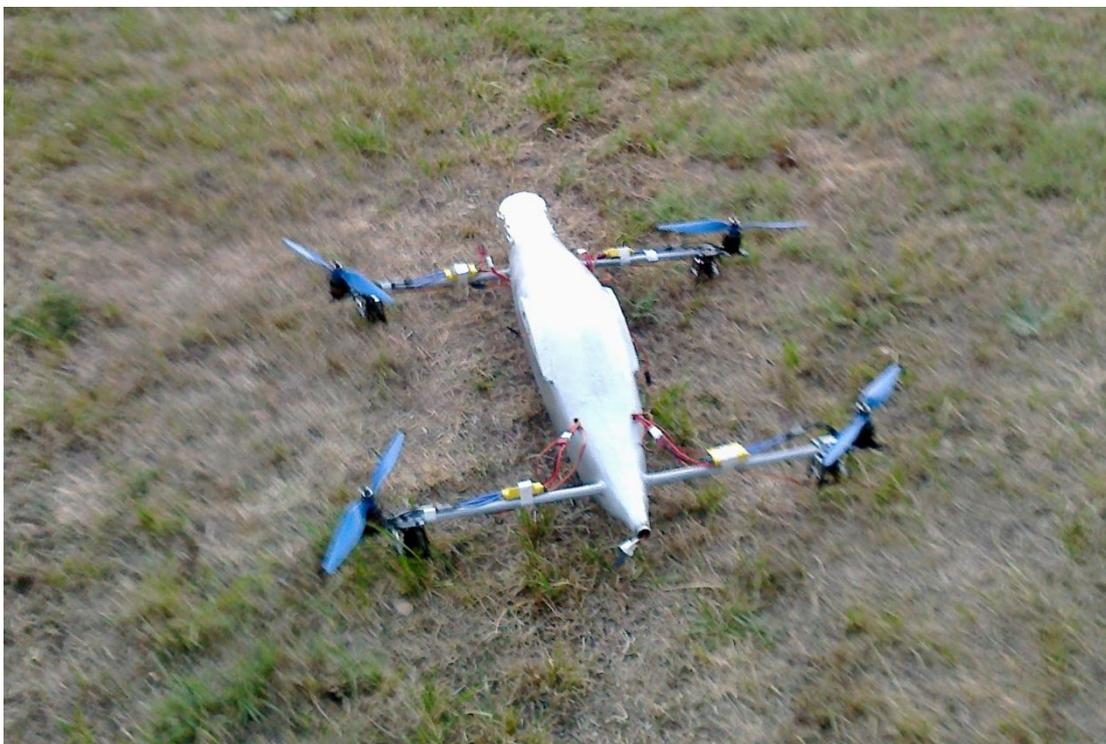
*Figure 4.29 View of the Equipped Aircraft (in Quad-rotor mode) for R/C Flight*
