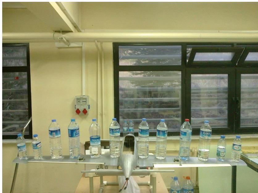
*Figure E.0.1 1g Static Wing Loading Test (about 2.5kg at each wing)*
