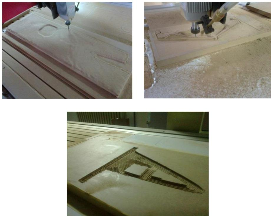
*Figure 4.8 Scenes from Machining of the Molds (Finishing of the wing and horizontal tail; roughening of the vertical tail)*
