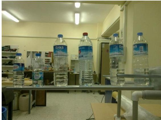
Figure E. 0.3 Wing Deformation in 1g Static Wing Loading Test
