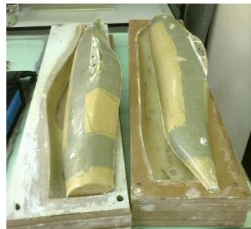
Figure 4.11 Manufacturing of the Fuselage Skins
