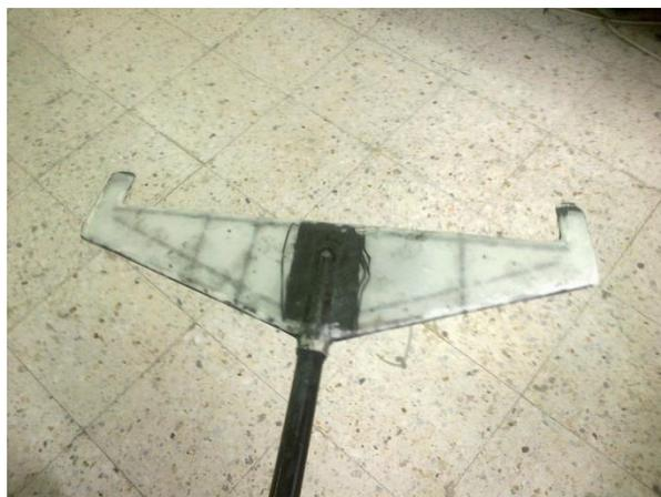
*Figure 4.21 Horizontal Tail Adhered to the End of the Tail Boom*
