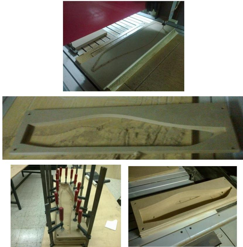
*Figure 4.7 Machining the Fuselage Mold*
