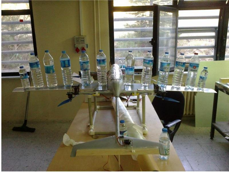
*Figure E.0.4 3g Static Wing Loading Test (about 7.5 kg at each wing)*
