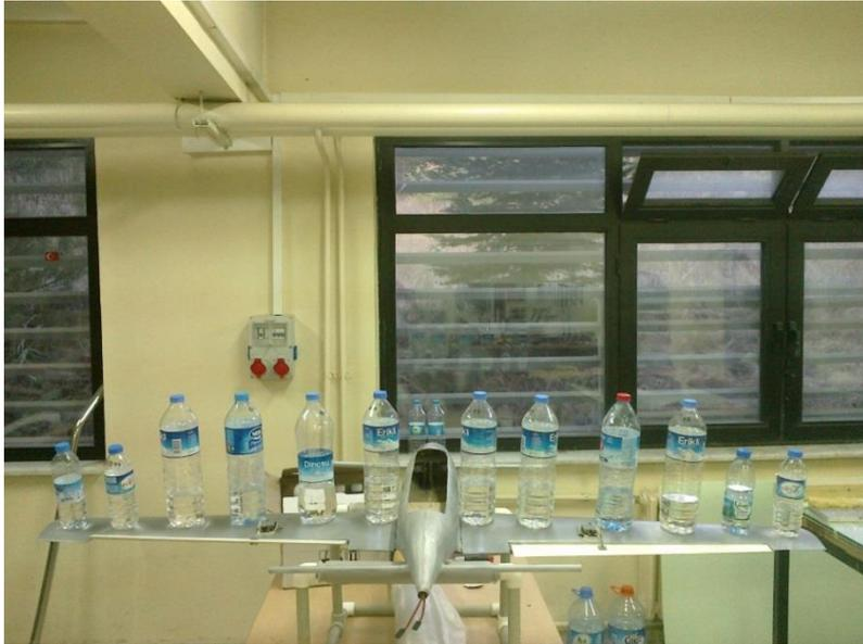
Figure E. 0.2 1g Static Wing Loading Test (about 2.5kg at each wing)
