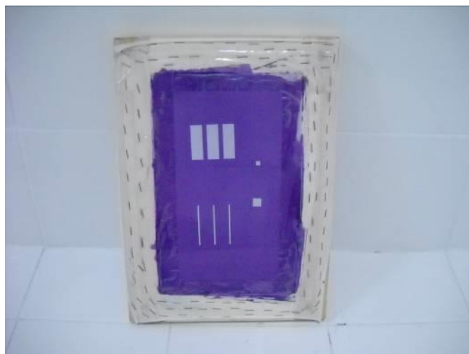
Figure 3.3 aluminium screen used during screen printing deposition [5].
