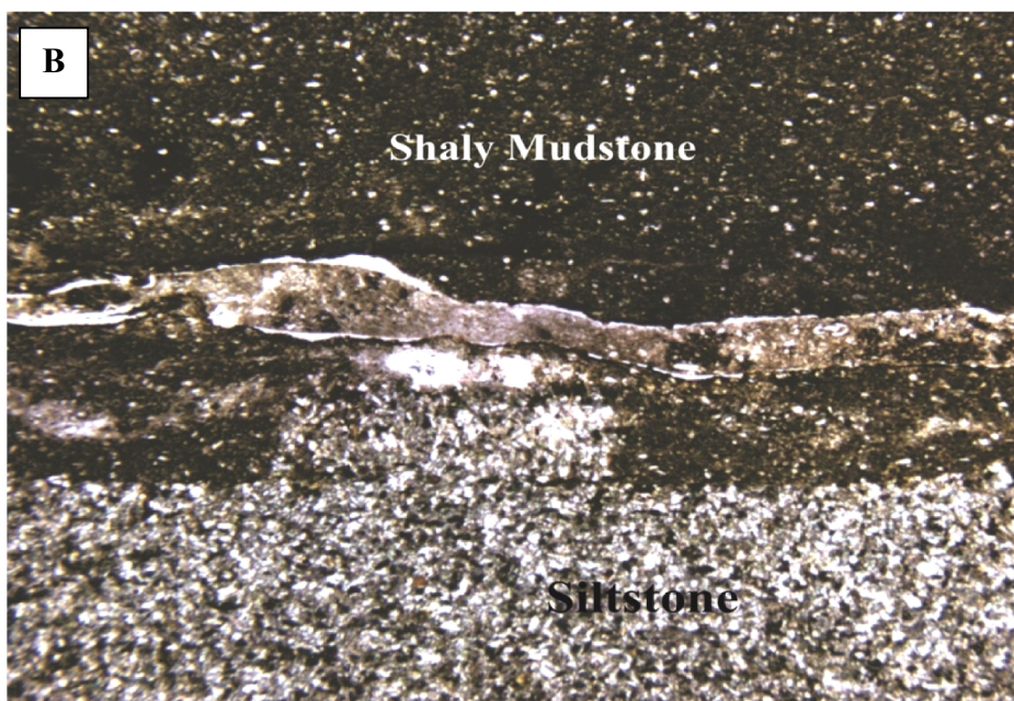
Figure 3.23: Photomicrographs of greenish to gray siltstone representing laminated siltstone and representing contact with greenish gray to gray Mudstone (Sample no. GOZ41, (A) PPL x2.5, GOZ45, (B) PPL x2.5).
