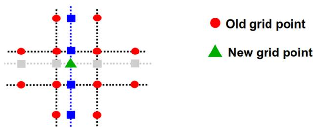
**Figure 2.5:** Interpolation Scheme for Quasi-Regular Gaussian Grids (Dando, 2013)
