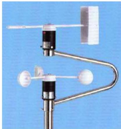
**Figure 3.4:** A Typical Bucket Anemometer ([www.dmi.gov.tr](http://www.dmi.gov.tr))
