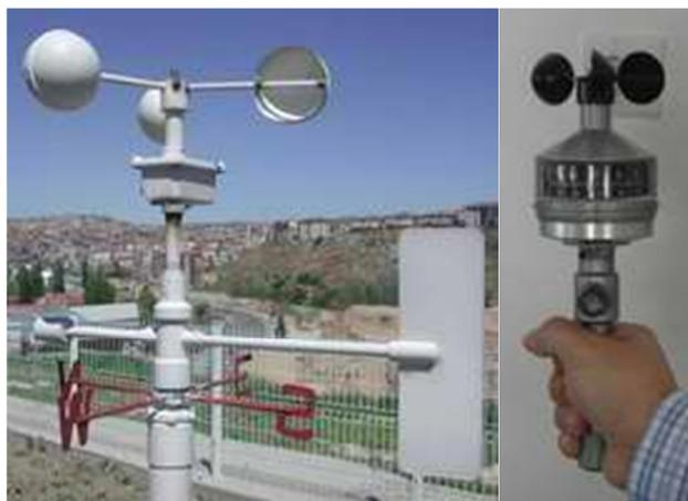
**Figure 3.1:** Examples of Fixed Anemometer (right) and Manual Anemometer (left)
