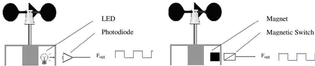
**Figure 3.5:** General Schematic View of Wind Speed Measurement System
