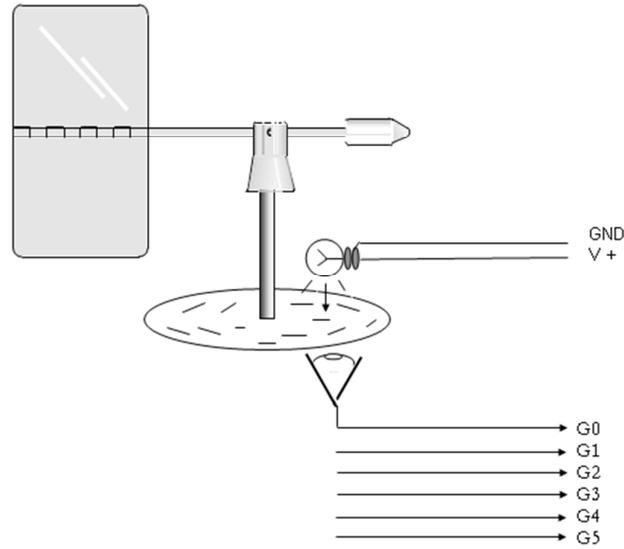
**Figure 3.6:** A Typical Schematic View of Wind Direction Apparatus
