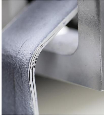
Figure 4.3.3 Picture of the [0] UD specimen after failure.
