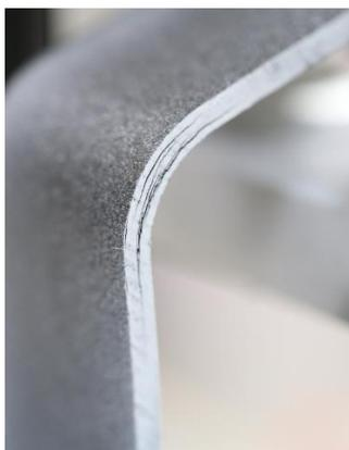
Figure 4.2.2 The cracked surface of F2 after failure.
