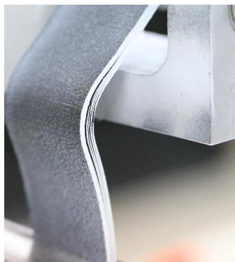
Figure 4.4.3 Picture of the [90/0] cross-ply specimen taken after the failure.
