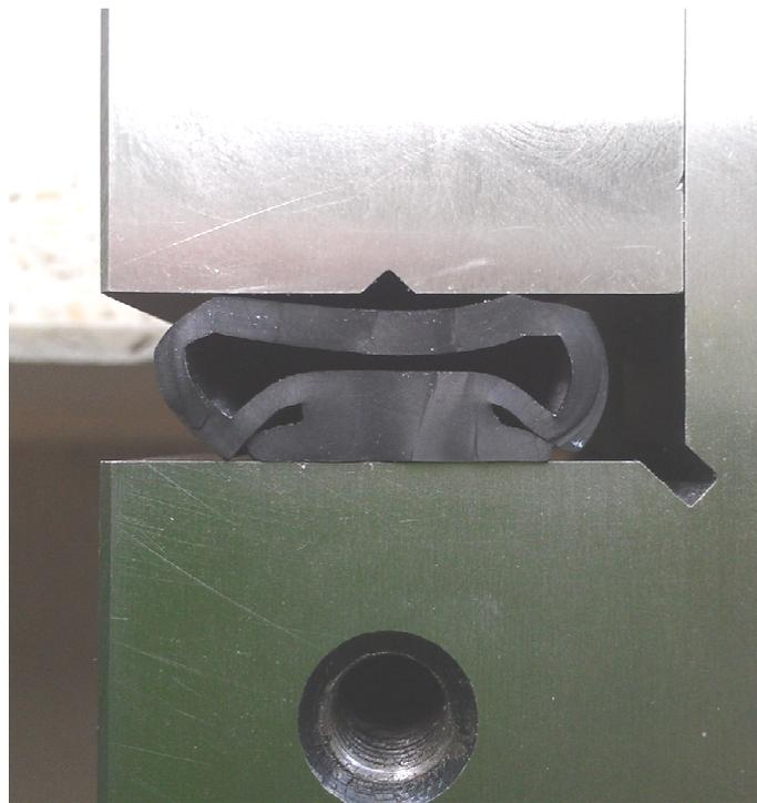
**Figure 29. Buckling occurs when the system is under compression**
