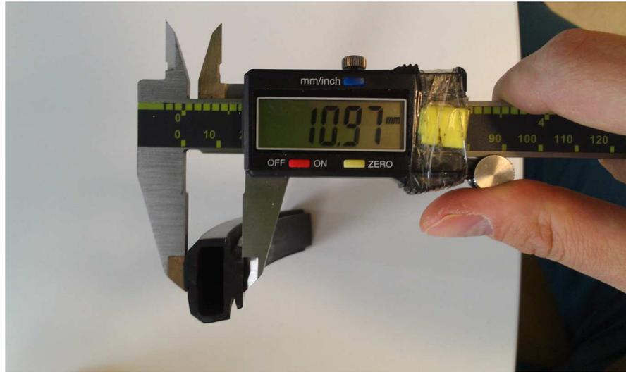
**Figure 28. BilPlas sample and its thickness**
