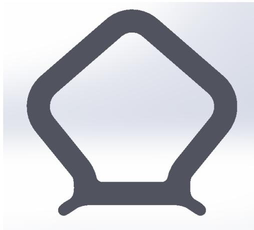
**Figure 15. Section of seal obtained from Standart Profil Co.**
