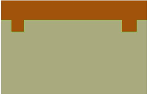
3. Pour, Degas, and Cure the PDMS Mold on to the Master Silicon Wafer
