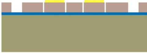
3. SOI Active Layer Structure Etch by DRIE with Bioactivation Metals Appear on Proof Masses of the Resonators
