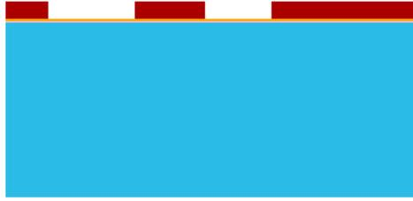
3. Metal Mask Coat and Lithography for Recess Etch on Glass
