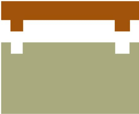
4. After Curing Peel Off PDMS Mold as a Whole Wafer
