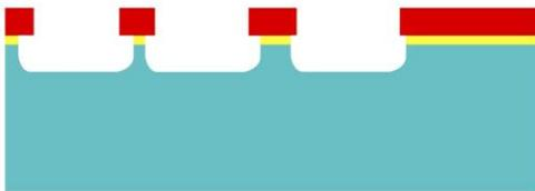
5. Recess Gap Etch on Glass with Metal Mask Under Pure HF
