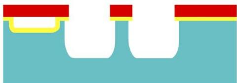
6. Microchannel Etch Inside the Glass with Metal Mask Under Pure HF
