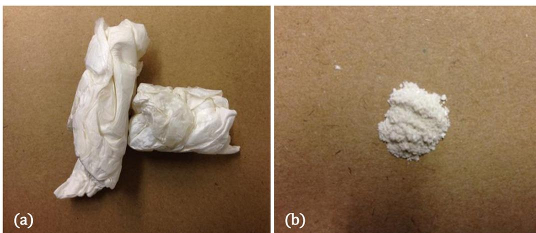
Figure 12. Dried BC (a) before and (b) after sulfuric acid treatment.
