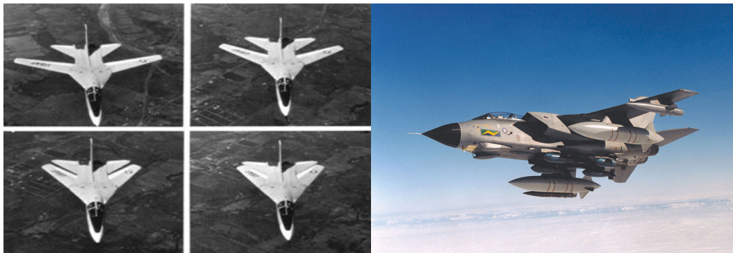
Figure 1.5 F-111 at different sweep phases (left) [8], Tornado F3 (right) [7].
