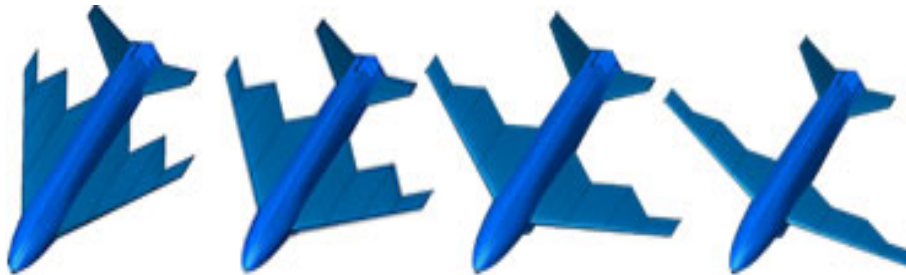
Figure 1.7 Hypercomp/NextGen's morphing wing on UAV [10].
