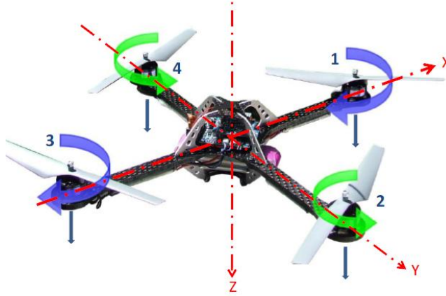
Figure 1.6: Body coordinate system of the quadrotor [18]
