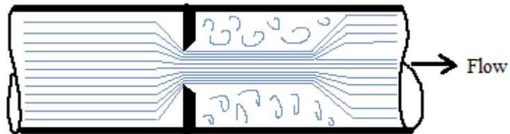
**Figure 4-28.** Flow through orifice
