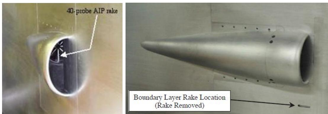
Figure 3-2 Photograph of Inlet Model Mounted on Tunnel Sidewall. [8]
