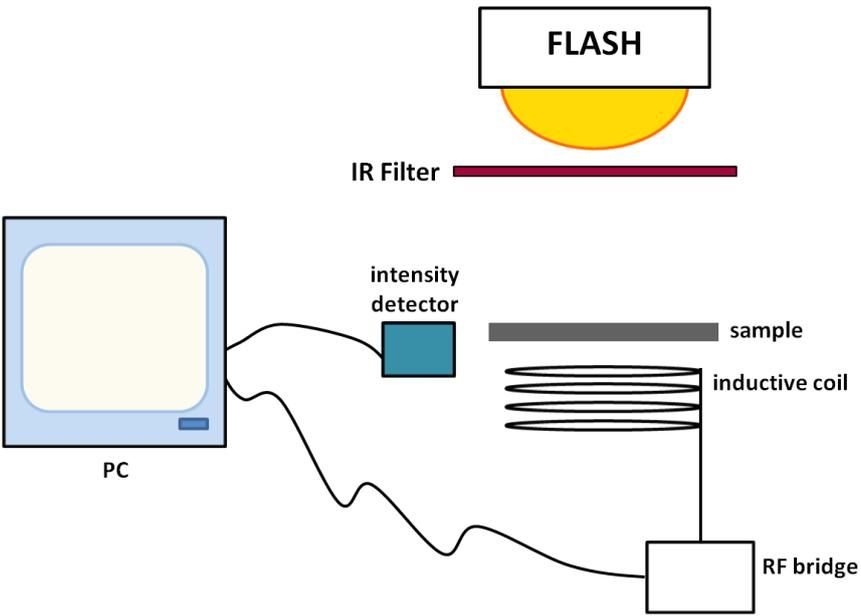
**Figure 51: Schematic of Lifetime measurement system**
