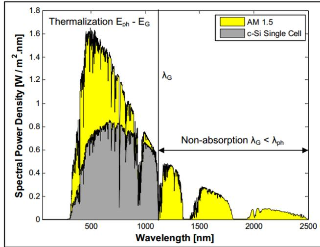
Figure 15: Fraction of AM1.5 spectrum utilized by c-Si [16]
