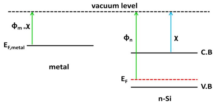
**Figure 26: Band Diagram of metal and n-Semiconductor before physical contact**
