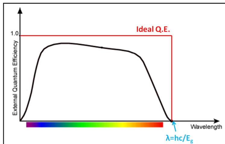
**Figure 11: External quantum efficiency of a silicon solar cell [13]**
