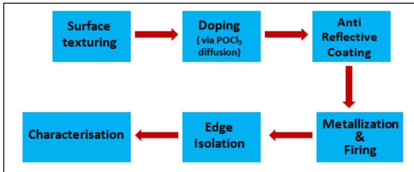
**Figure 14: Standard solar cell production**
