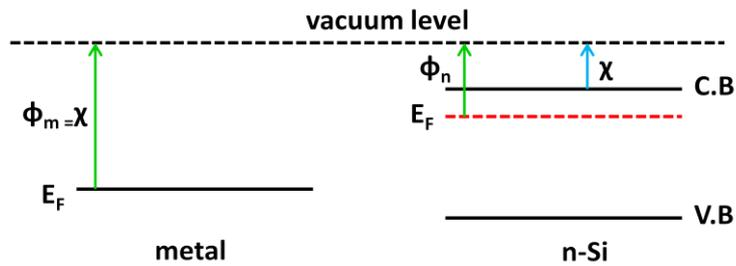
**Figure 24: Band diagrams of metal and n-Semiconductor before physical contact**
