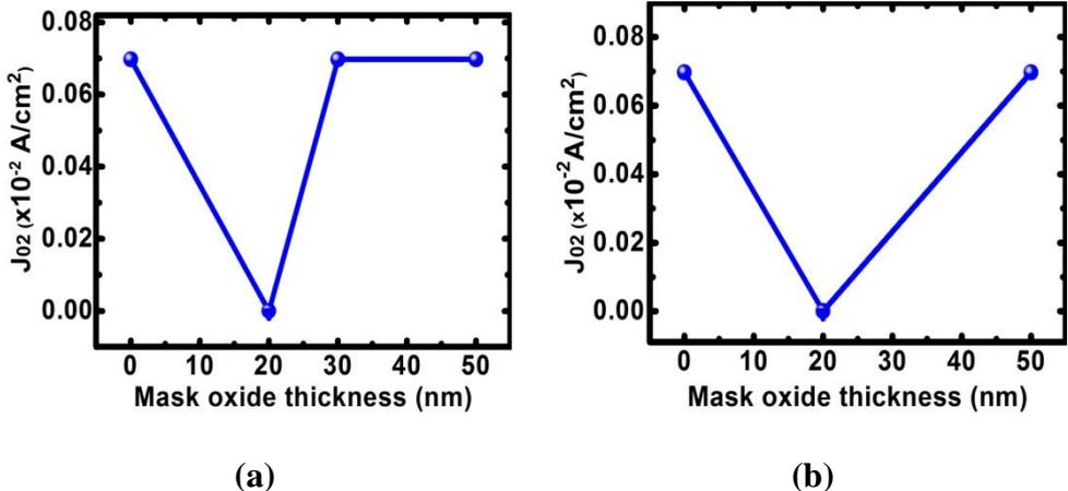
Figure 82: Effect on mask oxide thickness on J<sub>02</sub> (a) with (b) without oxide passivation. Lines are for visual aid
