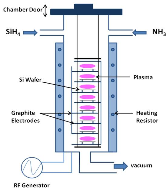
**Figure 46: Schematic of PECVD chamber**
