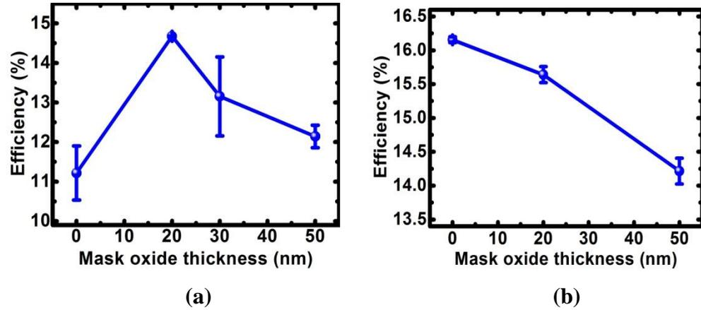
**Figure 70: Effect of mask oxide thickness on cell efficiency of fabricated cells (a) with oxide passivation, (b) without oxide passivation. Lines are for visual aid**
