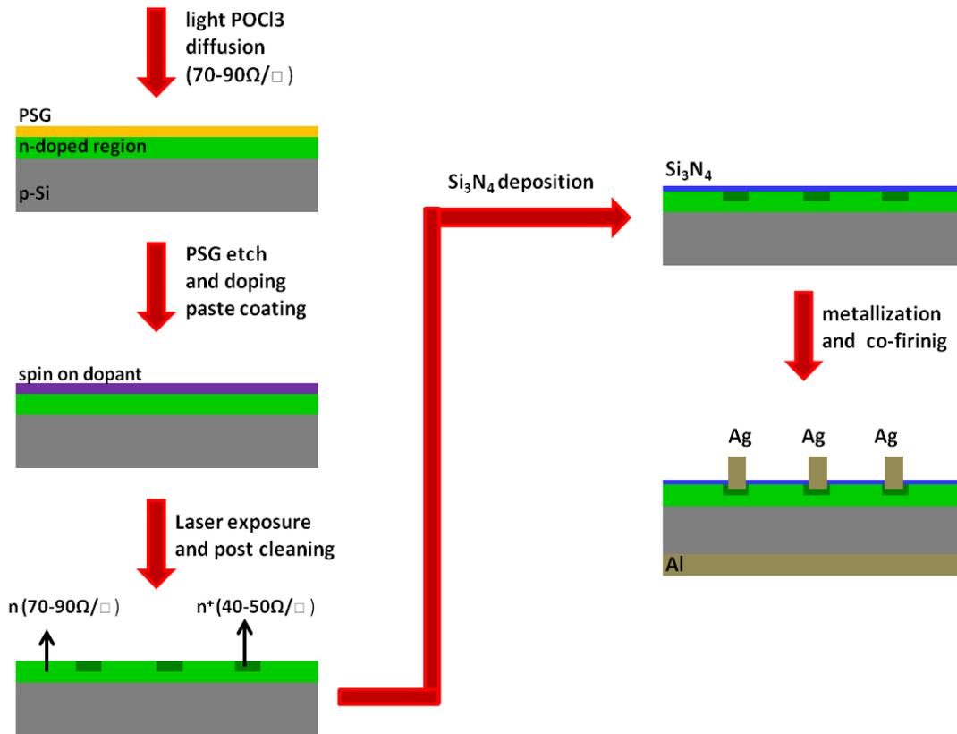
**Figure 33: Fabrication process of laser doped selective emitter solar cells with two step doping**
