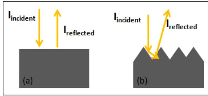
**Figure 18: Reflection from a flat surface (a) and textured surface (b)**
