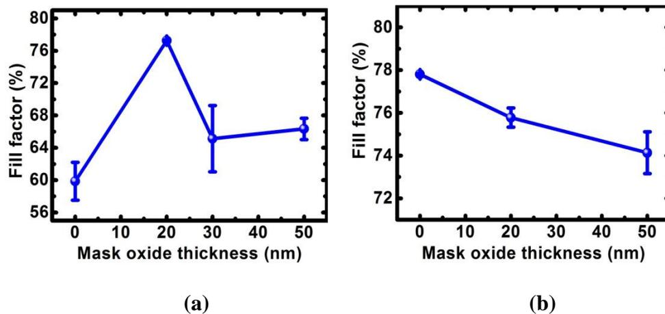
**Figure 71: Effect of mask oxide thickness on fill factor of solar cells (a) with oxide passivation, (b) without oxide passivation. Lines are for visual aid**
