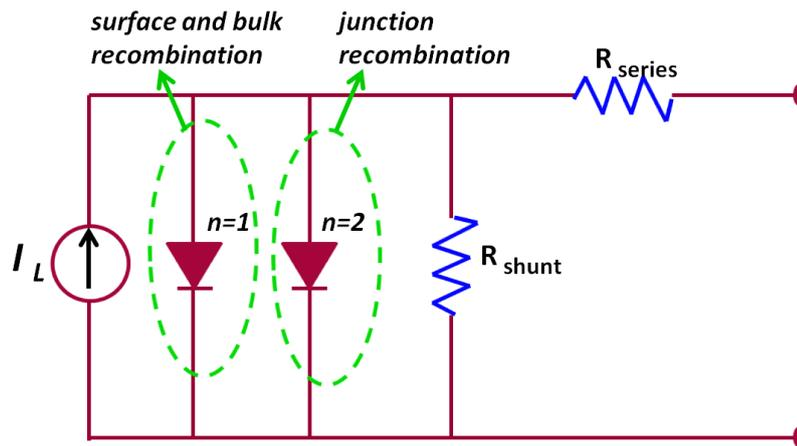
**Figure 61: Circuit representation of two diode model**
