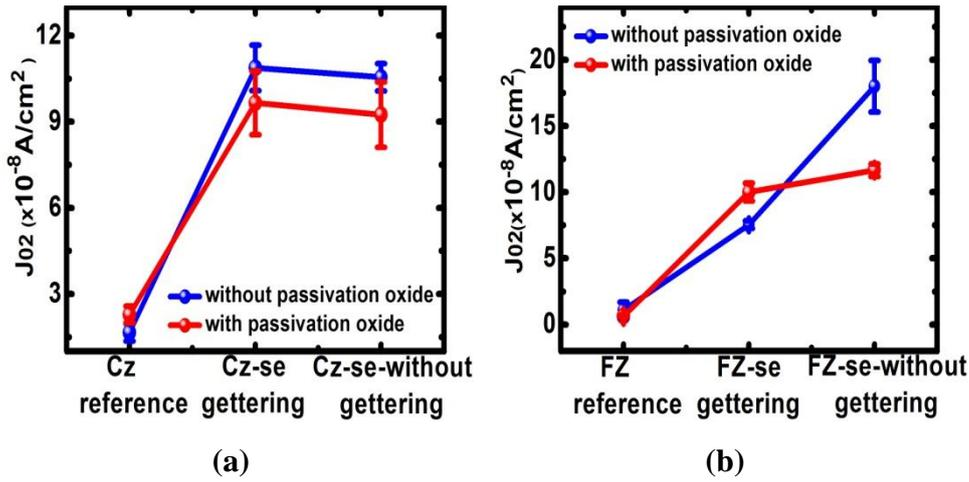
**Figure 96: Measured  $J_{02}$  values of fabricated (a) Cz and (b) FZ cells. Lines are for visual aid**
