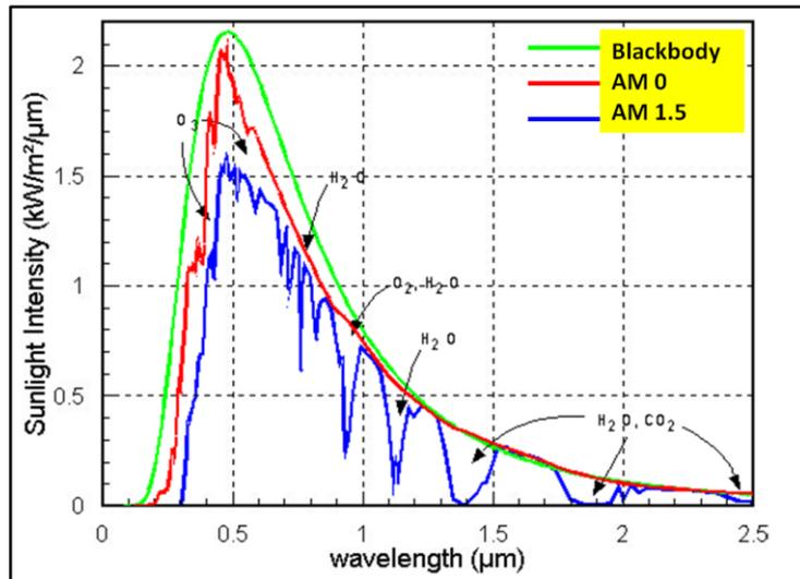
**Figure 7: Solar spectrum reaching the Earth's surface [10]. Blue curve represents the spectrum on the surface of the Earth. Absorption bands of water vapor, O<sub>2</sub>, and CO<sub>2</sub> are clearly seen**
