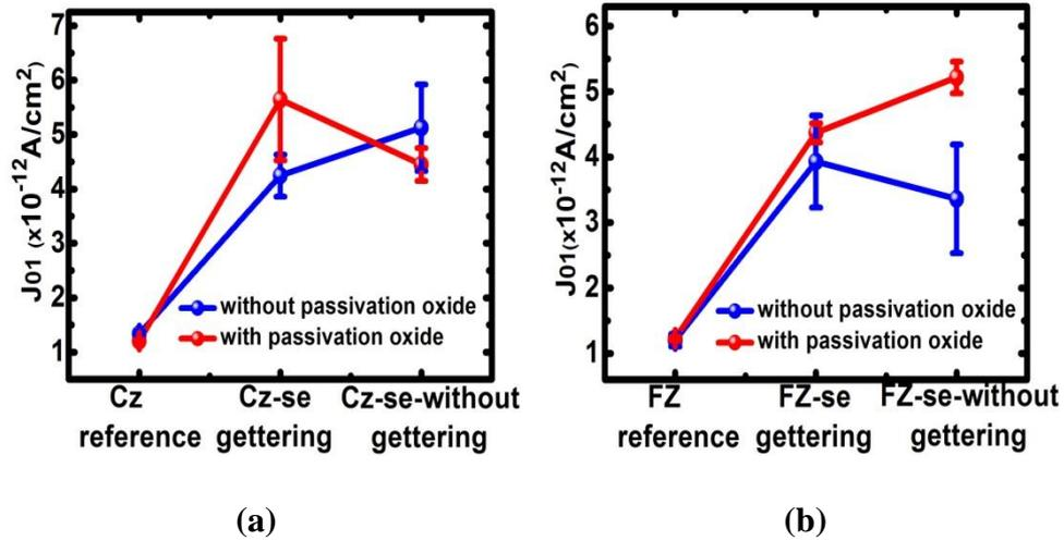
**Figure 95: Measured  $J_{01}$  values of fabricated (a) Cz and (b) FZ cells. Lines are for visual aid**
