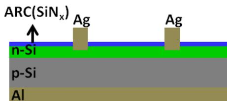
**Figure 12: Cross-sectional view of a standard Si solar cell**
