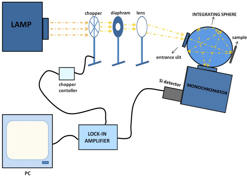
**Figure 47: Reflection set-up used in GUNAM Laboratories**
