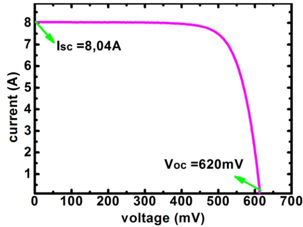
**Figure 10: I-V curve plotted in the 1<sup>st</sup> quadrant and representation of corresponding  $I_{sc}$  and  $V_{oc}$  values**
