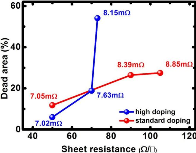
Figure 59: Effect of sheet resistance and dead area on series resistance
