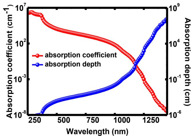
Figure 16: Absorption coefficient and depth of intrinsic Si at 300°K
