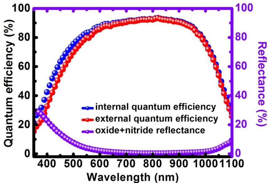
Figure 101: Internal and external quantum efficiency and corresponding reflectance spectrum of an oxide passivated reference cell
