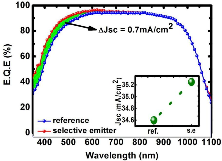
**Figure 97: EQE comparison of reference and selective emitter solar cells with corresponding short circuit current density enhancement**
