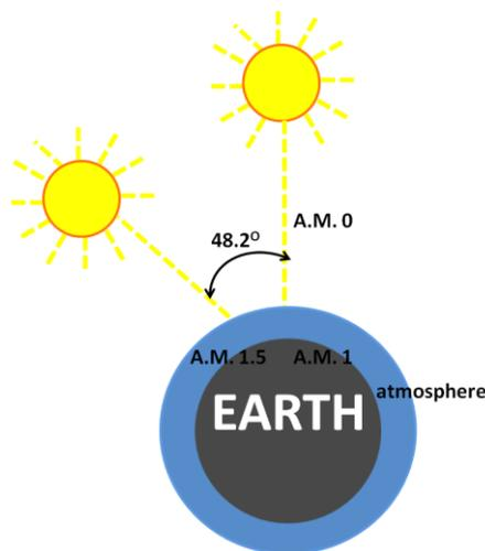
**Figure 8: Schematic of A.M. 0, 1 and 1.5 conditions**
