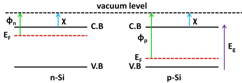
**Figure 21: Band diagram of n-Si and p-Si before electrical contact**
