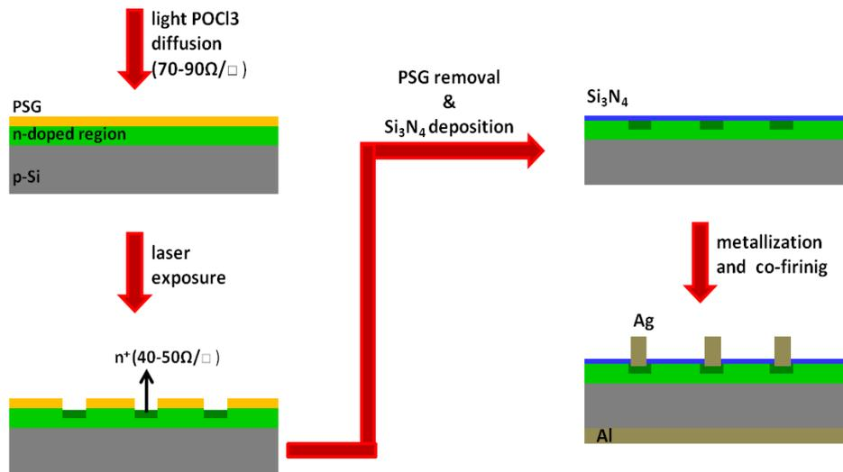
**Figure 32: Fabrication process of laser doped selective emitter solar cells with single step doping**
