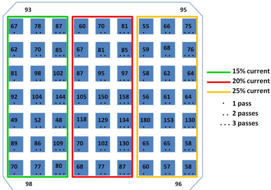
**Figure 67: Sheet resistance mapping on a full wafer with 4cm<sup>2</sup> laser scanned squares of different parameters**
