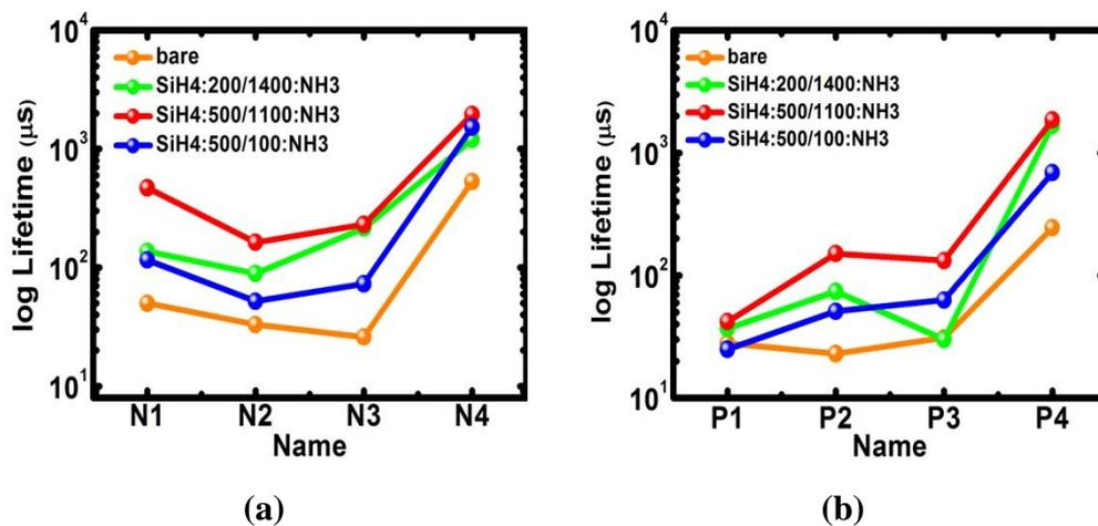
Figure 108: Effect of process gas flow ratio on lifetime of full (a) n-type, (b) p-type DSP wafers. Lines are for visual aid
