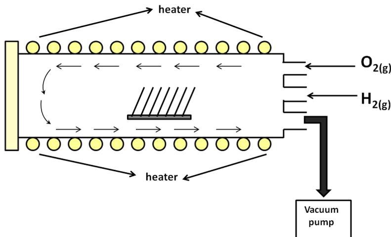
**Figure 44: Schematic of oxidation furnace**
