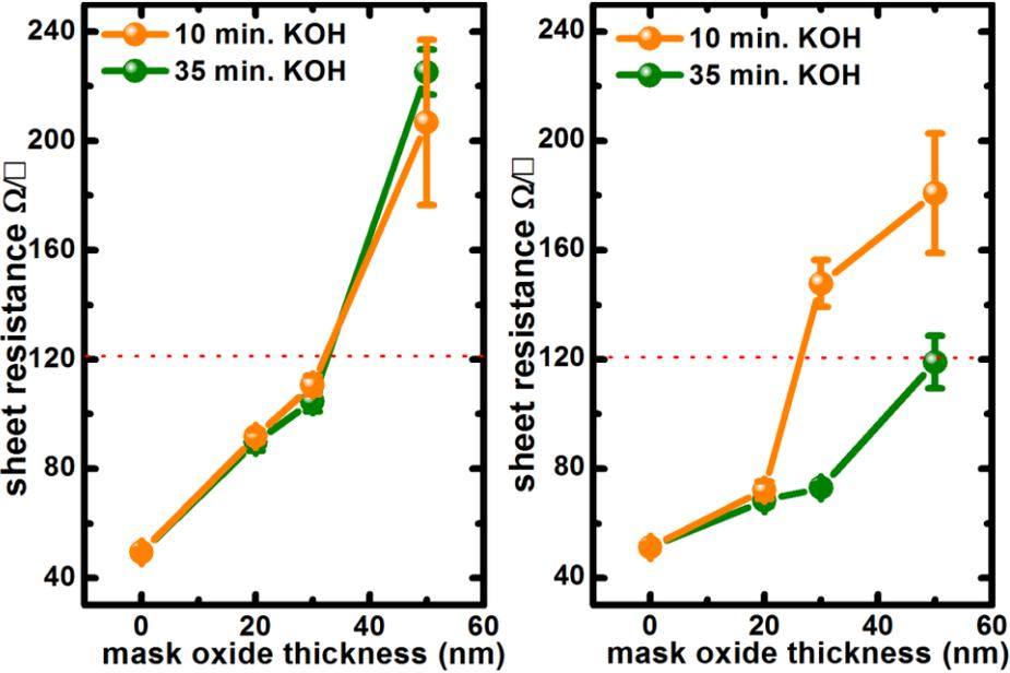
**Figure 54: Effect of 10% KOH dipping duration on sheet resistance of (a) standard doping, (b) high doping samples**
