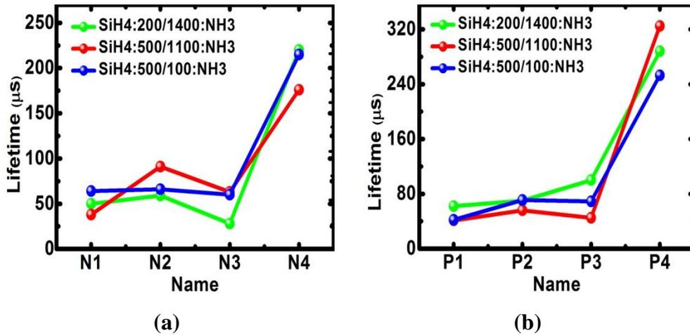
**Figure 106: Effect of process gas flow ratio on lifetime of (a) n-type, (b) p-type DSP samples. Lines are for visual aid**
