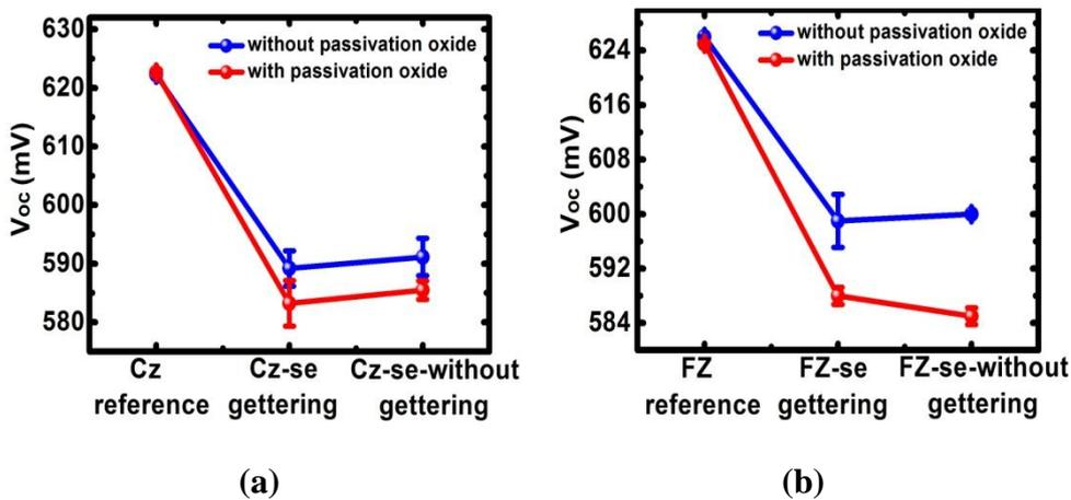
**Figure 88: Open circuit voltage values of fabricated (a) Cz and (b) FZ cells. Lines are for visual aid**
