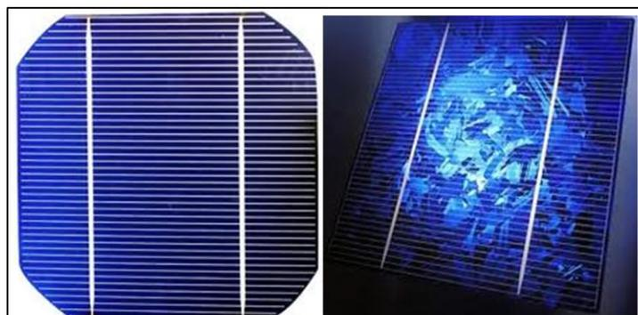
**Figure 4: Industrial mono and multi crystalline silicon solar cells [5]**
