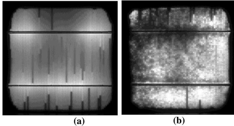
**Figure 76: Electroluminescence images of reference cells (a) without oxide passivation, (b) with oxide passivation. Lines are for visual aid**
