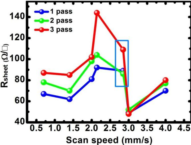
**Figure 69: Effect of laser scan speed on sheet resistance. Lines are for visual aid**
