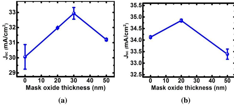
**Figure 73: Effect of mask oxide thickness on  $J_{sc}$  (a) with oxide passivation, (b) without oxide passivation. Lines are for visual aid**
