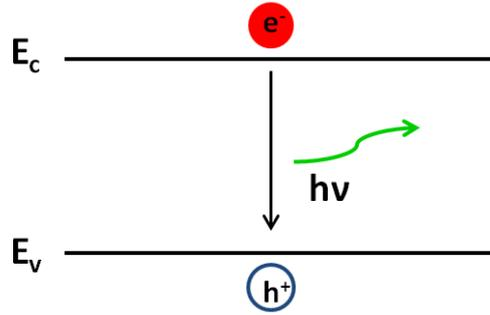
**Figure 39: Schematic of radiative recombination process**
