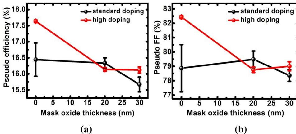
**Figure 62: Effect of mask oxide thickness on (a) pseudo efficiency, (b) pseudo fill factor**
