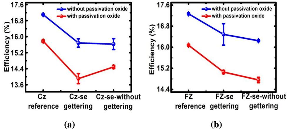
**Figure 86: Efficiency values of fabricated (a) Cz and (b) FZ cells. Lines are for visual aid**
