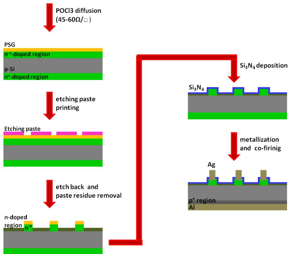
**Figure 31: Fabrication process of emitter etch back selective emitter solar cells**
