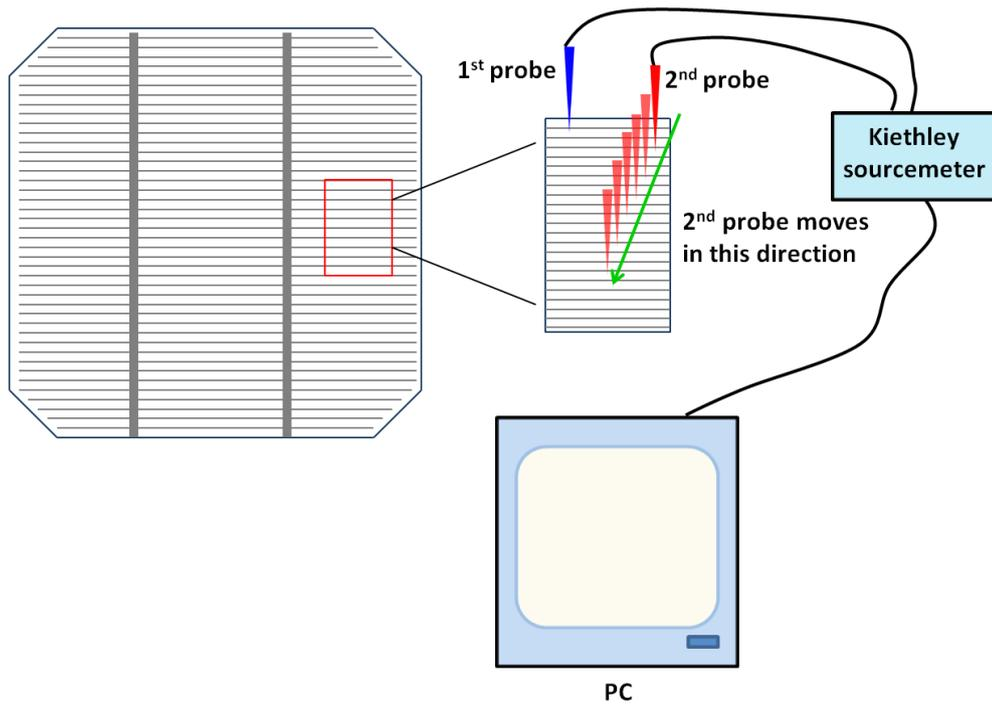
**Figure 50: Schematic of contact resistance measurement system**
