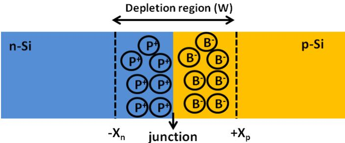
**Figure 20: Cross-sectional view of a p-n junction**
