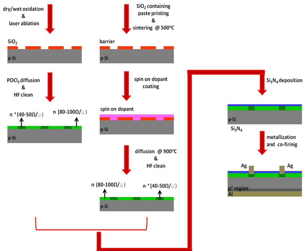
**Figure 38: Fabrication process of selective emitter solar cells using silicon dioxide diffusion barrier**
