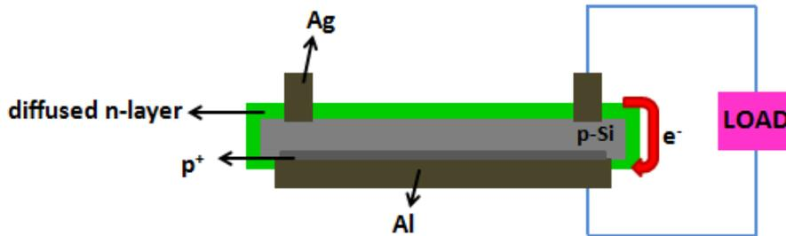
**Figure 29: Operation of a Si solar cell before edge isolation**
