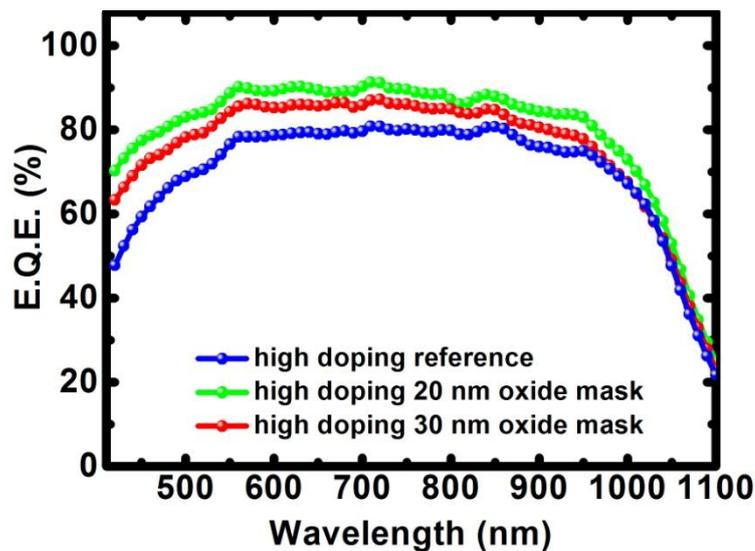
**Figure 65: Effect of mask oxide thickness on external quantum efficiency of high doping samples**
