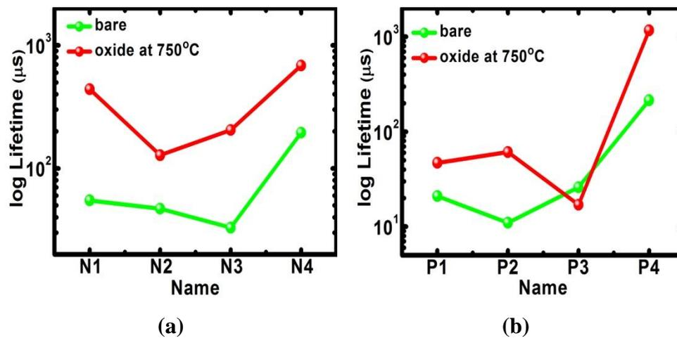
**Figure 110: Effect of oxide passivation via pyrogenic oxidation on lifetime of full (a) n-type, (b) p-type DSP wafers. Lines are for visual aid**
