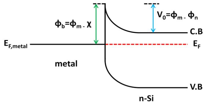
**Figure 25: Band diagram of metal-n-Semiconductor junction after physical contact**
