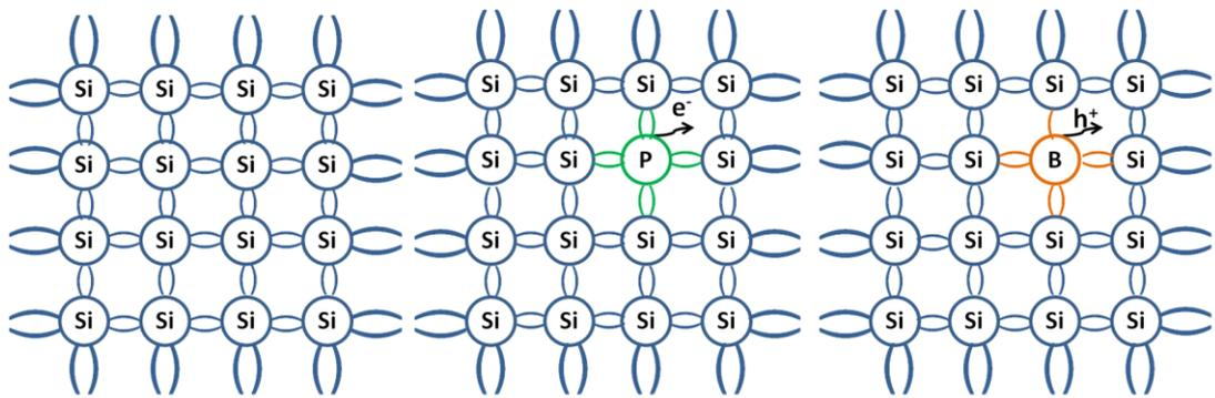
**Figure 19: Crystal structure of intrinsic Si (a), phosphorous Si (b) and boron doped Si (c)**
