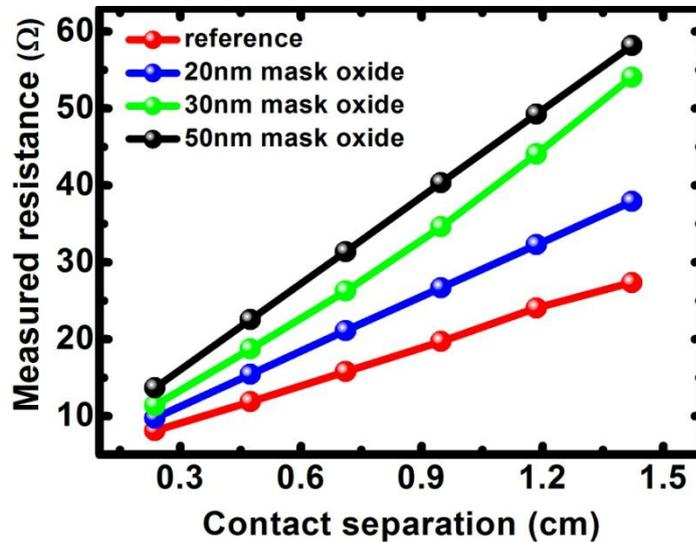
Figure 84: Resistance measurements by transferring line method. Lines are for visual aid
