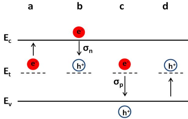
**Figure 41: Schematic of Shockley Read Hall mechanism: (a) electron emission, (b) electron capture, (c) hole capture, (d) hole emission**
