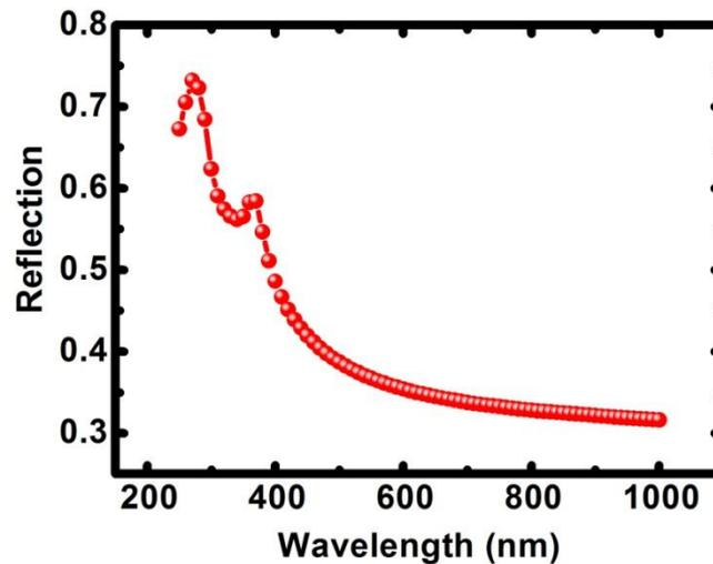
**Figure 23: Reflection spectrum of bare silicon**
