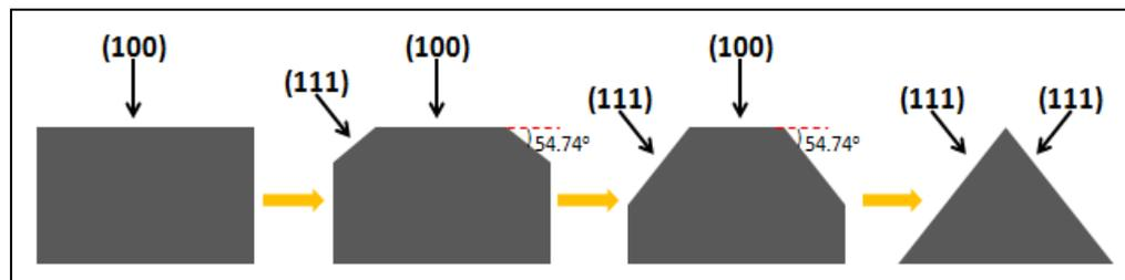
**Figure 17: Etching process of (100) Si**
