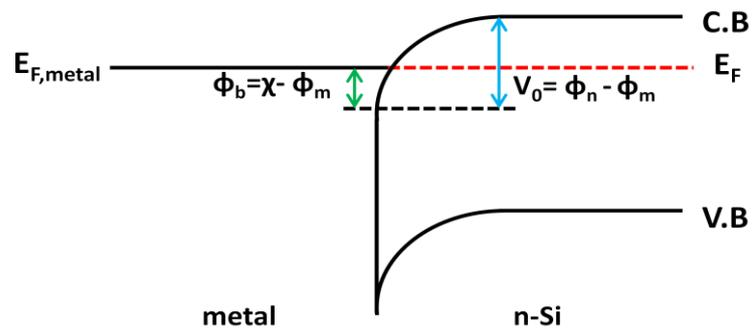
**Figure 27: Band diagram of metal & n-Semiconductor after physical contact**
