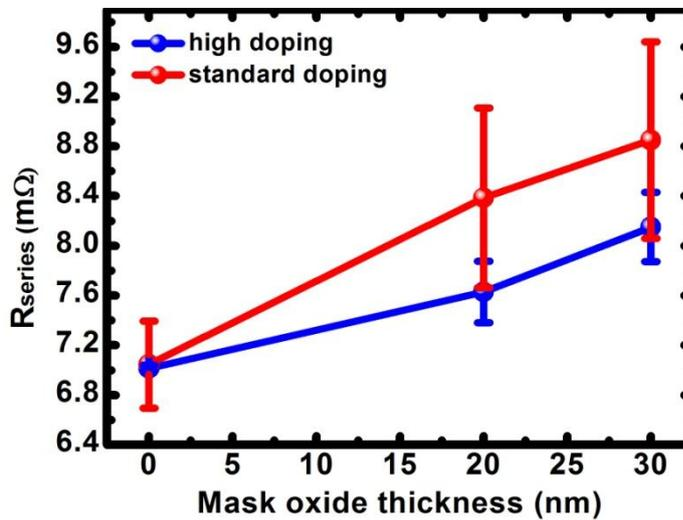
Figure 57: Effect of mask oxide thickness on series resistance
