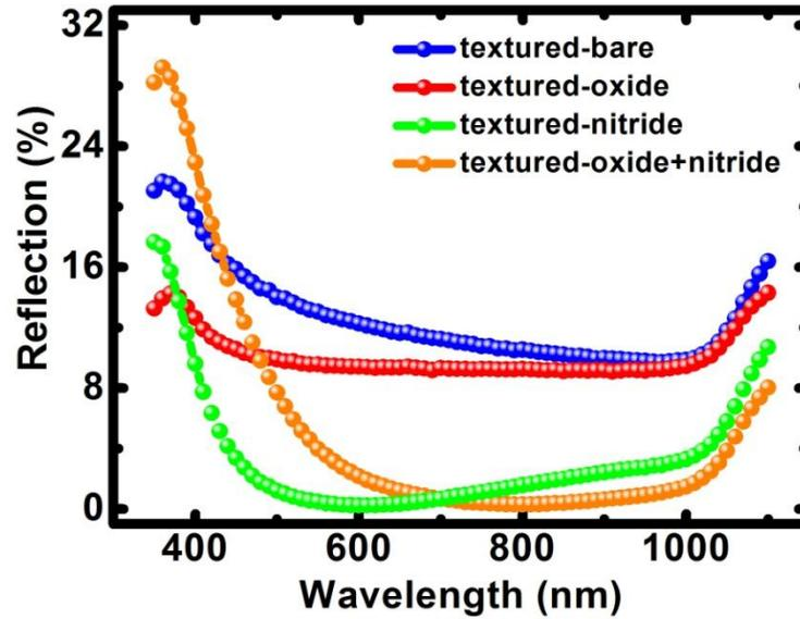
**Figure 99: Reflection spectra of bare , oxide, nitride and oxide/nitride stack existing textured silicon surfaces**
