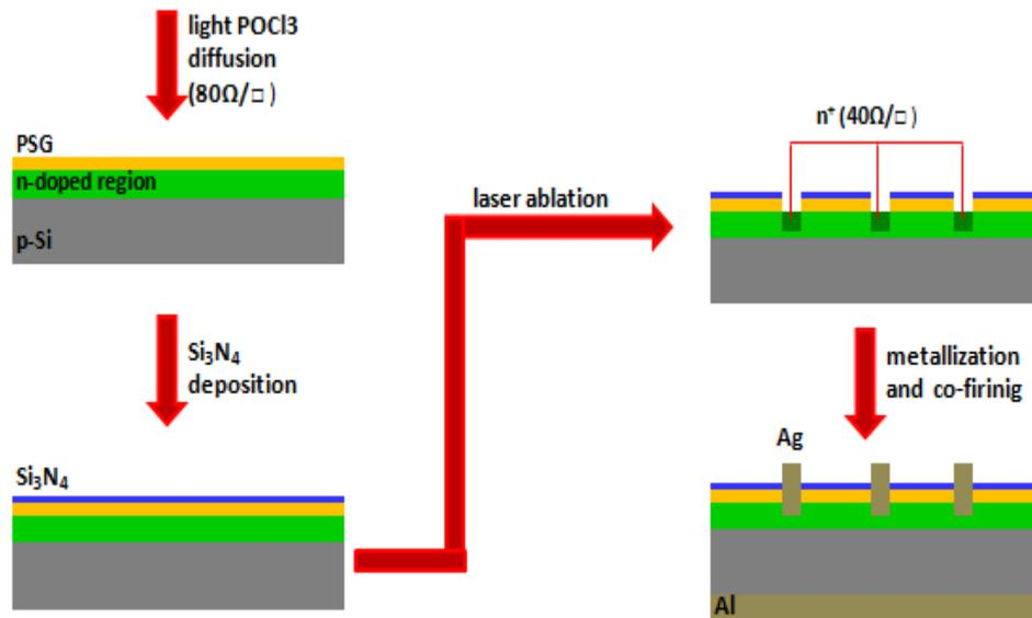
**Figure 34: Fabrication process of laser doped selective emitter solar cells with single step doping**
