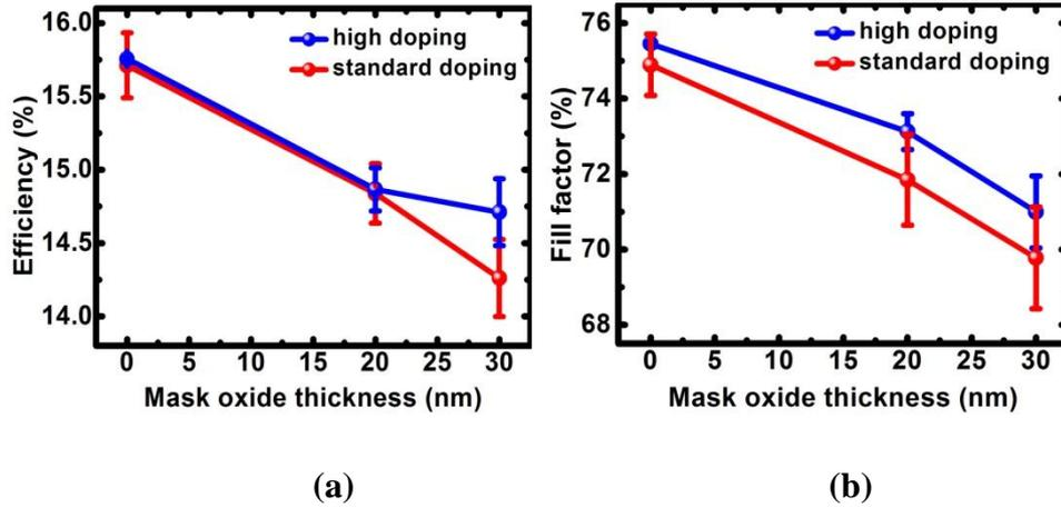
**Figure 55: Effect of mask oxide thickness on (a) cell efficiency, (b) fill factor**
