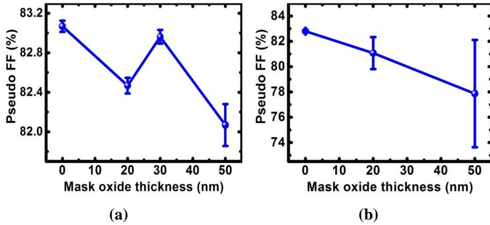
Figure 79: Effect of mask oxide thickness on pseudo fill factor (a) with (b) without oxide passivation. Lines are for visual aid
