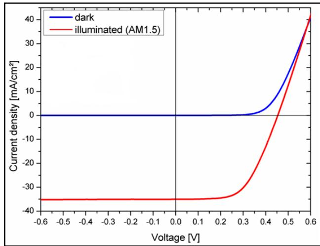
**Figure 9: I-V Characteristics of solar cell under dark and illuminated conditions [11]**
