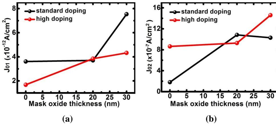
**Figure 64: Effect of mask oxide thickness on (a)  $J_{01}$  and (b)  $J_{02}$**
