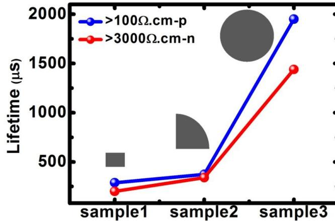
Figure 107: Effect of sample shape on lifetime. Lines are for visual aid
