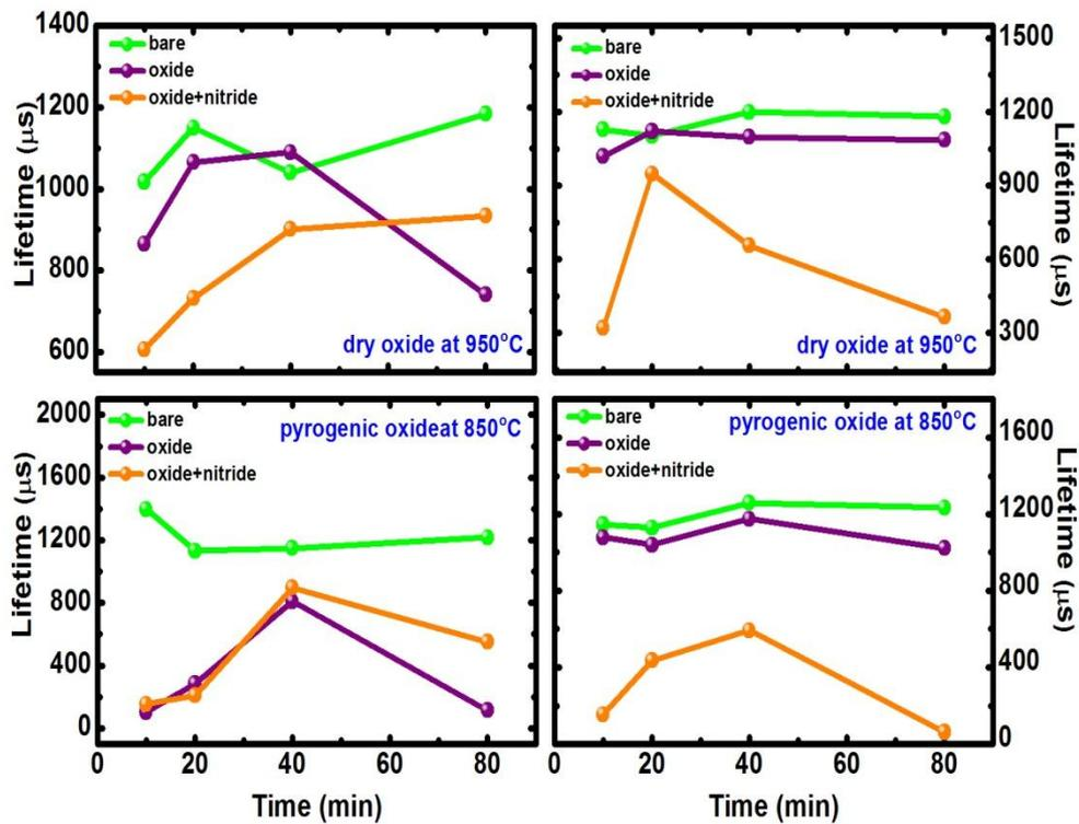
**Figure 112: Performance of oxide / nitride stack structure. Lines are for visual aid**
