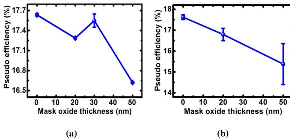
**Figure 78: Effect of mask oxide thickness on pseudo efficiency (a) with (b) without oxide passivation. Lines are for visual aid**
