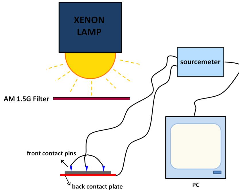
**Figure 48: Schematic of solar simulator**
