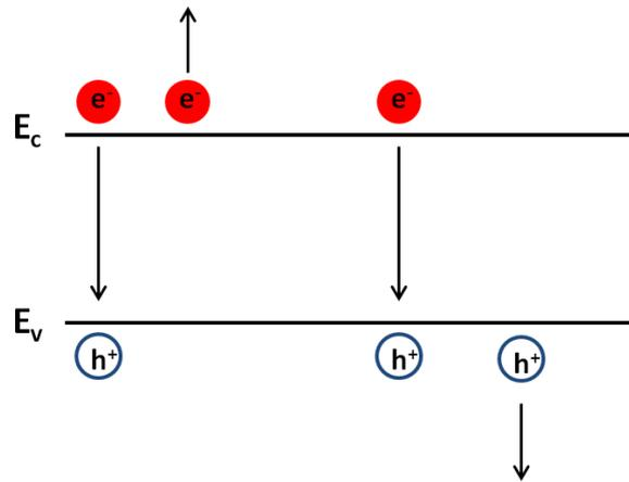
**Figure 40: Schematic of Auger recombination process**
