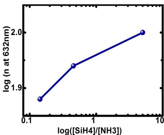
**Figure 105: Effect of process gas flow ratio on refractive index at 632 nm. Lines are for visual aid**
