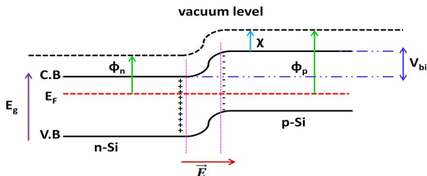
**Figure 22: Band diagram of the system after p-n junction formation**
