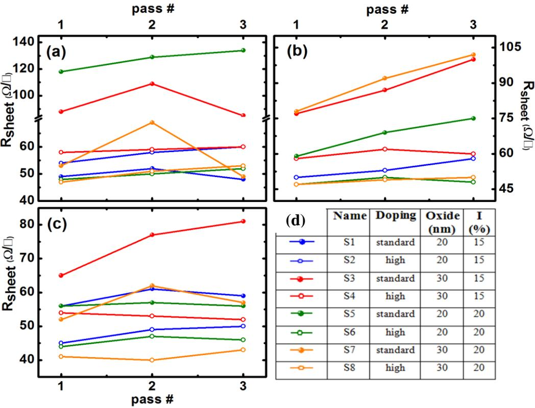
**Figure 68: Effect of (a) 5sec., (b) 10sec., (c) 17 sec HF dipping on sheet resistance of both high and standard doping samples with 20,30 and 50 nm mask oxide layers for laser speed: 3mm/s with table (d) of symbol about corresponding doping recipe, oxide thickness and laser current. Lines are for visual aid**
