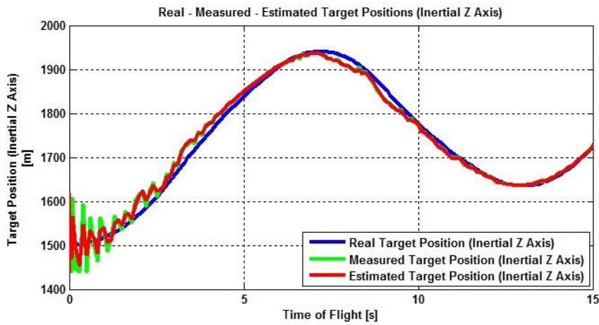
Figure 5.7: Target Position Estimation along Z_{ref} by 3 rd Order Fading Memory Filter
