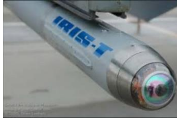
Figure 4.9: Gimbaled Infrared Seeker of Short-Range Infrared IRIS-T Missile [18]
