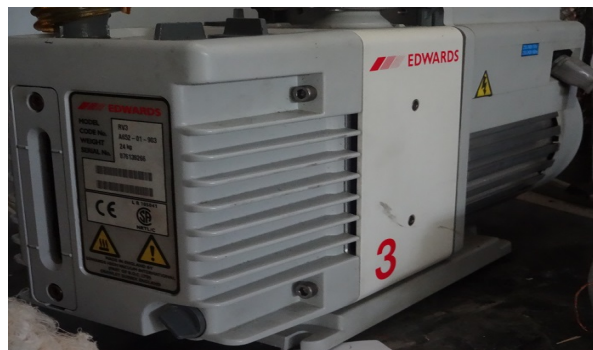
Figure 5.5: The photograph of the rotary vacuum pump used in the system.
