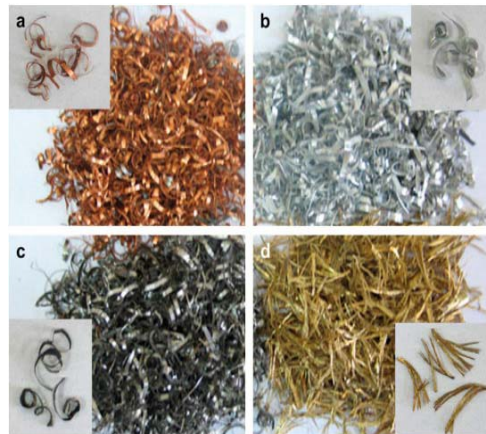
Figure 1.15: metal chips: a) copper; b) aluminum; c) stainless steel; d) brass [10].
