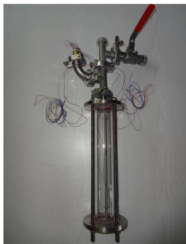
Figure 5.3: The photograph of the evaporator/condenser component used in the system.
