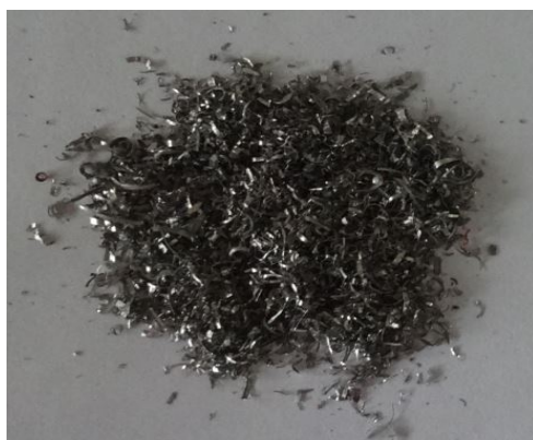
Figure 3.2: Picture of the prepared aluminum metal additive.
