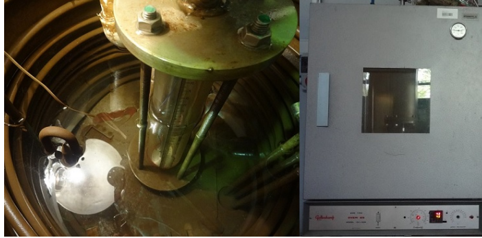
Figure 5.4: The photograph of the water bath and oven used in the system.
