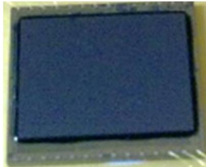
**Figure 4.17.** 320x256 HgCdTe FPA hybridized with ROIC
