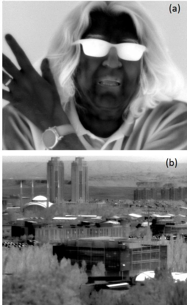
**Figure 2.25.** Thermal images recorded with the InP/InGaAs QWIP FPA (a) at  $\sim 80$  K, (b) at  $\sim 65$  K. The second thermal image is recorded with  $300 \mu\text{s}$  integration time [108].
