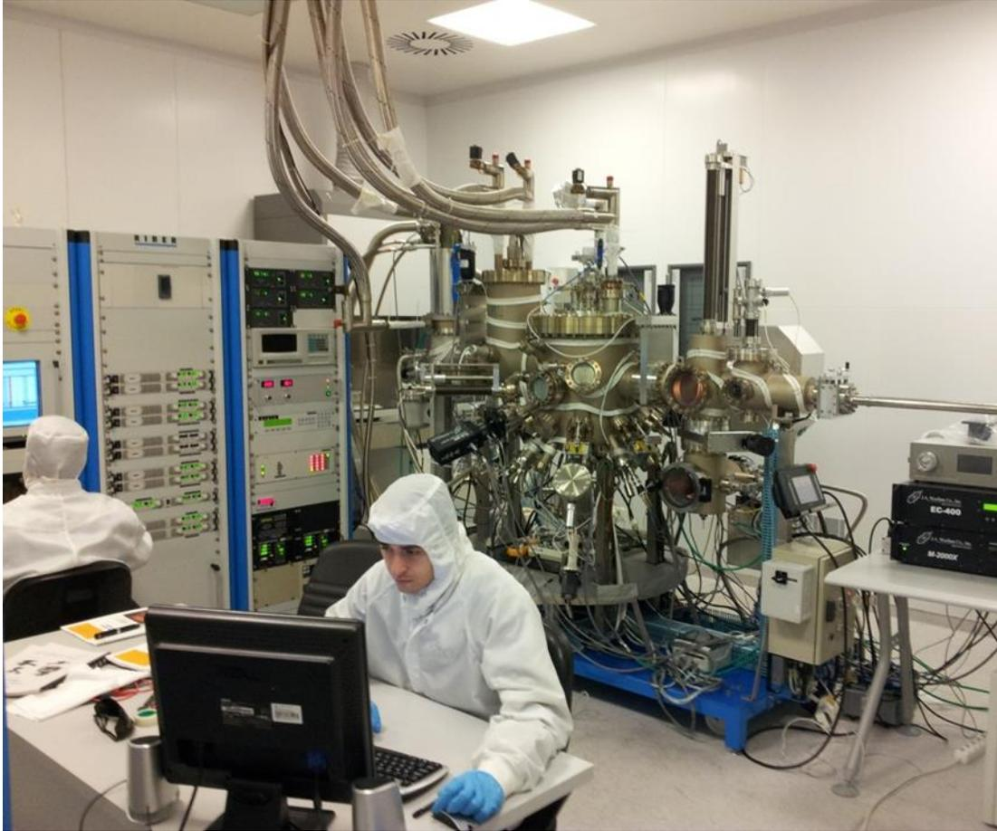
**Figure 4.2.** Riber C21 reactor used in HgCdTe growths
