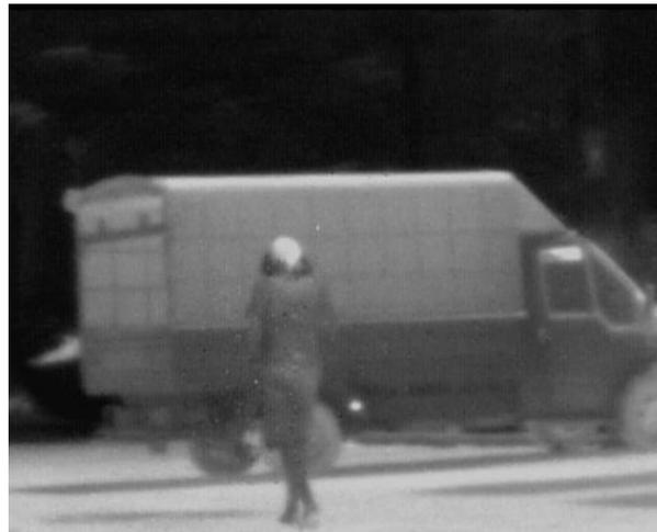
**Figure 4.18.** Thermal image recorded with 320x256 FPA fabricated with LWIR HgCdTe detector epilayer structure grown on Si substrate
