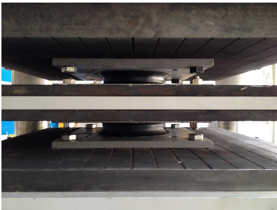
Figure C.3: C-15 bearing in the case of a tension without displacement
