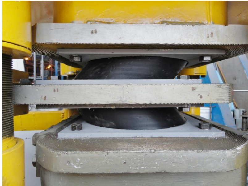
Figure C.1: O-30 bearing in the case of an 100% shear deformation under tension
