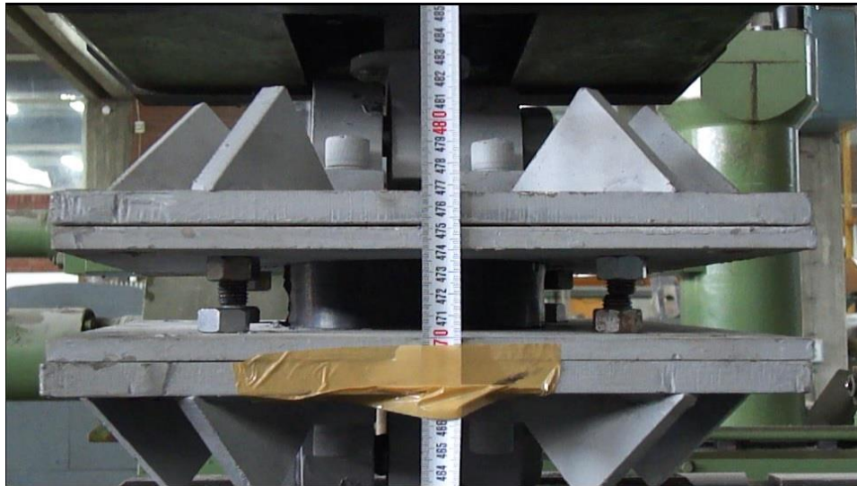
Figure C.6: O-15 bearing in the case of pure tension with %0 strain
