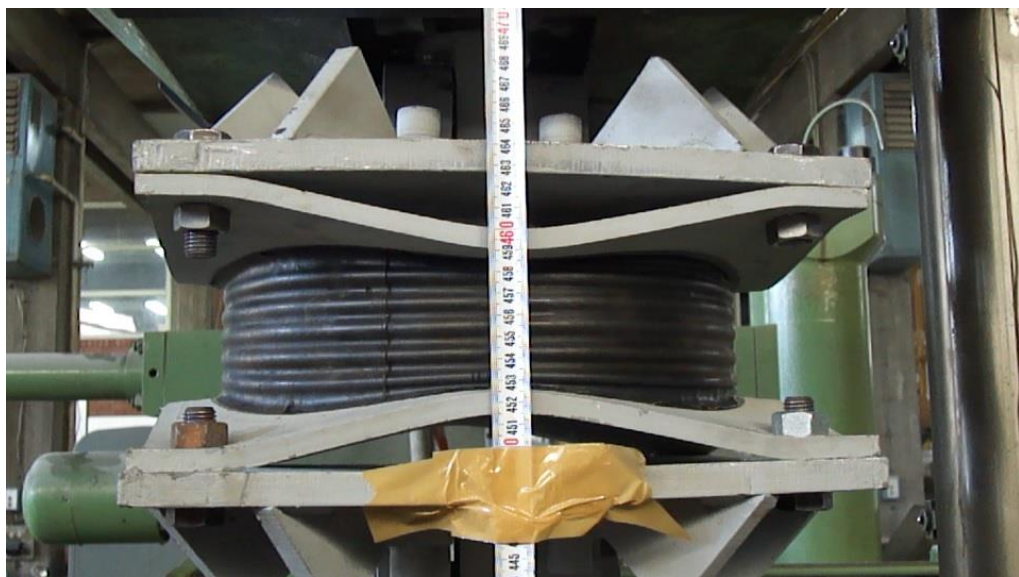
Figure C.14: O-30 bearing in the case of pure tension when outer plates are bended
