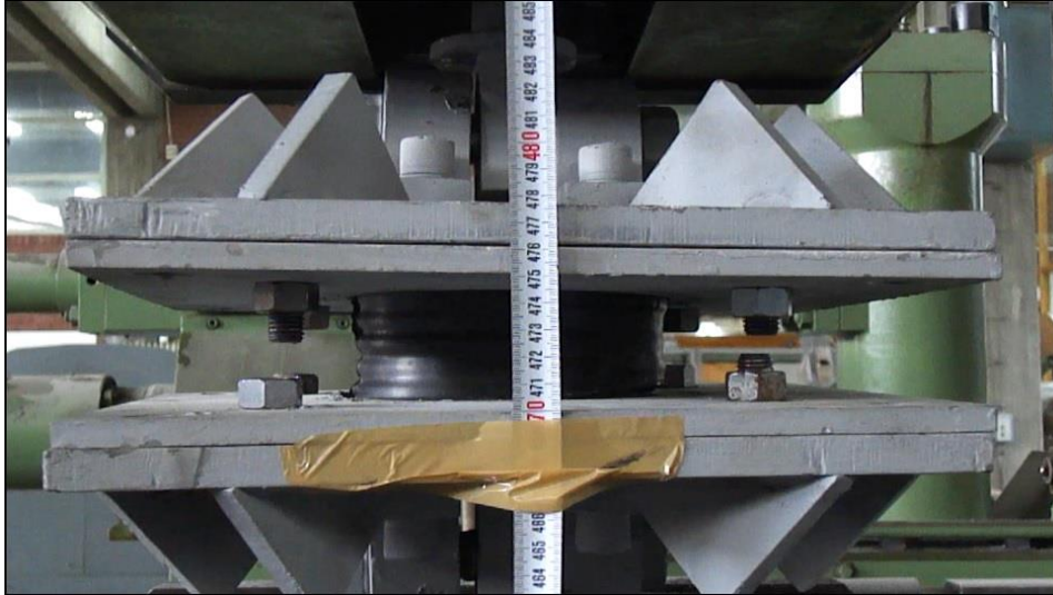
Figure C.7: O-15 bearing in the case of pure tension with %25 strain
