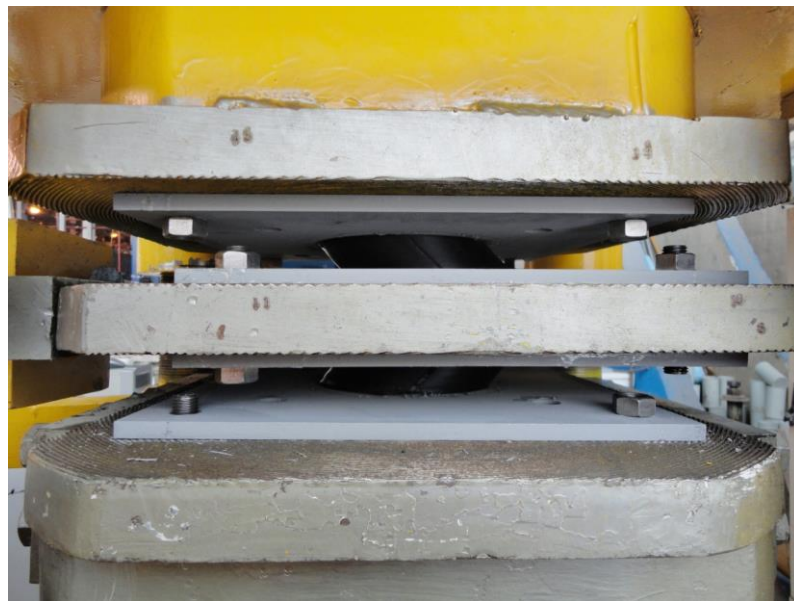
Figure C.2: O-15 bearing in the case of an 100% shear deformation under tension
