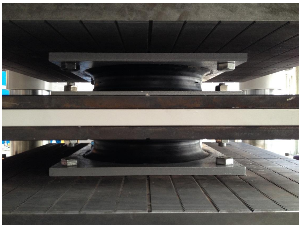
Figure C.4: C-30 bearing in the case of a tension without displacement
