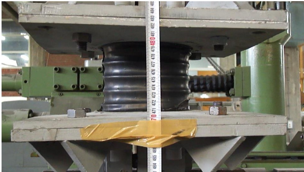
Figure C.11: O-15 bearing in the case of pure tension with %220 strain
