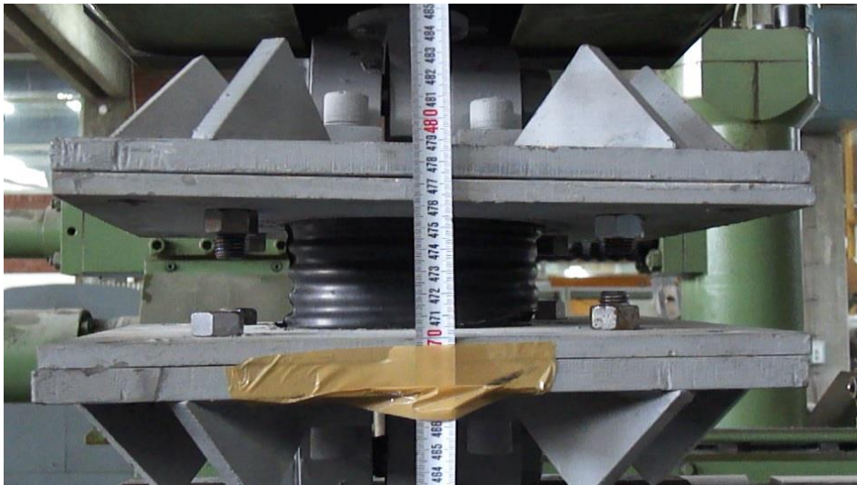
Figure C.8: O-15 bearing in the case of pure tension with %50 strain
