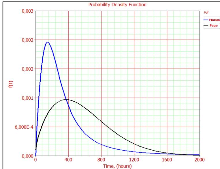
Figure A.31 PDF curves of Rigging - Rope
