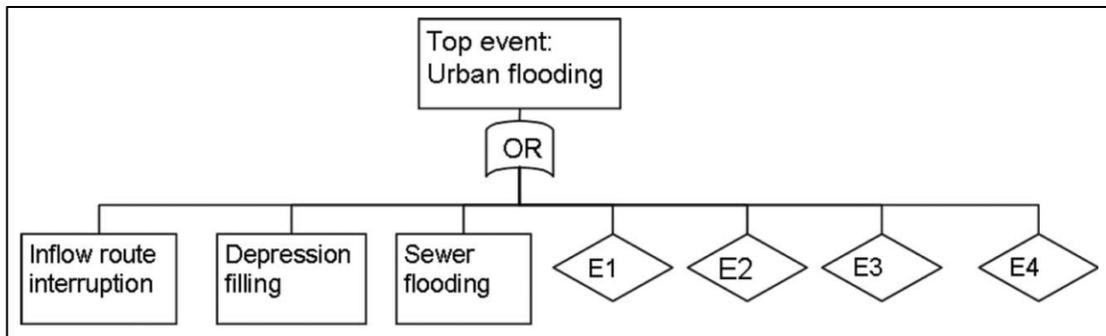
Figure 2.12 Fault tree representation for the urban flooding (Veldhuis *et al*, 2011)
