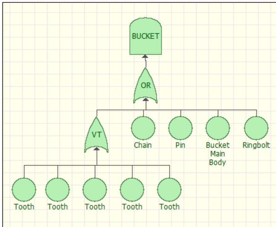
Figure 4.10 Fault tree representation of bucket units
