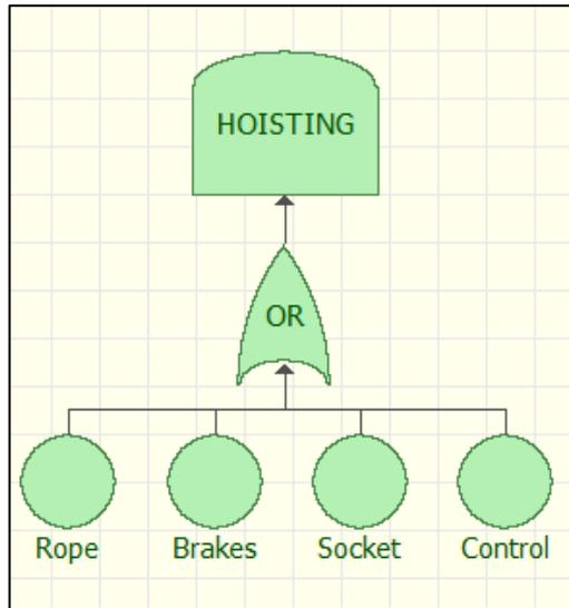
Figure 4.6 Fault tree representation of hoisting units
