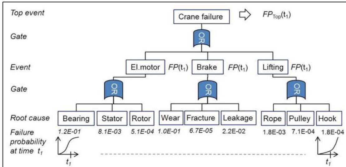
Figure 2.10 Fault tree representation of the crane system (Halme and Aikala, 2012)
