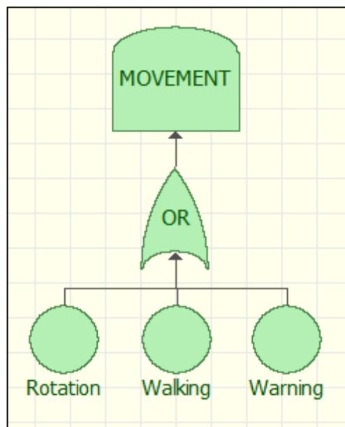
Figure 4.12 Fault tree representation of movement units
