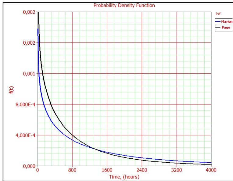
Figure A.19 PDF curves of Dragging – Chain
