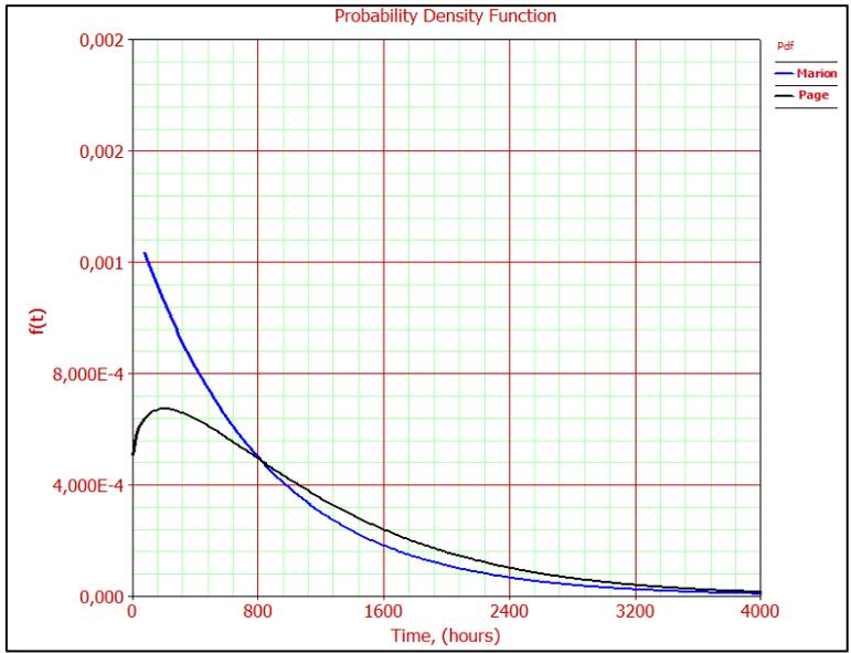
Figure A.17 PDF curves of Dragging – Ringbolt
