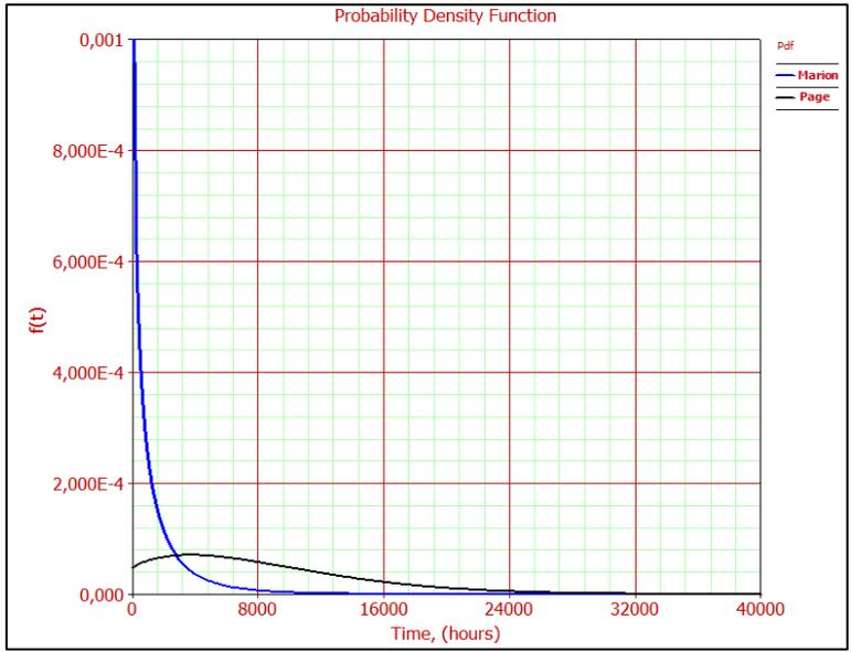
Figure A.26 PDF curves of Hoisting - Control
