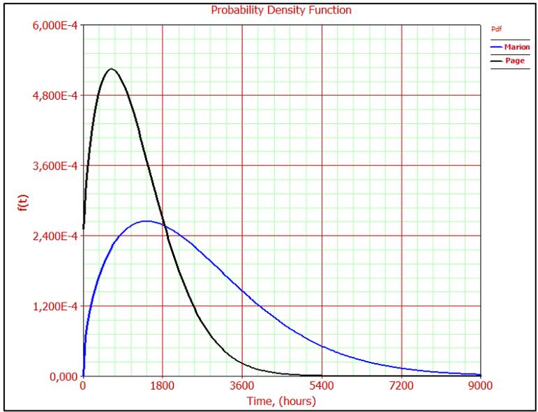
Figure A.25 PDF curves of Hoisting - Rope
