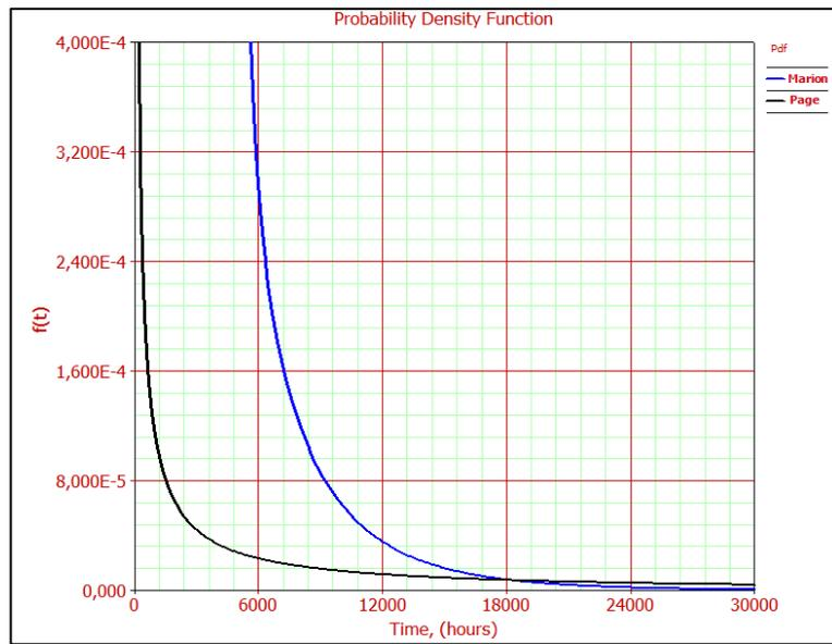
Figure A.43 PDF curves of Bucket – Chains
