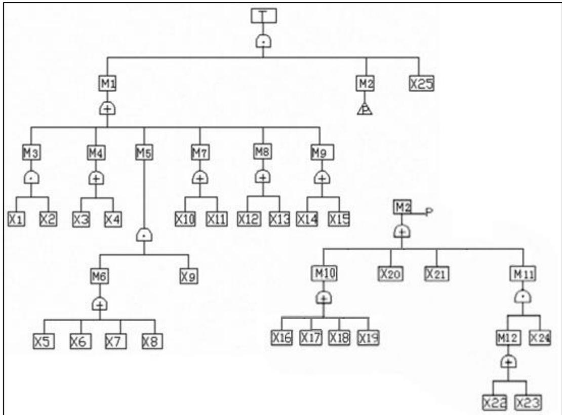
Figure 2.7 Fault tree representation of the system (Wang, 2010)
