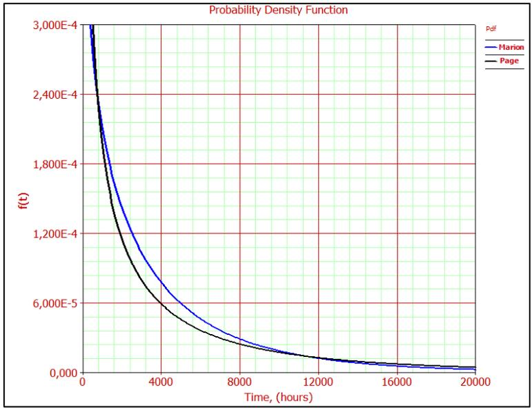
Figure A.33 PDF curves of Rigging – Ringbolt
