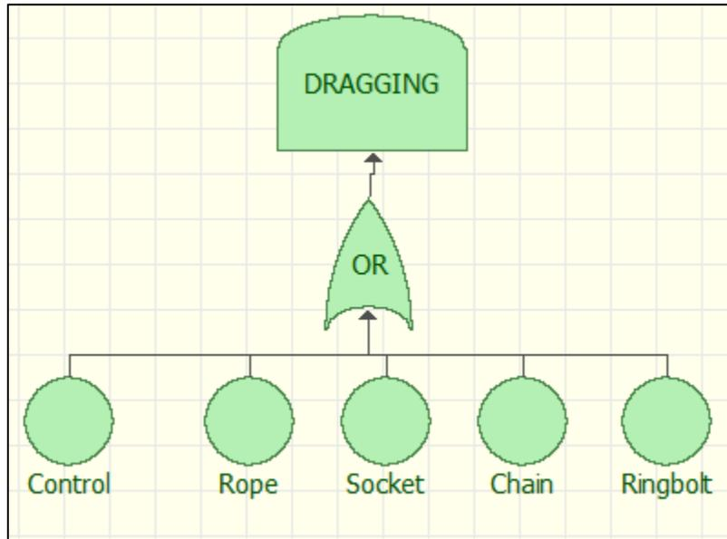
Figure 4.4 Fault tree representation of dragging units
