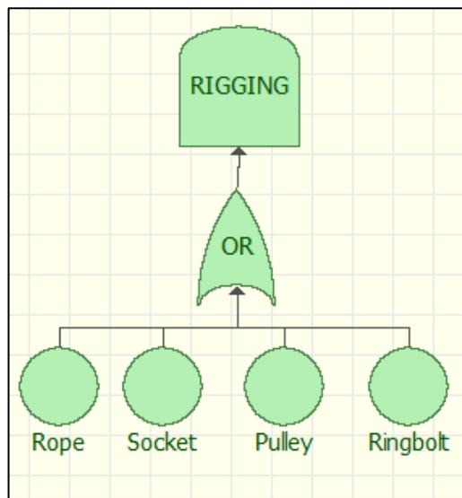
Figure 4.8 Fault tree representation of rigging units
