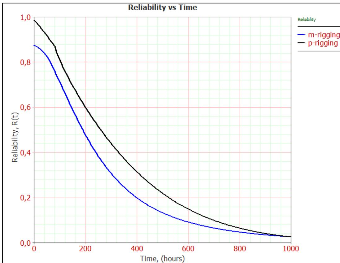
Figure 4.9 Reliability graph of rigging units
