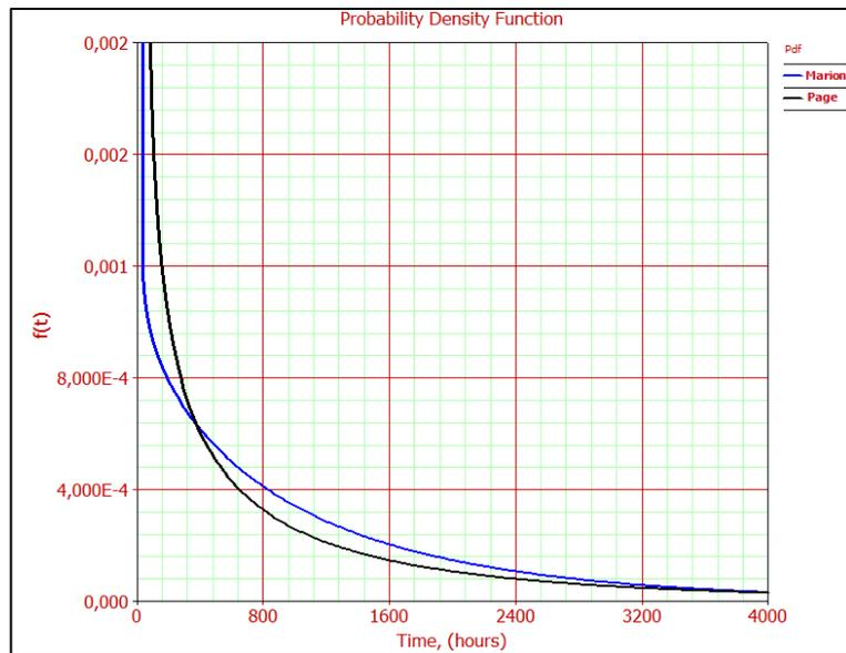
Figure A.40 PDF curves of Bucket – Ringbolt
