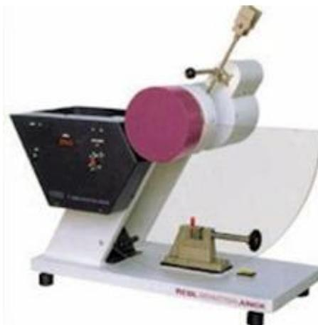
**Figure 3.13** Impact testing instrument [71]
