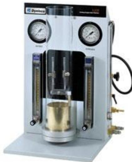
**Figure 3.10** The limiting oxygen index test instrument [70]
