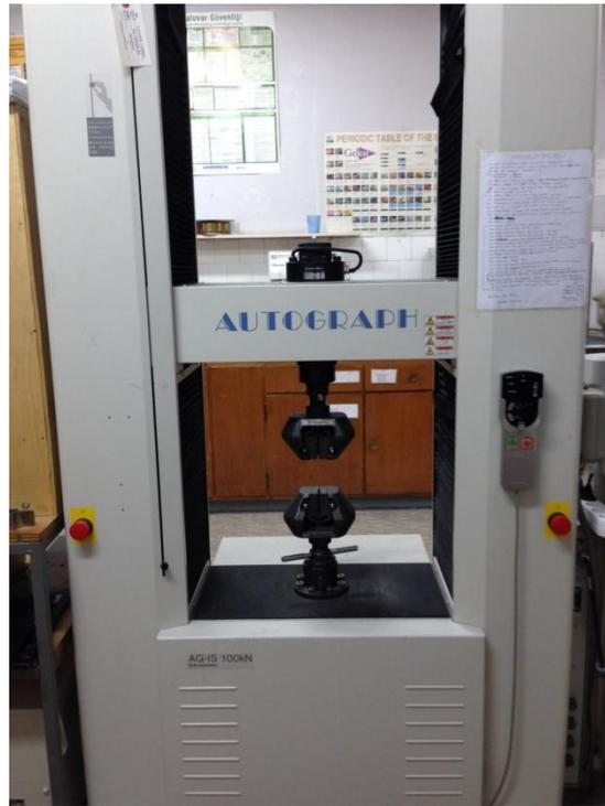
**Figure 3.11** The universal tensile testing instrument
