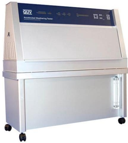
**Figure 3.14** QUV Accelerated Weathering Tester Machine [72]
