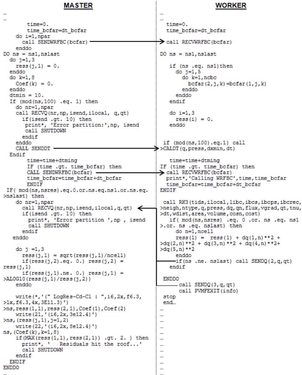
Figure 2.8: Master and worker routines of HYP3D
