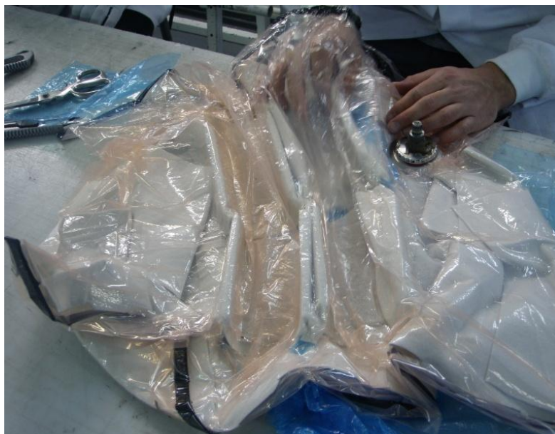
Figure 28: Intermediate vacuum bagging process
