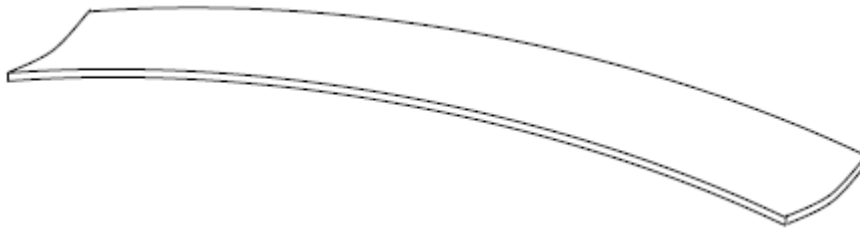
Figure 16: Warpage on an initially flat part [30]
