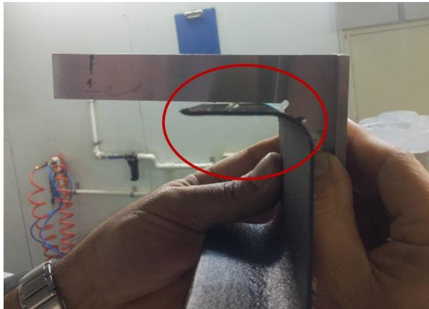
Figure 34: Spring-in of a composite part by eye inspection
