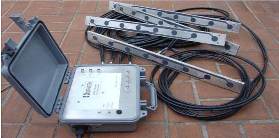
Figure 4-7: SeaTek ultrasonic bathymetry measurement device.
