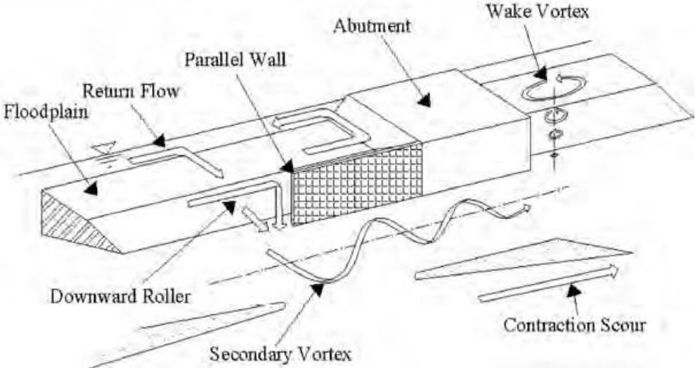
Figure 3-5: Flow patterns with parallel wall application (Barkdoll, Ettema & Melville, 2007).
