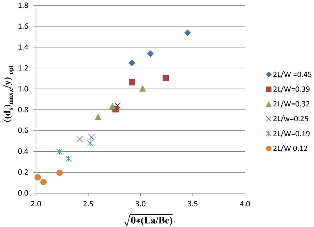
Figure 5-5: Variation of  $((d_s)_{max,c}/y)_{opt}$  with respect to  $[\theta(L_a/B_c)]^{0.5}$ .
