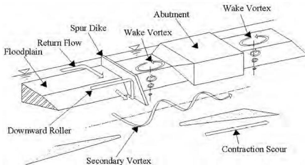
Figure 3-4: Flow patterns with spur dike application (Barkdoll, Ettema & Melville, 2007).
