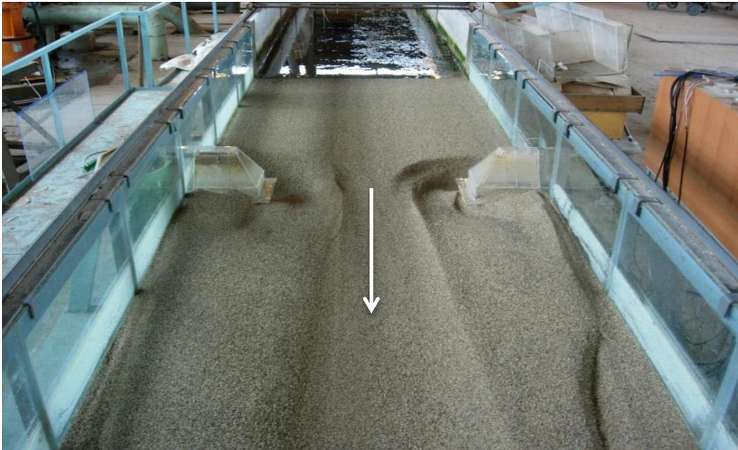
Figure 5-2: View of scour hole around abutment with a collar of 5 cm at  $Z_c=-0.5$ .
