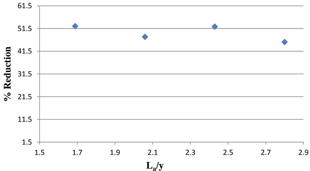
Figure 5-7: Distribution of percent reduction with abutment length for single abutment.
