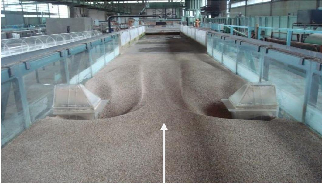
Figure 4-1: Downstream and sediment storage part of the flume after the experiment.
