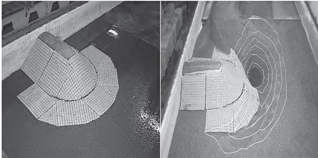
Figure 3-2: Cable tied blocks application before and after scour (Barkdoll, Ettema & Melville, 2007).
