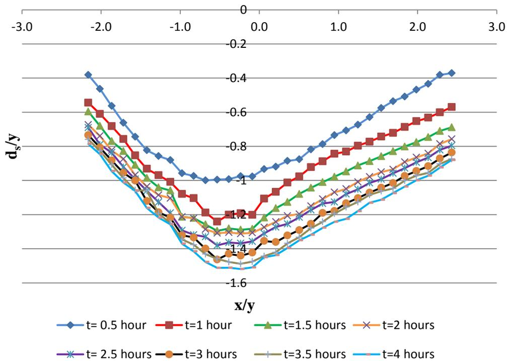
Figure 5-12: Temporal variation of scour hole without collar for the contraction ratio of  $2L/W=0.45$  at section I.
