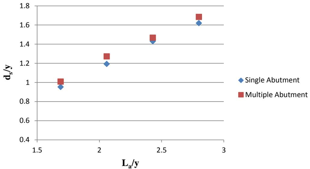
Figure 5-9: Comparison of maximum scour depths for single and multiple abutment case without collar application.
