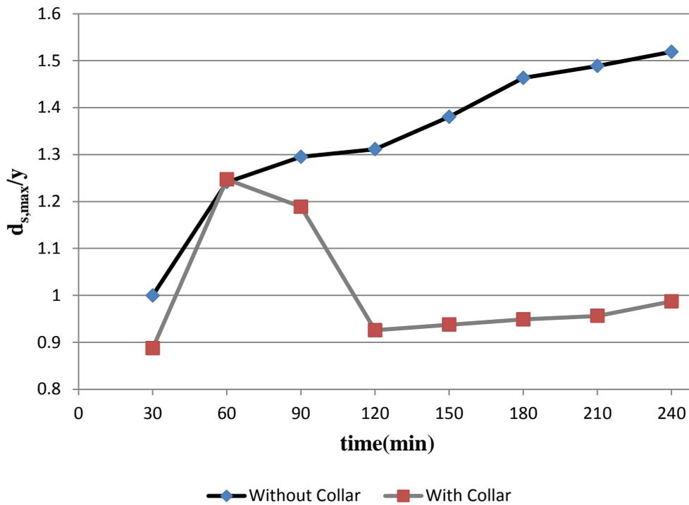
Figure 5-14: Variation of maximum scour depths with time for cases with and without collar at section I.
