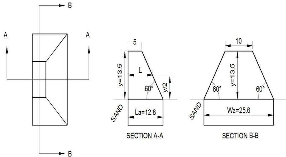
Figure 4-3: Abutment model for shortest length.
