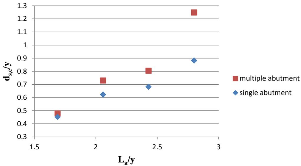
Figure 5-10: Comparison of maximum scour depths for single and multiple abutment case with collar application.
