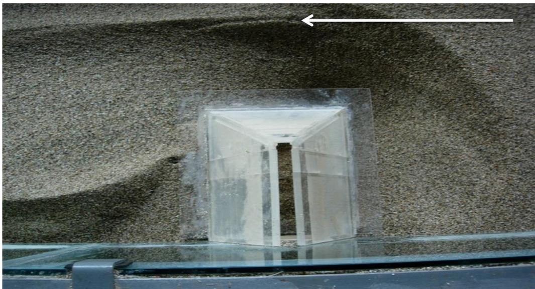
Figure 5-1: Scour hole with a collar of 5cm at  $Z_c=0$ .
