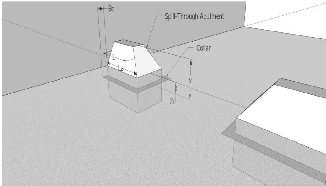
Figure 4-2: Representation of the abutment model and collar in the channel.
