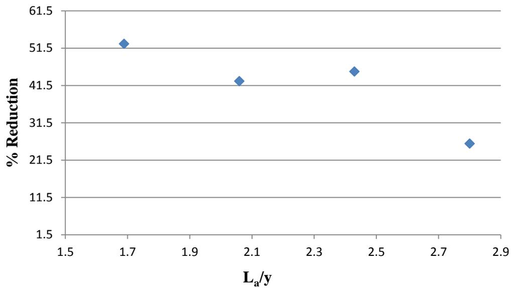
Figure 5-8: Distribution of percent reduction with abutment length for multiple abutment.
