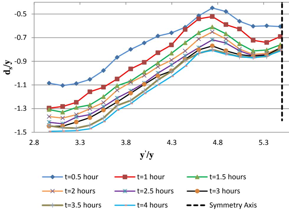
Figure 5-15: Temporal variation of scour hole without collar for the contraction ratio of  $2L/W=0.45$  at section II.
