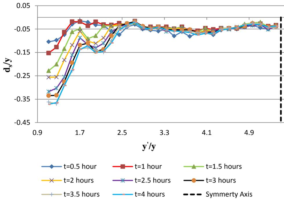
Figure 5-17: Temporal variation of scour hole without collar protection for the contraction ratio of  $2L/W=0.12$  at section II.
