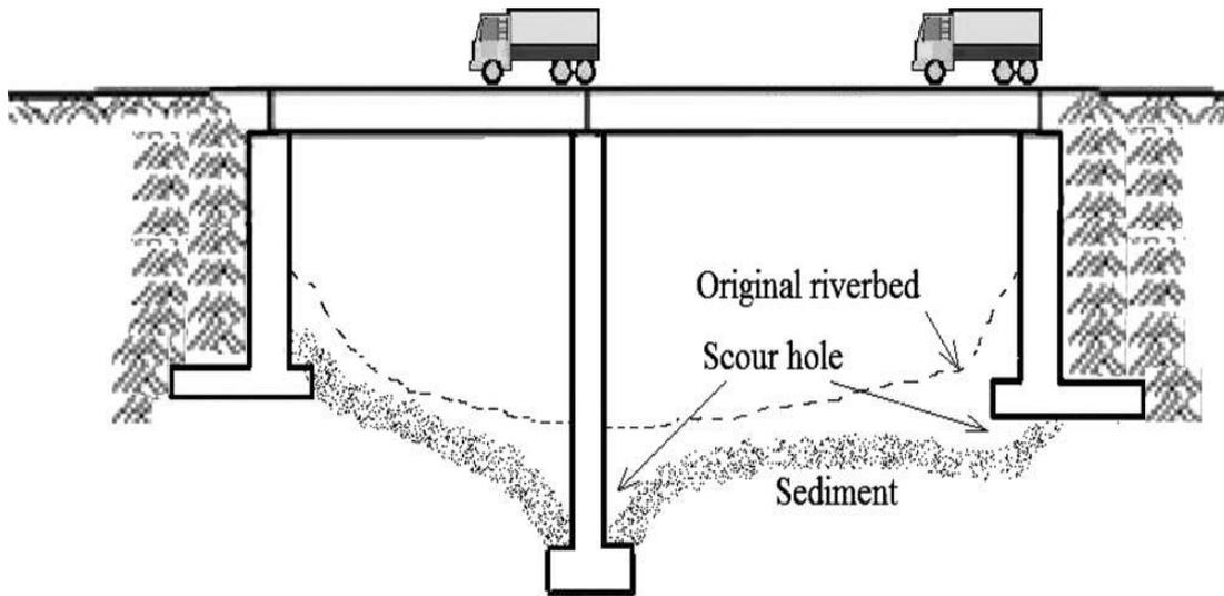
Figure 2-1: Scour hole around bridge (Deng & Cai, 2010).
