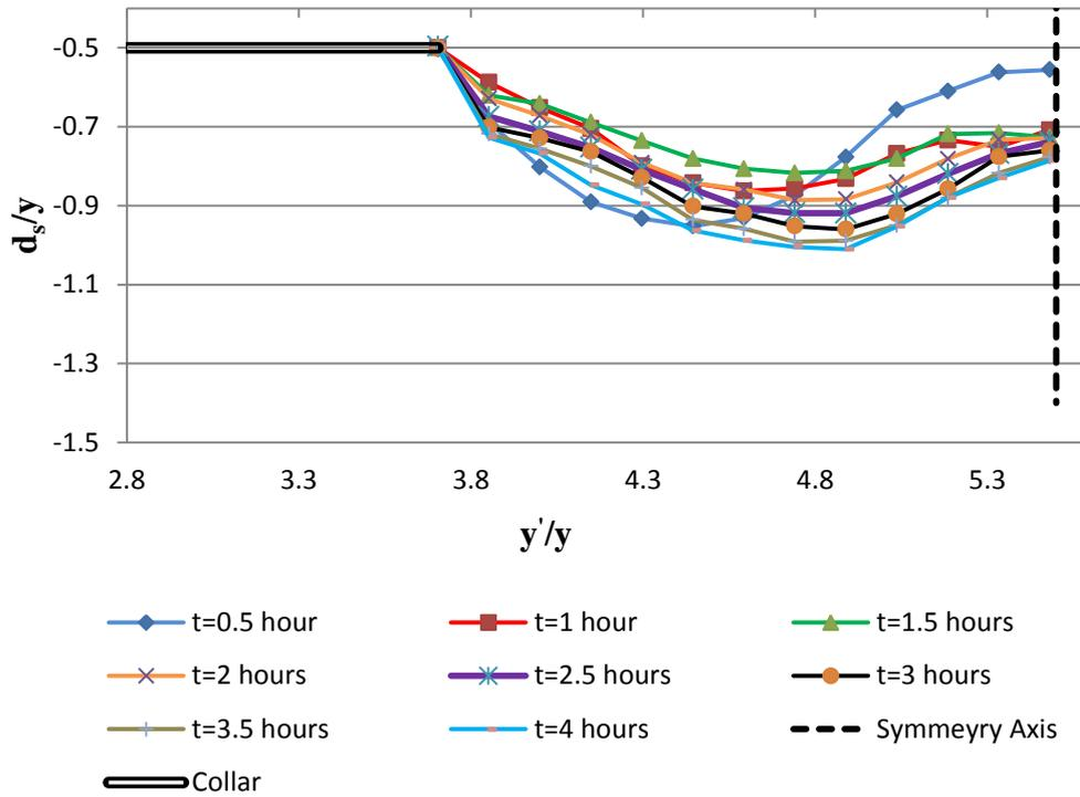
Figure 5-16: Temporal variation of scour hole with collar protection for the contraction ratio of  $2L/W=0.45$  at section II.
