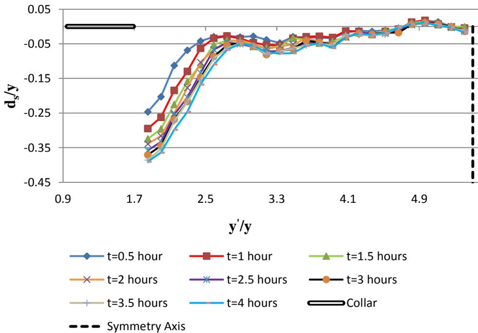
Figure 5-18: Temporal variation of scour hole with collar protection for the contraction ratio of  $2L/W=0.12$  at section II.
