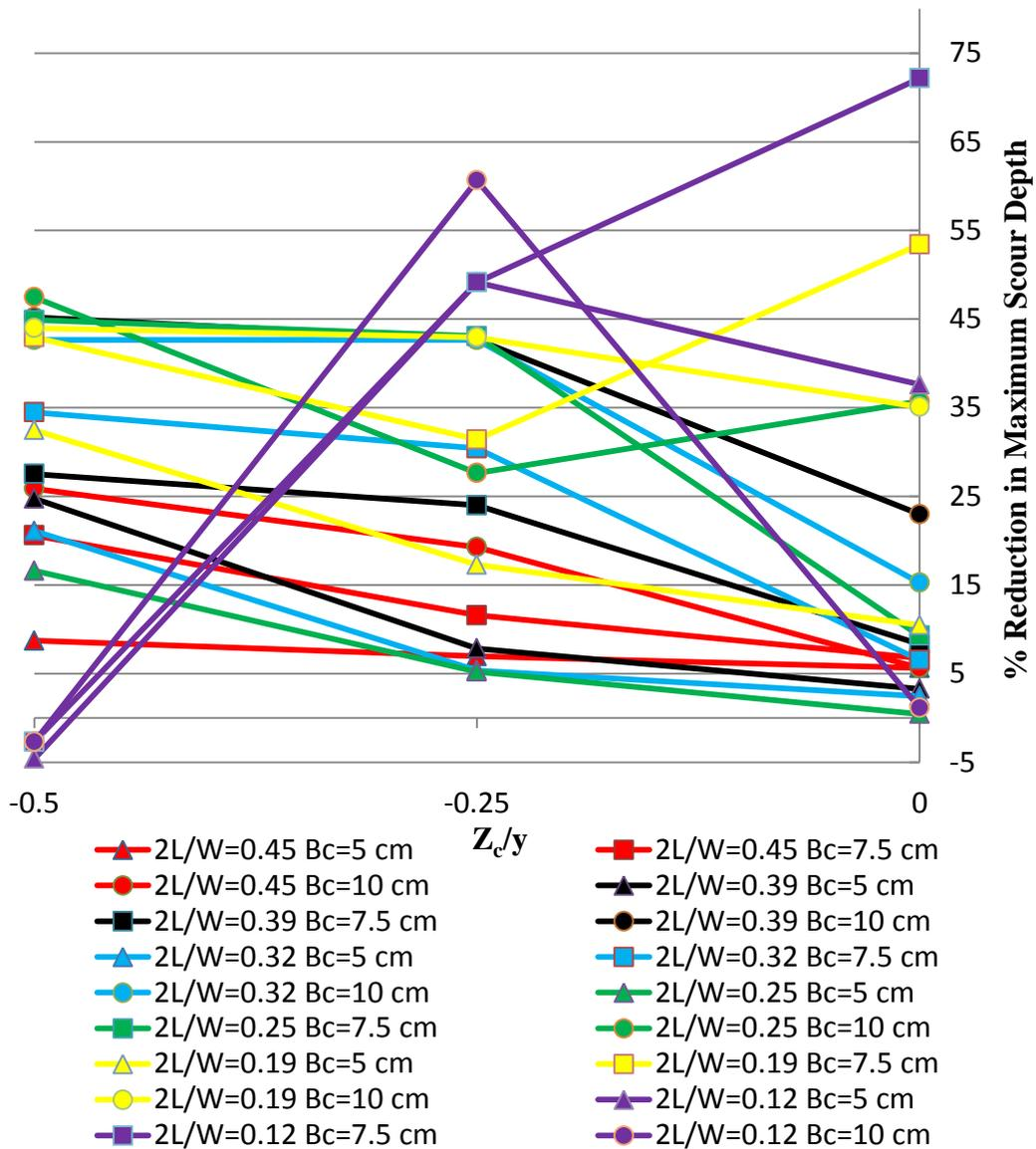
Figure 5-3: Effect of collar size and elevation on the maximum scour depth for abutments with different lengths.
