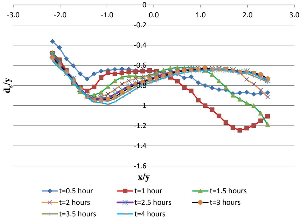
Figure 5-13: Temporal variation of scour hole with collar protection for the contraction ratio of  $2L/W=0.45$  at section I.
