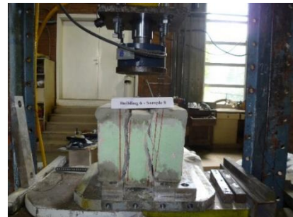
b) Geometric properties and triplet test result of Specimen 2
