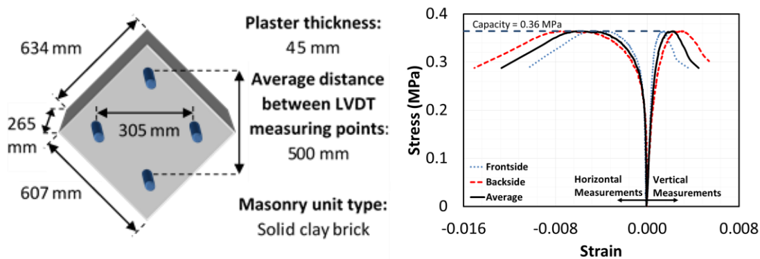
a) Geometric properties and diagonal tension test result of Specimen 1
