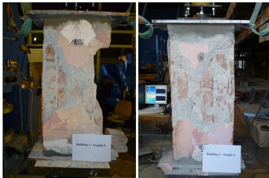
c) Specimen 3 and Specimen 4 at the end of the test
