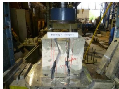
a) Geometric properties and triplet test result of Specimen 1
