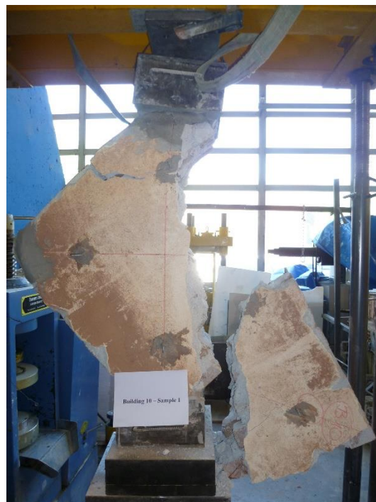
b) Specimen 1 at the end of the test
