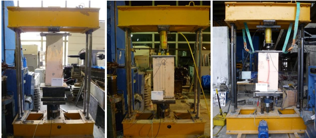
Figure 3.3 Axial compression test setup
