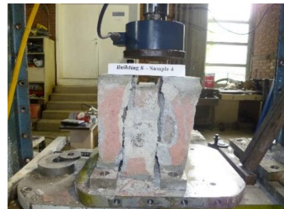
b) Geometric properties and triplet test result of Specimen 2
