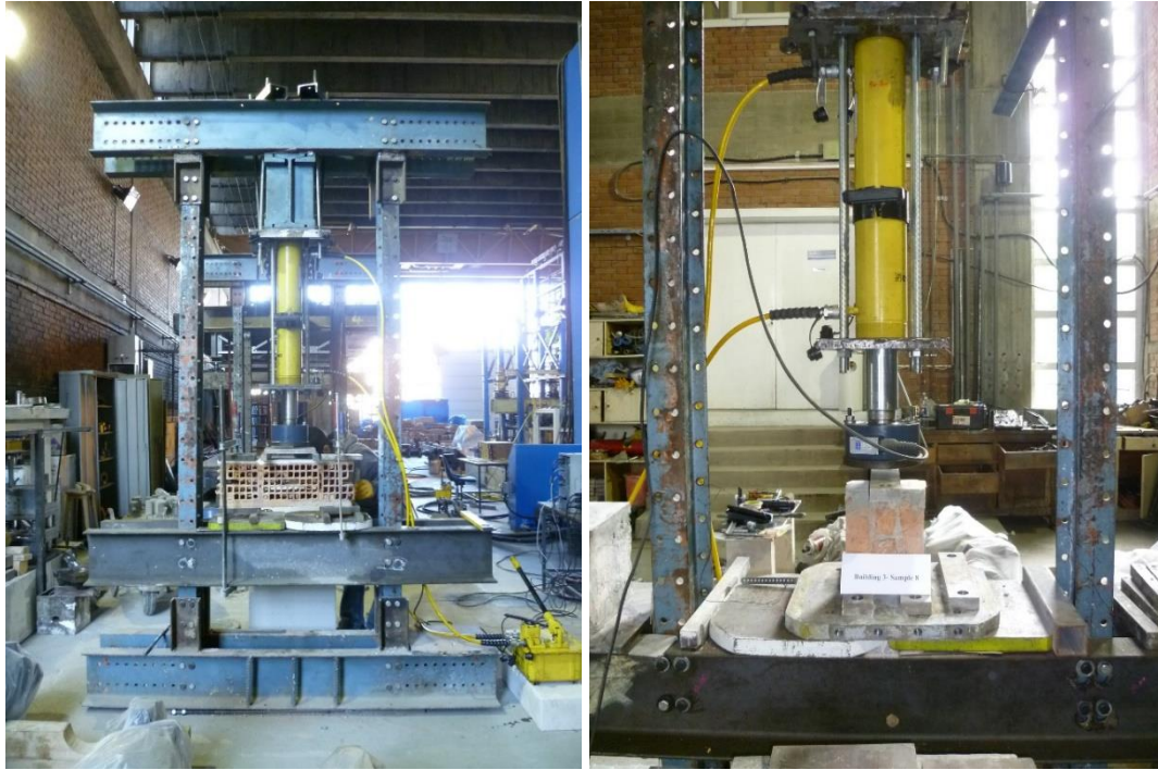
Figure 3.35 Sliding shear test setup
