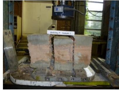
a) Geometric properties and triplet test result of Specimen 1
