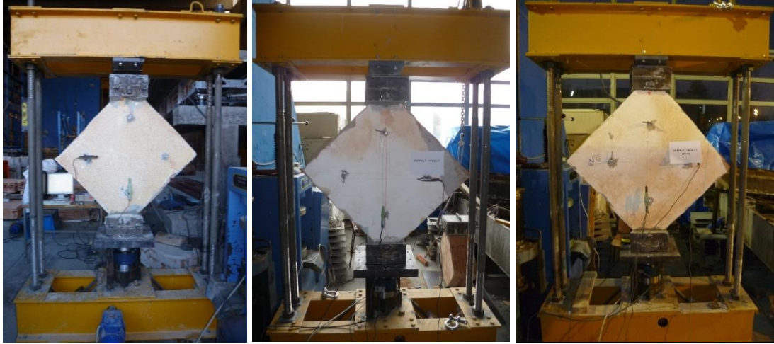
Figure 3.23 Diagonal tension test setup
