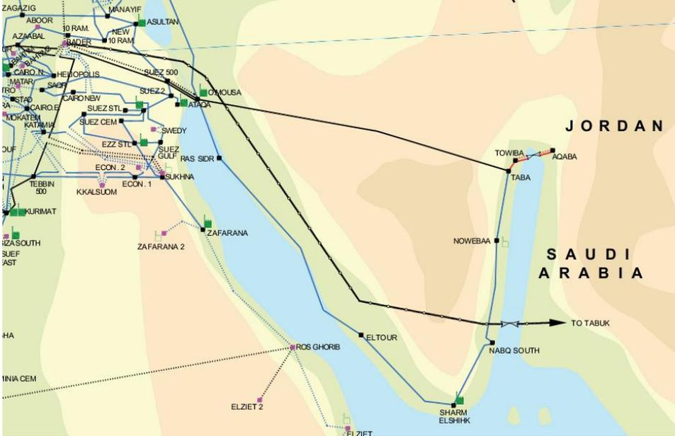
Figure 6 East part of Egyptian transmission network
