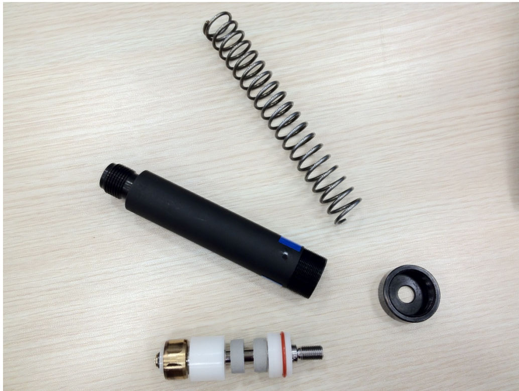
Figure 5-2: Disassembled Off-The-Shelf Shock Absorber
