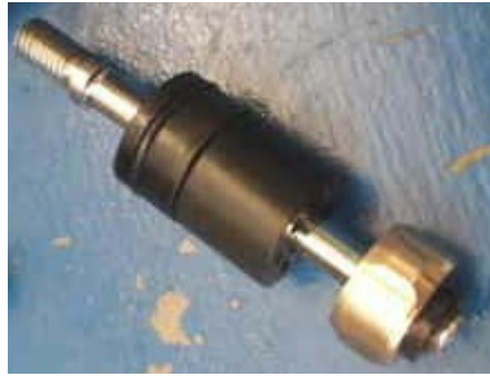
Figure 5-6: Seal Cap Assembly Manufactured from Teflon®
