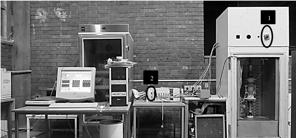
1. In order to supply the TSRST with electricity, turn this button right
