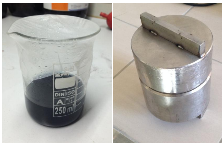
Figure 5-1 : Mixture of Oxalic Acid, Water, NH_4VO_3 and Reactor
