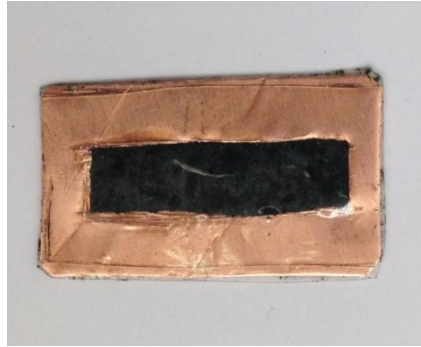
Figure 5-15 : General view of 300 \mu\text{m} copper plate with aperture of 5 mm
