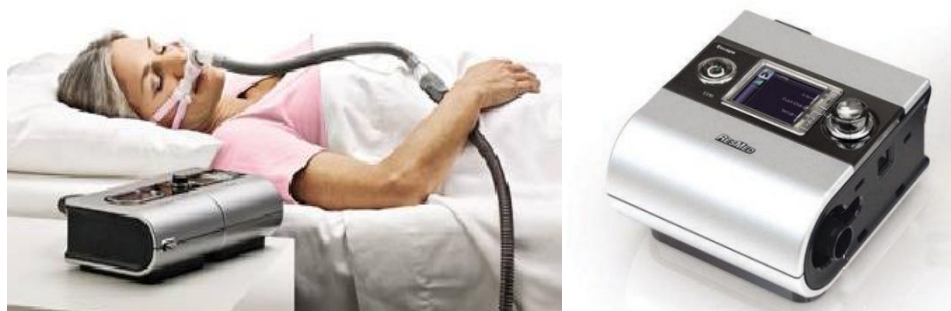
Figure 2.6 ResMed S9 CPAP Device and its usage with an attached humidifier
