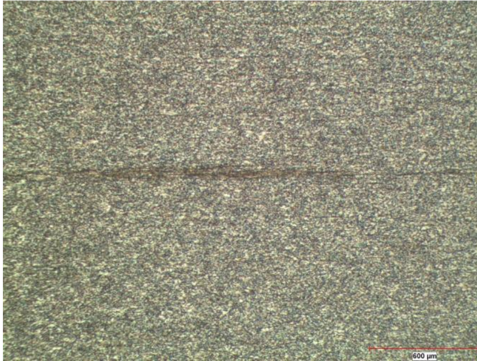
Figure 4.33 X25 Micro Structure of Sample 8 Soft Reduction Ratio is not applied. Casting Speed is 1.15 m/min.
