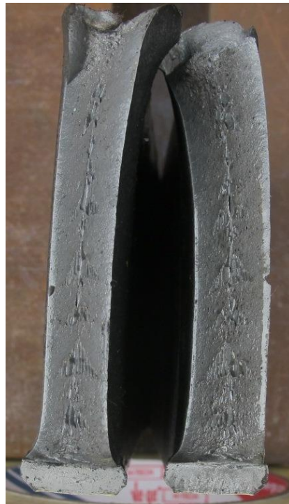
Figure A.10 Sample 10 Soft Reduction is not applied. Casting Speed is 1.17 m/min.
