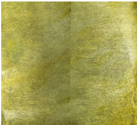
Figure B.3 Macro Sample 4 Side 3 Soft Reduction Ratio is 1 mm/m. Casting Speed is 1.20 m/min.
