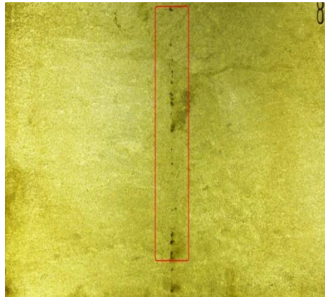
Figure 4.12 Macro Sample 6 Side 4 Soft Reduction Ratio is 1 mm/m. Casting Speed is 1.15 m/min.
