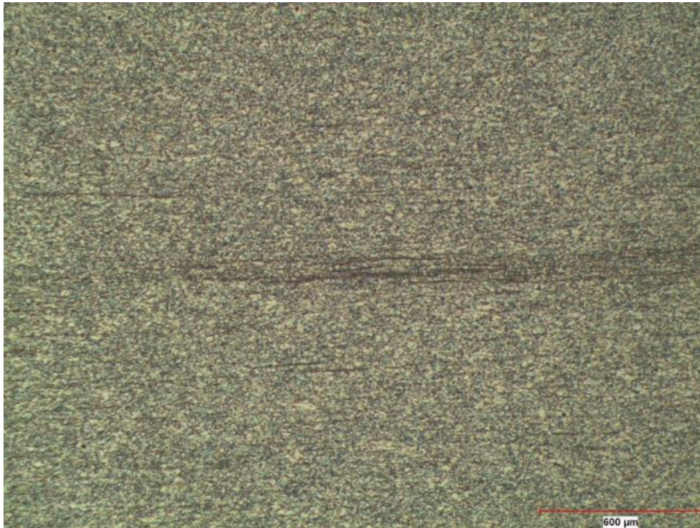
Figure 4.29 X25 Micro Structure of Sample 6 Soft Reduction Ratio is 1 mm/m. Casting Speed is 1.15 m/min.
