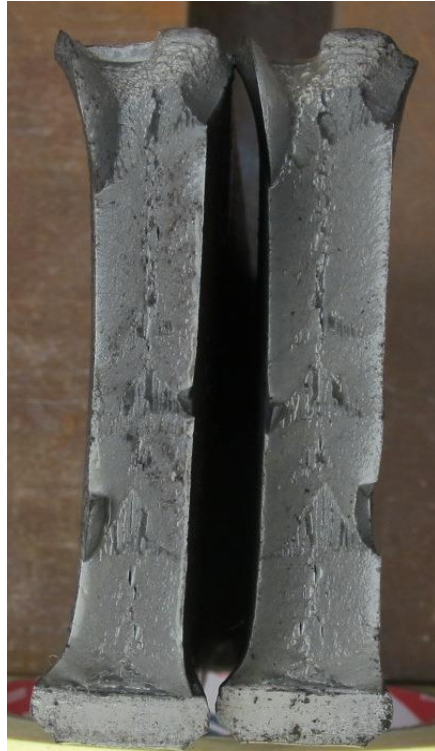
Figure A.11 Sample 11 Soft Reduction is not applied. Casting Speed is 1.15 m/min.
