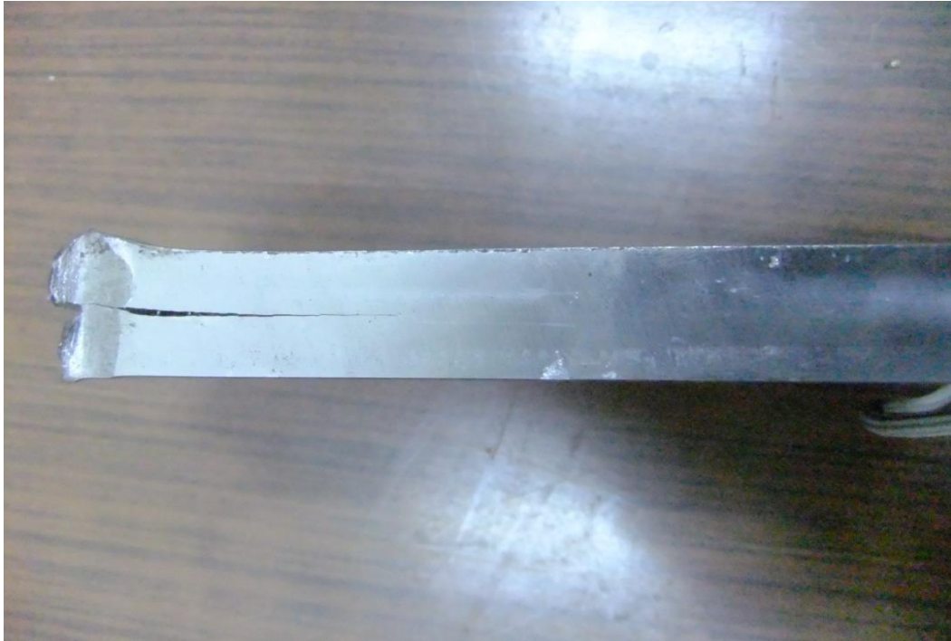
Figure 2.3 X70 Steel Grade DWT Testing Sample Crack goes along the pearlite-ferrite band.
