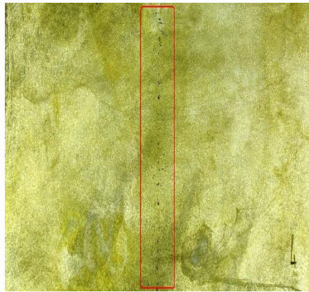
Figure B.8 Macro Sample 9 Side 4 Soft Reduction Ratio is 1.20 mm/m. Casting Speed is 1.15 m/min.
