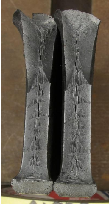
Figure A.3 Sample 3 Soft Reduction Ratio is 1 mm/m. Casting Speed is 1.20 m/min.
