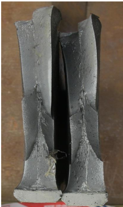
Figure A.9 Sample 9 Soft Reduction Ratio is 1.20 mm/m. Casting Speed is 1.15 m/min.
