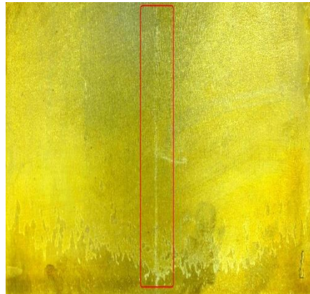
Figure B.2 Macro Sample 2 Side 4 Soft Reduction Ratio is 1 mm/m. Casting Speed is 1.05 m/min.
