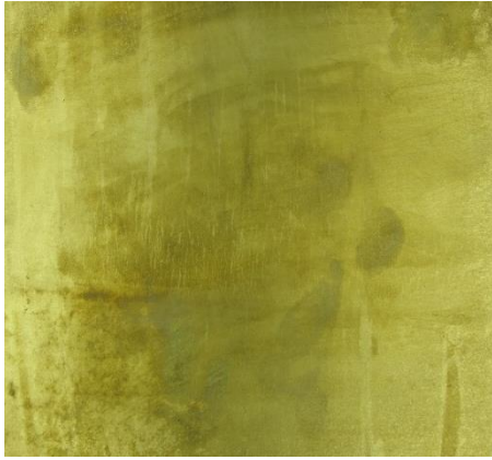
Figure B.5 Macro Sample 5 Side 3 Soft Reduction Ratio is 1 mm/m. Casting Speed is 1.20 m/min.
