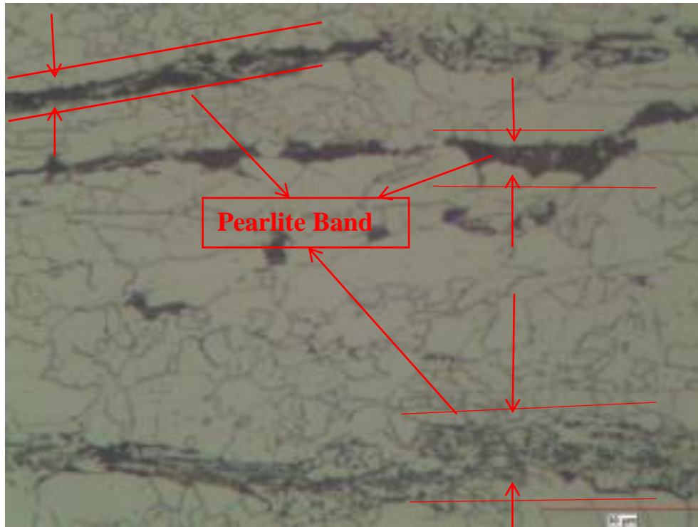
Figure 4.26 X500 Micro Structure of Sample 4 Soft Reduction Ratio is 1 mm/m. Casting Speed is 1.20 m/min. The arrows show where the thickness is measured.
