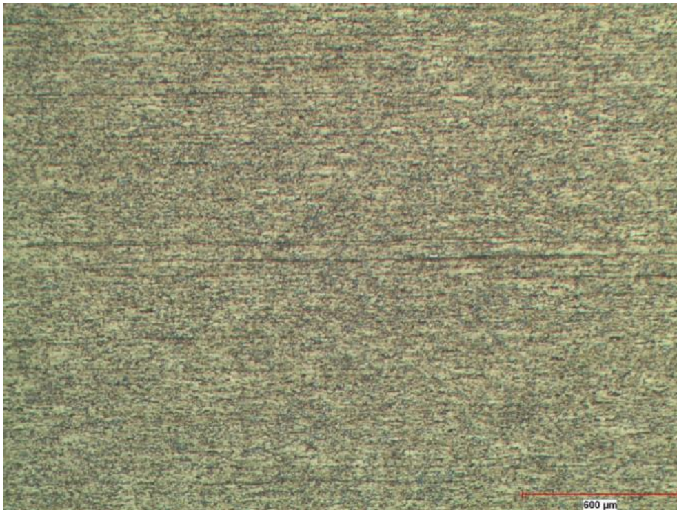
Figure 4.25 X25 Micro Structure of Sample 4 Soft Reduction Ratio is 1 mm/m. Casting Speed is 1.20 m/min.
