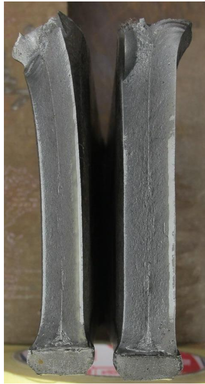
Figure A.8 Sample 8 Soft Reduction is not applied. Casting Speed is 1.15 m/min.
