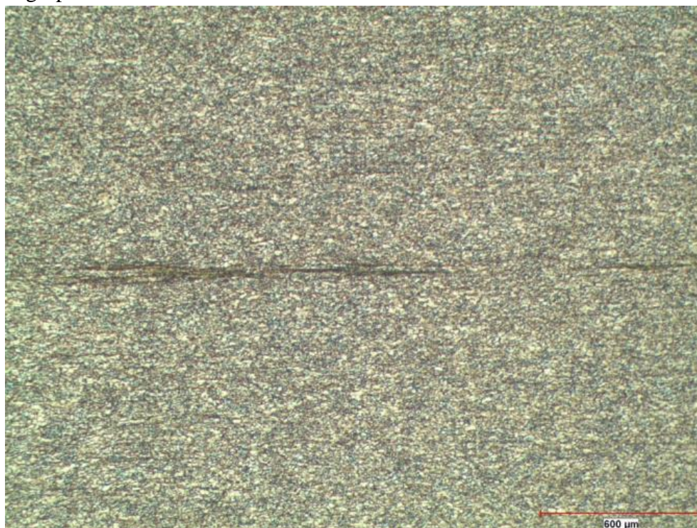
Figure 4.31 X25 Micro Structure of Sample 7 Soft Reduction Ratio is 1.10 mm/m. Casting Speed is 1.15 m/min.
