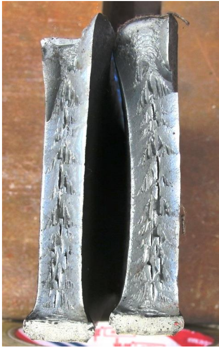
Figure A.1 Sample 1 Soft Reduction Ratio is 1 mm/m. Casting Speed is 1.15 m/min.
