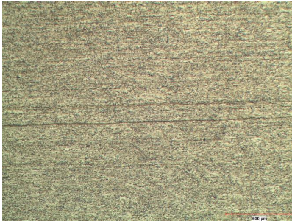
Figure 4.27 X25 Micro Structure of Sample 5 Soft Reduction Ratio is 1 mm/m. Casting Speed is 1.20 m/min.
