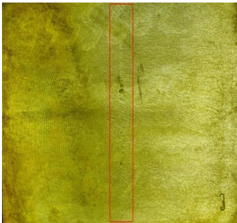
Figure 4.7 Macro Sample 1 Side 3 Soft Reduction Ratio is 1 mm/m. Casting Speed is 1.15 m/min.
