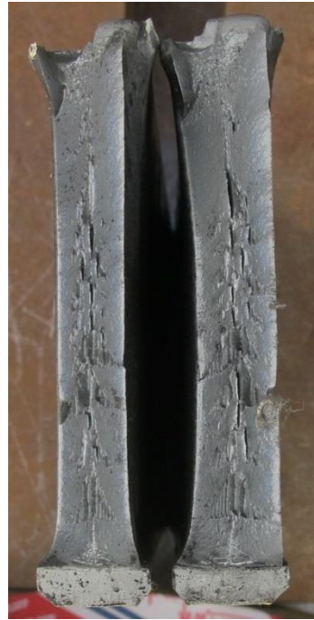
Figure A.2 Sample 2 Soft Reduction Ratio is 1 mm/m. Casting Speed is 1.05 m/min.
