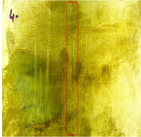
Figure 4.10 Macro Sample 3 Side 4 Soft Reduction Ratio is 1 mm/m. Casting Speed is 1.20 m/min.
