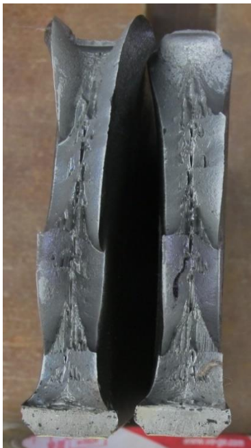
Figure A.5 Sample 5 Soft Reduction Ratio is 1 mm/m. Casting Speed is 1.20 m/min.
