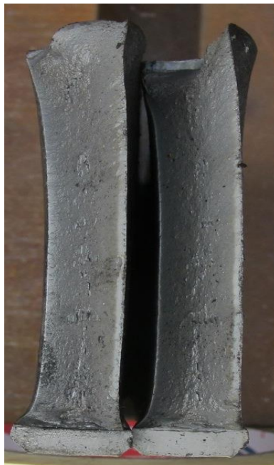
Figure A.6 Sample 6 Soft Reduction Ratio is 1 mm/m. Casting Speed is 1.15 m/min.
