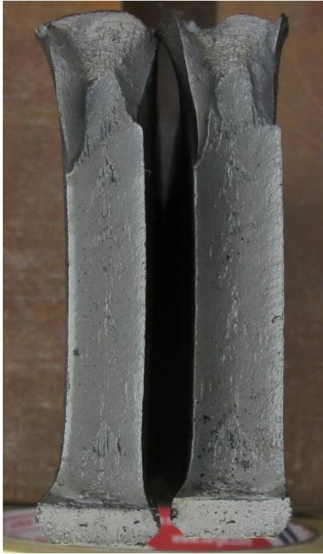
Figure A.7 Sample 7 Soft Reduction Ratio is 1.10 mm/m. Casting Speed is 1.15 m/min.
