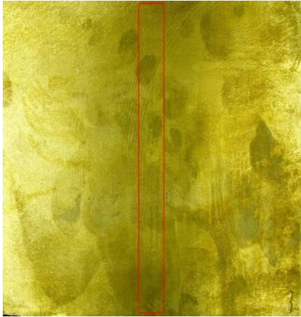
Figure 4.9 Macro Sample 3 Side 3 Soft Reduction Ratio is 1 mm/m Casting Speed is 1.20 m/min.
