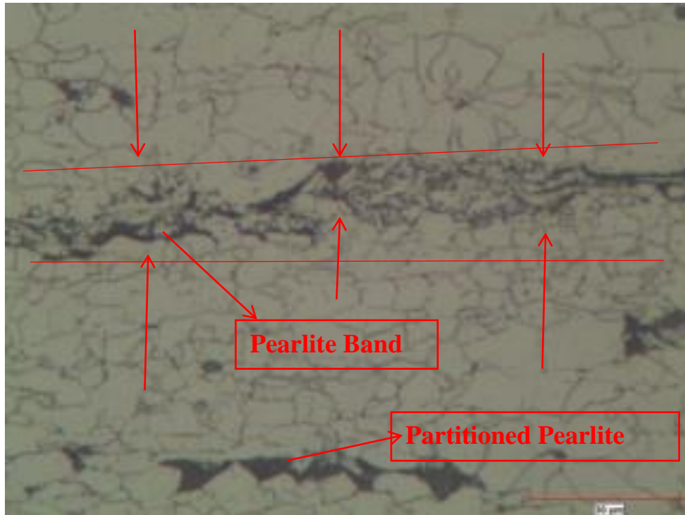
Figure 4.28 X500 Micro Structure of Sample 5 Soft Reduction Ratio is 1 mm/m. Casting Speed is 1.20 m/min. The arrows show where the thickness is measured.
