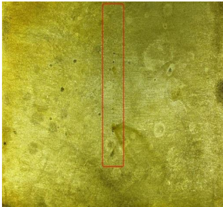
Figure 4.11 Macro Sample 6 Side 3 Soft Reduction Ratio is 1 mm/m. Casting Speed is 1.15 m/min.
