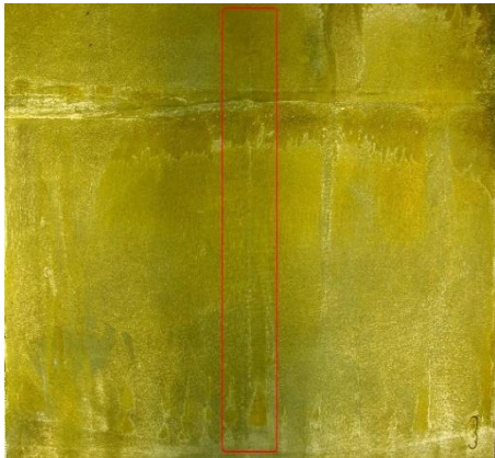
Figure B.1 Macro Sample 2 Side 3 Soft Reduction Ratio is 1 mm/m. Casting Speed is 1.05 m/min.
