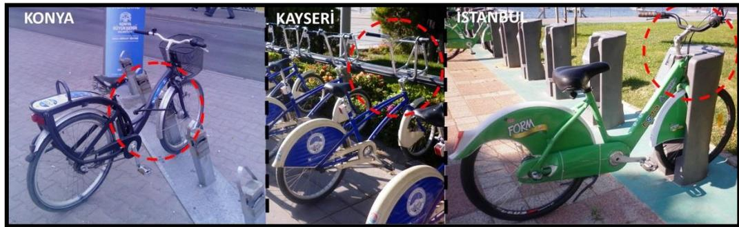
**Figure 52. Locking Mechanisms of Konya, Kayseri and İstanbul Bike-sharing Systems**
