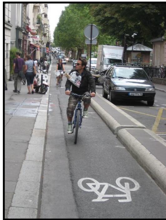
**Figure 5. Segregated Bike Lane from Road Traffic near to sidewalk in Paris**
