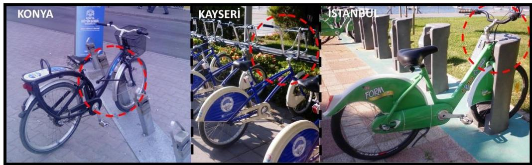
**Figure 52. Locking Mechanisms of Konya, Kayseri and İstanbul Bike-sharing Systems**
