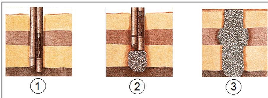
Figure 2.1 Construction phases of a dry bottom feed stone column (adopted from <http://www.vibroflotation.com>)
