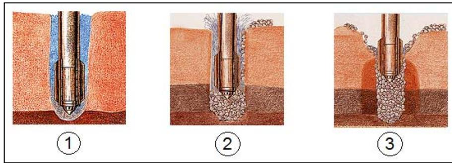
Figure 2.4 Construction phases of a wet top feed stone column (adopted from <http://www.vibroflotation.com>)
