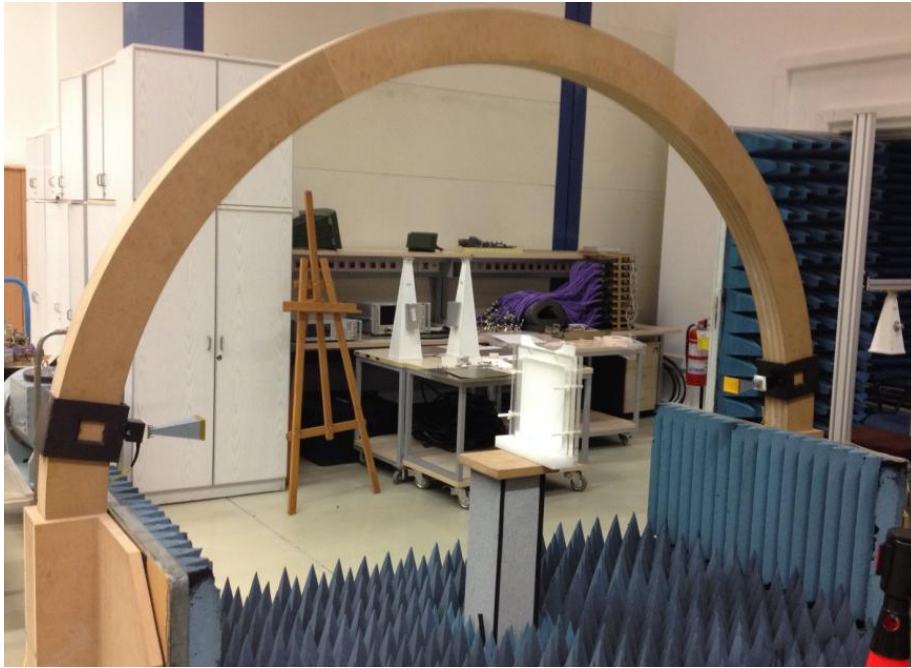
Figure 5- 6 Modified horn antenna measurement setup
