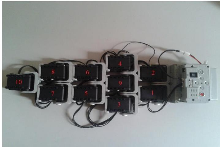
Figure 5.7: Reconfigured Exoskeleton Structure
