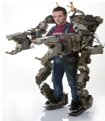
Figure 2.5: Body Extender (Marchesci et. al.,2011)
