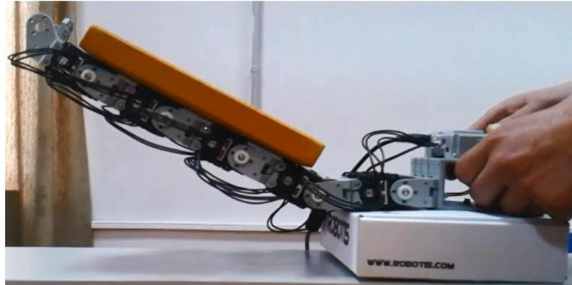
Figure 5.2: Exoskeleton with 400gr load
