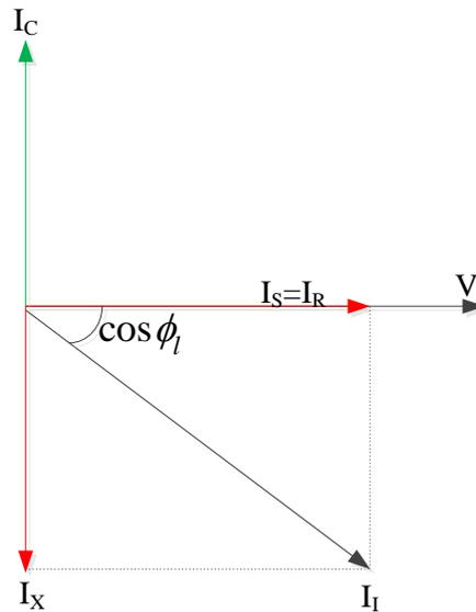
**Figure 2.7:** Load, compensator and supply side current components
