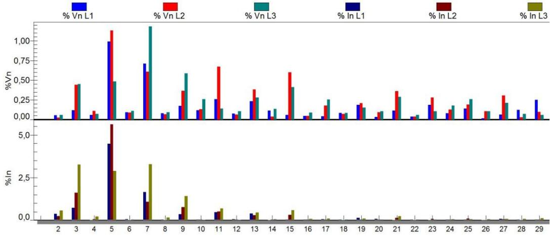
**Figure 5.16:** Current / voltage harmonics for unbalance of 120<sup>o</sup>-130<sup>o</sup>-140<sup>o</sup> in RS-ST-TR phases (field data)
