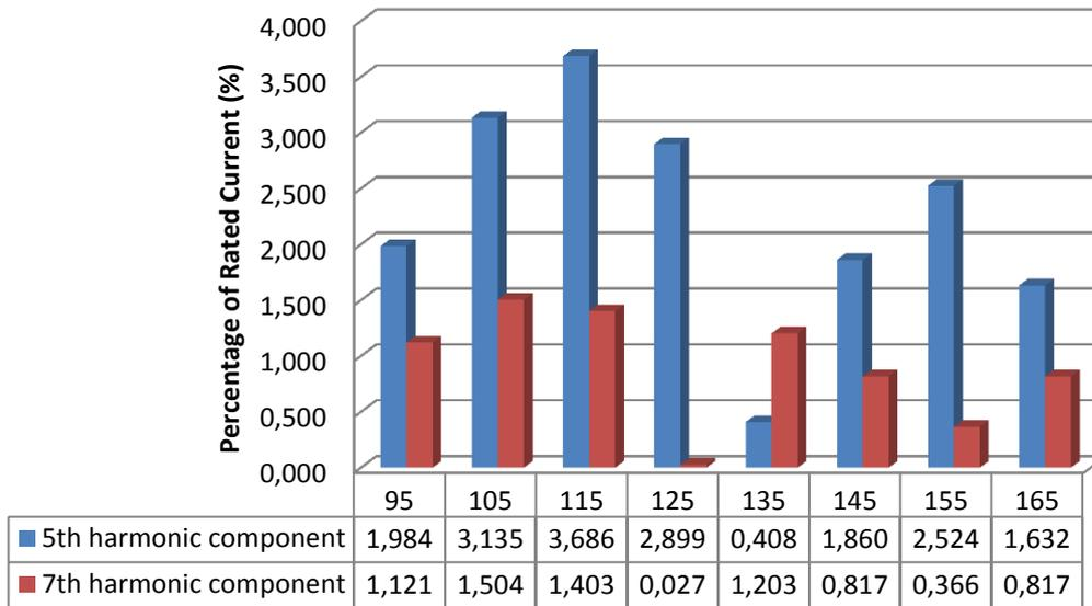
**Figure 5.13:** 5<sup>th</sup> - 7<sup>th</sup> harmonic currents versus firing angle relationship (field data)
