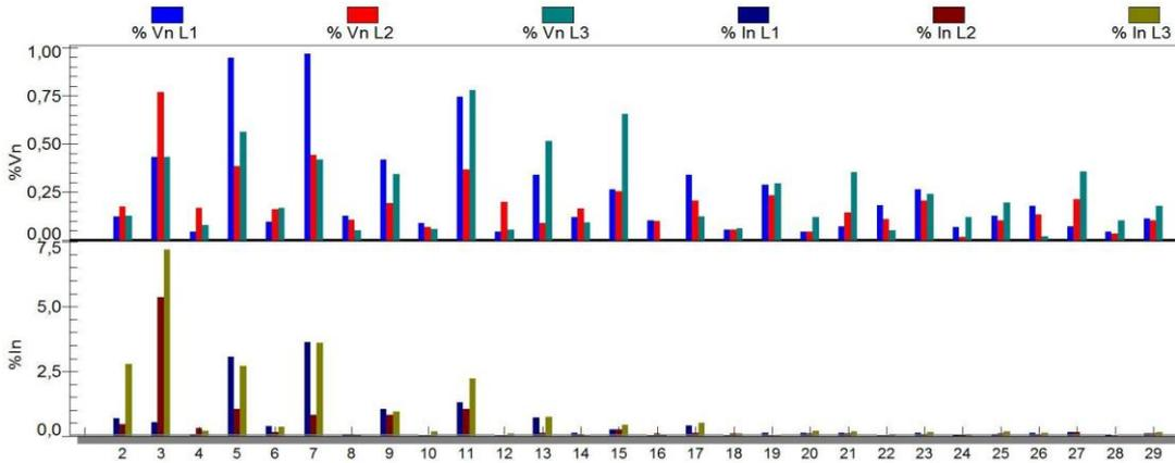
**Figure 5.18:** Current / voltage harmonics at PCC with 500kVAr sequential limit (field data)
