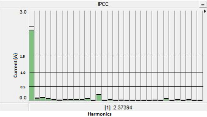
Figure 4.24: Current harmonics at PCC with equal load sharing (simulation)
