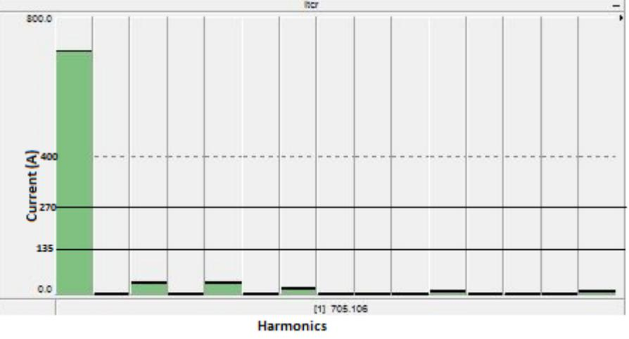
**Figure 4.21:** Harmonic currents going out of delta for unbalanced operation (simulation)
