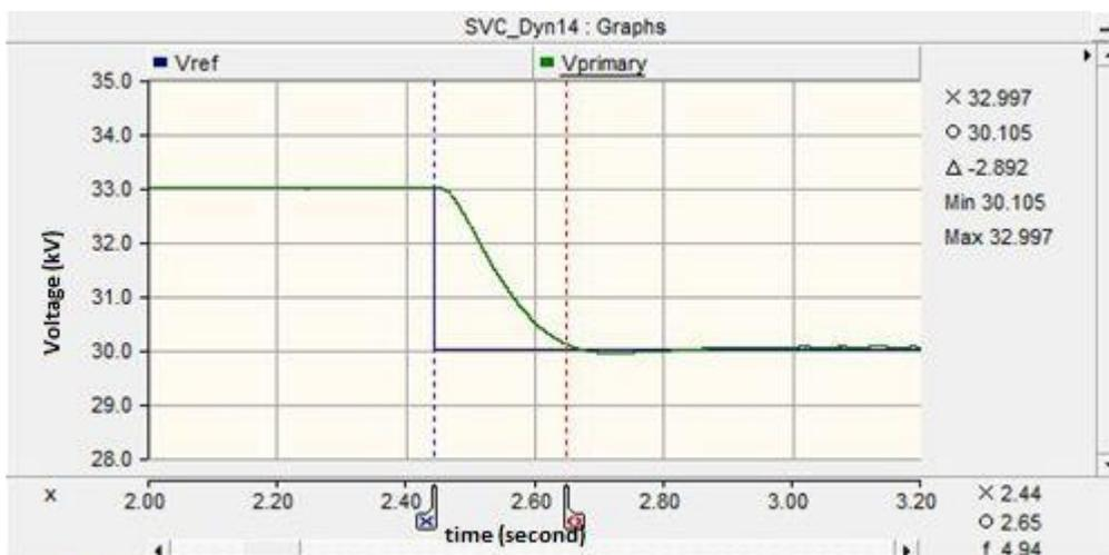
**Figure 4.13:** Over-damped response curve from 33kV to 30kV (simulation)
