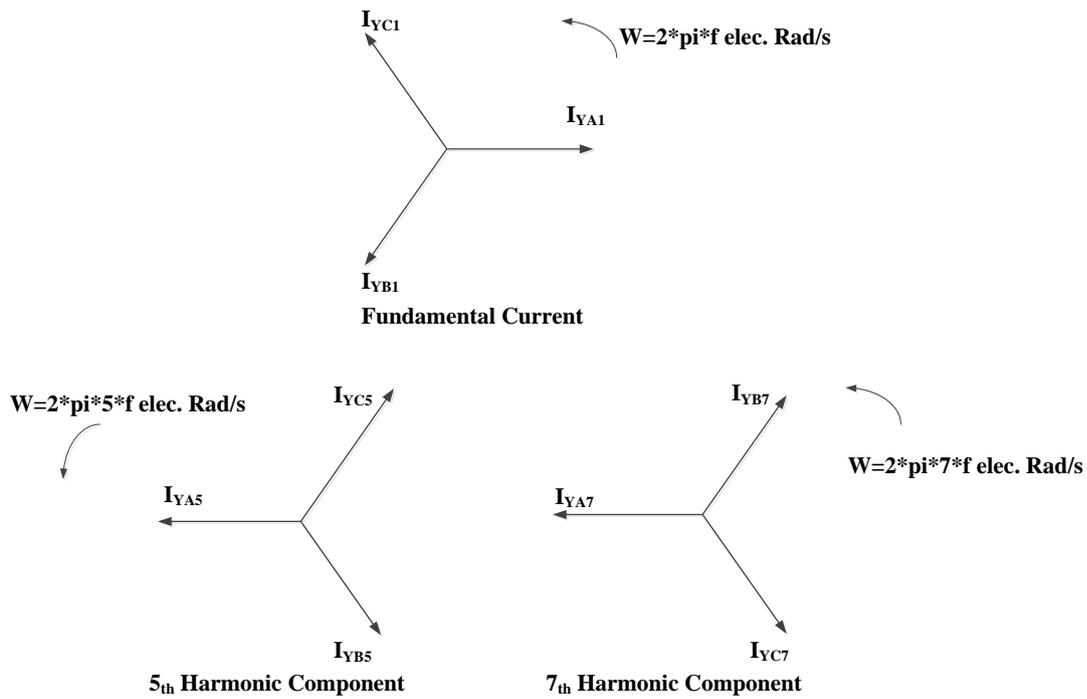
**Figure 2.15:** Transformer primary current components in Y-Y connection
