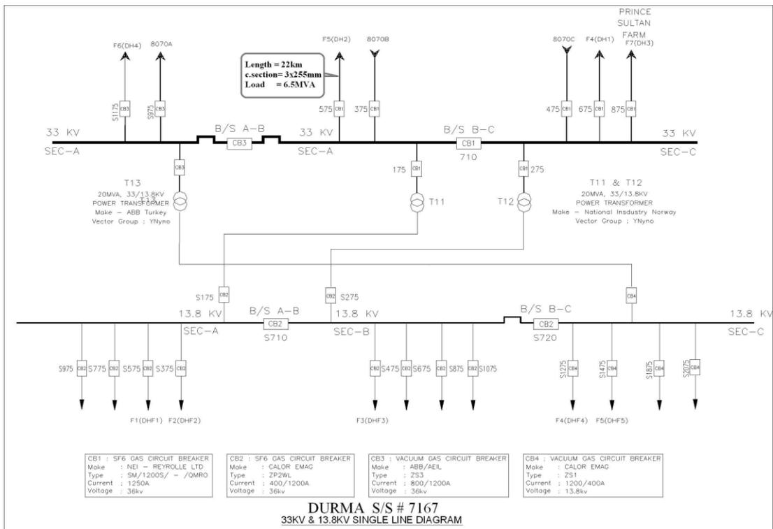
**Figure 3.5: Single line diagram of Dhurma power distribution system**
