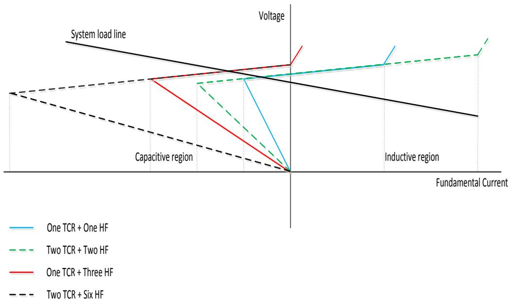
**Figure 4.3:** *I-V Characteristics of SVC system with different topologies*
