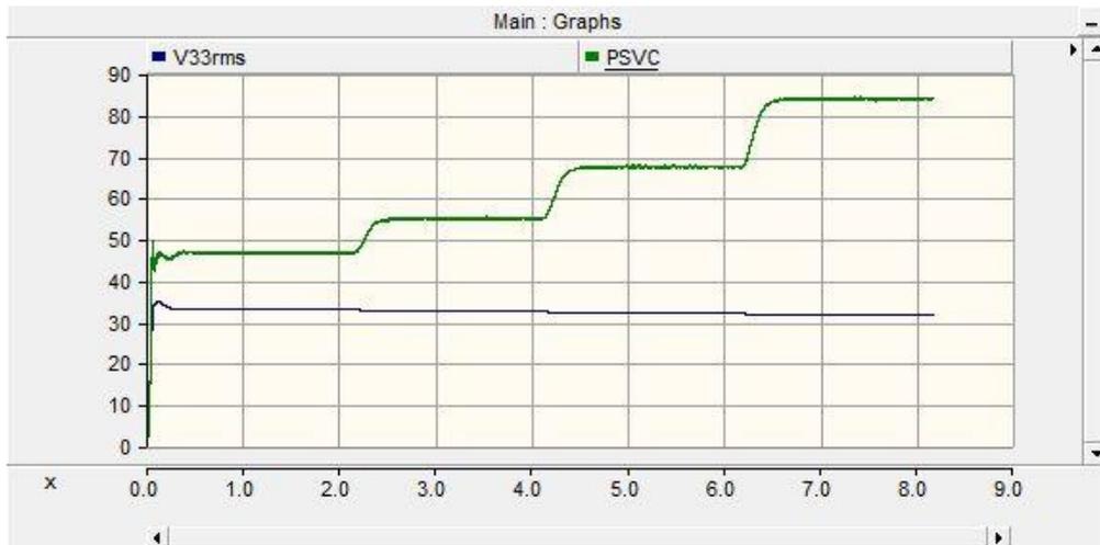
**Figure 4.28:** Total Losses under equal load sharing mode of operation (simulation)
