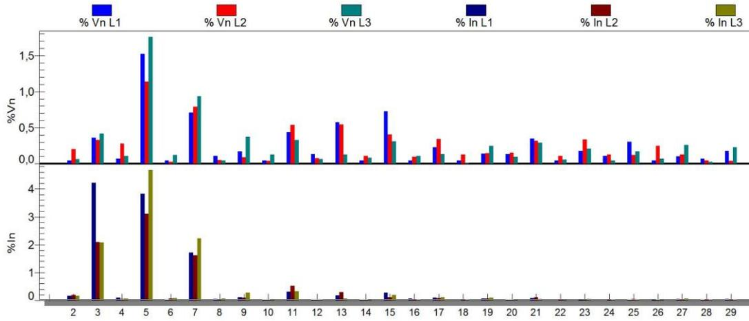
**Figure 5.15:** Current / voltage harmonics for unbalance of 95<sup>o</sup>-100<sup>o</sup>-105<sup>o</sup> in RS-ST-TR phases (field data)
