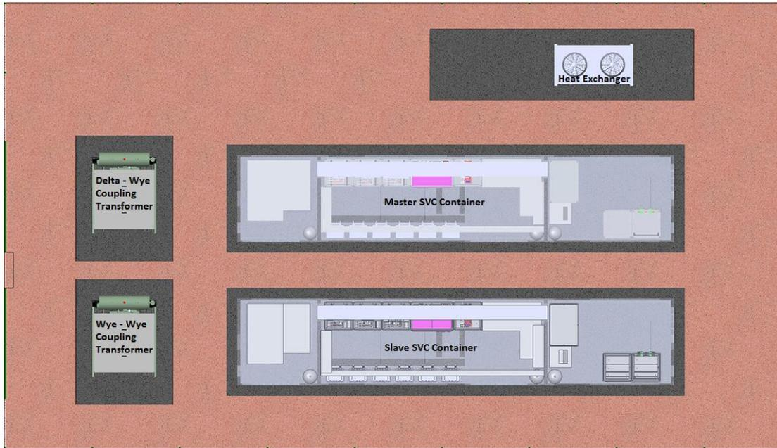
**Figure 3.8:** Platform design of SVC systems
