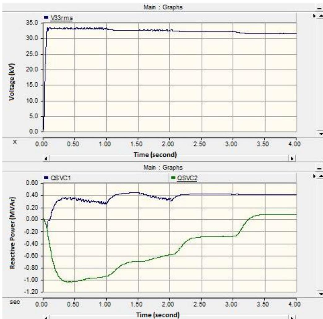
**Figure 4.6:** Load sharing for independent operation showing asymmetrical operation and oscillations (simulation)
