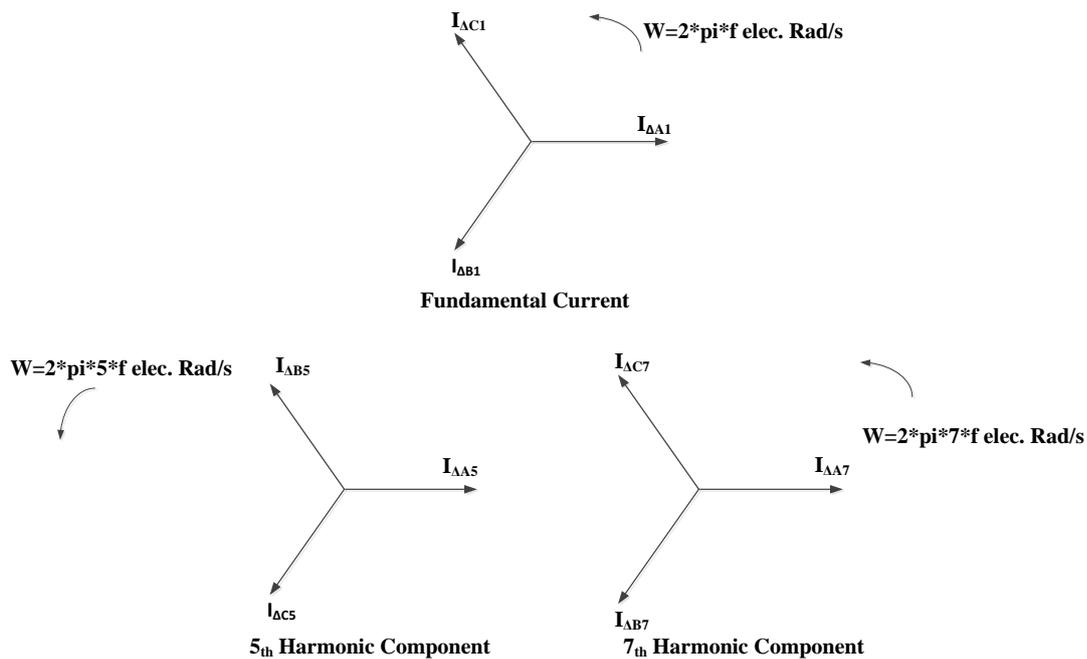
**Figure 2.16:** Transformer primary current components in Y- $\Delta$  connection
