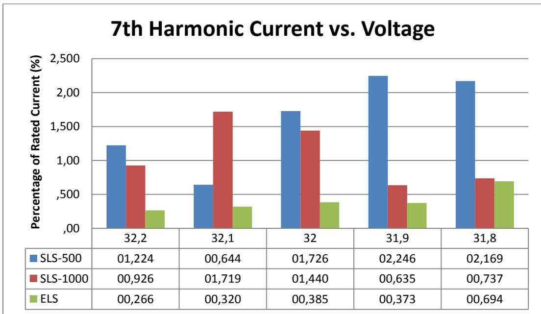
**Figure 5.24:** 7<sup>th</sup> harmonic current as percentage of rated current for different voltage levels and control algorithms (field data)
