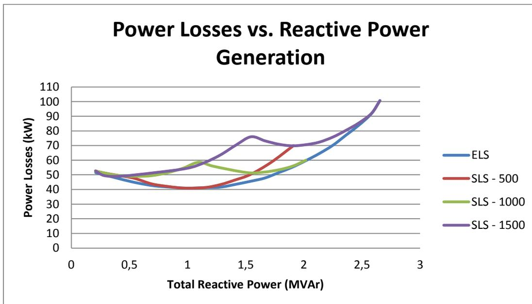
**Figure 4.30:** Power losses according to total reactive power generation (simulation)
