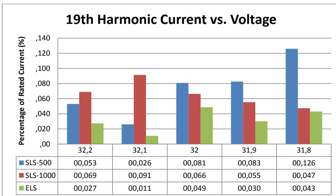
**Figure 5.26:** 19<sup>th</sup> harmonic current as percentage of rated current for different voltage levels and control algorithms (field data)
