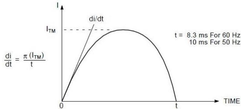
**Figure 3.11:** Rate of rise of current for surge condition [14]
