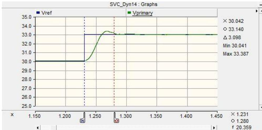
**Figure 4.16:** Critically damped response curve from 33kV to 30kV (simulation)
