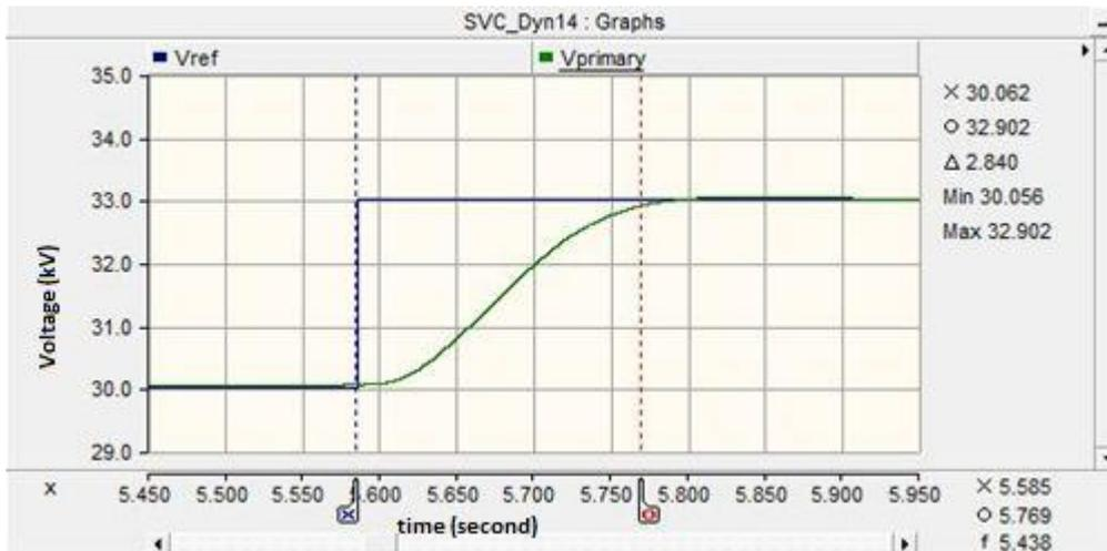
**Figure 4.12:** Over-damped response curve from 30kV to 33kV (simulation)
