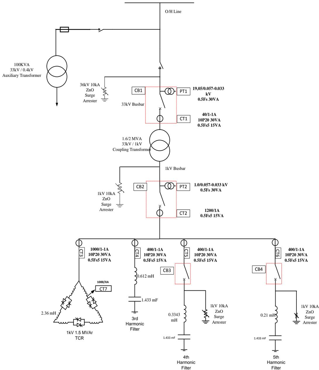
**Figure 3.7:** Single line diagram of the developed system, only the 6-pulse master SVC shown, slave SVC power system topology is also exactly the same
