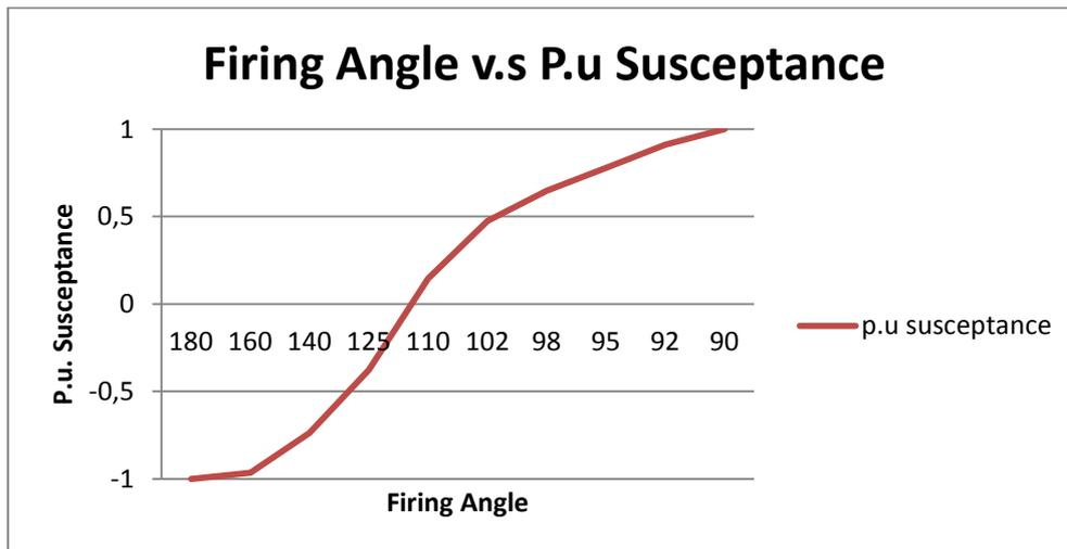
Figure 4.9: Susceptance / Firing angle conversion graph
