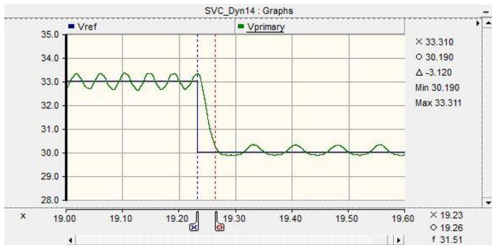
**Figure 4.15:** Under-damped (and oscillatory) response curve from 33kV to 30kV due to improper parameter settings (simulation)
