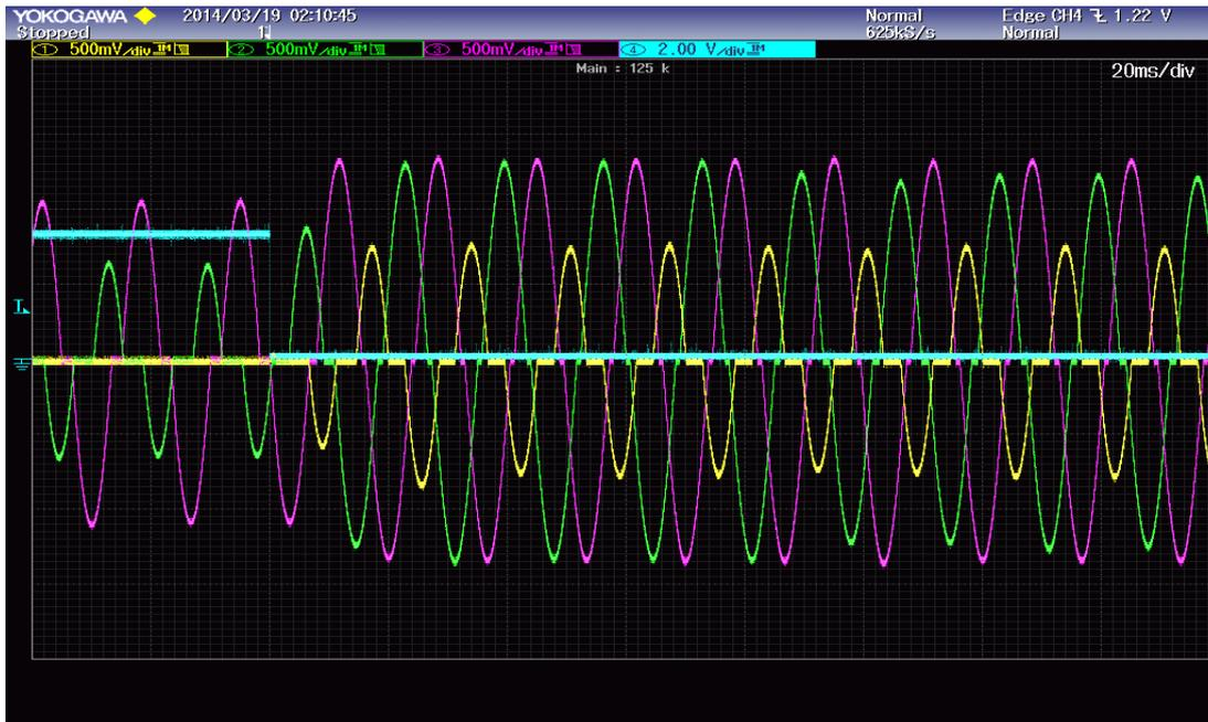
**Figure 5.31:** *Transient response from 33kV to 32.5kV*
