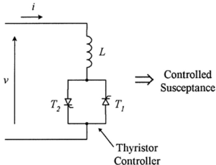
**Figure 2.1:** Thyristor controlled reactor
