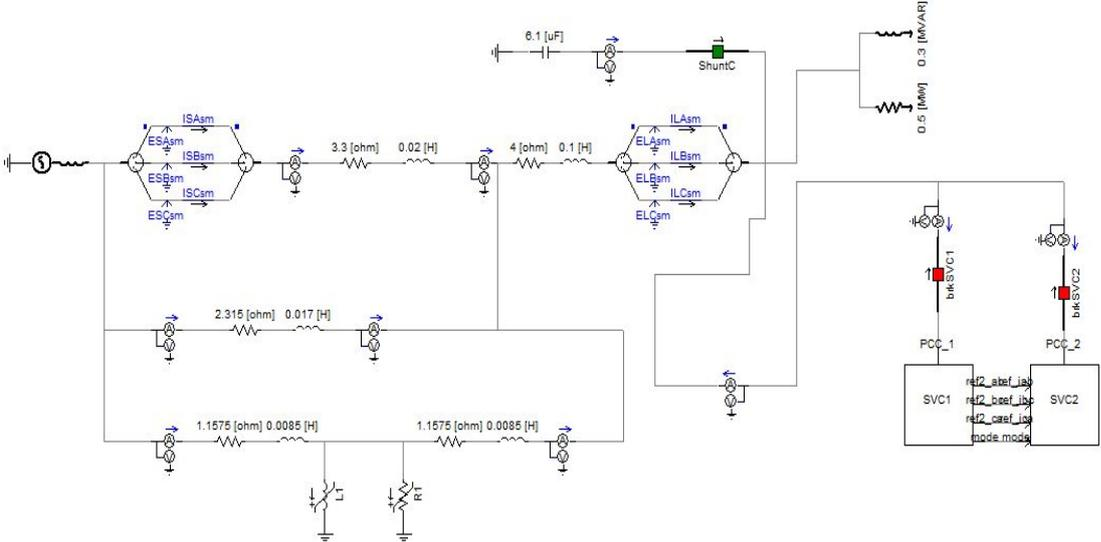
**Figure 3.6:** Single line diagram of simulated electricity system with two SVC systems
