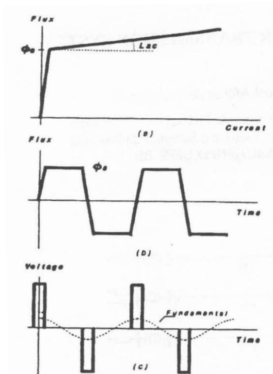
Figure 1.2: Core characteristics of saturated reactor [3]
