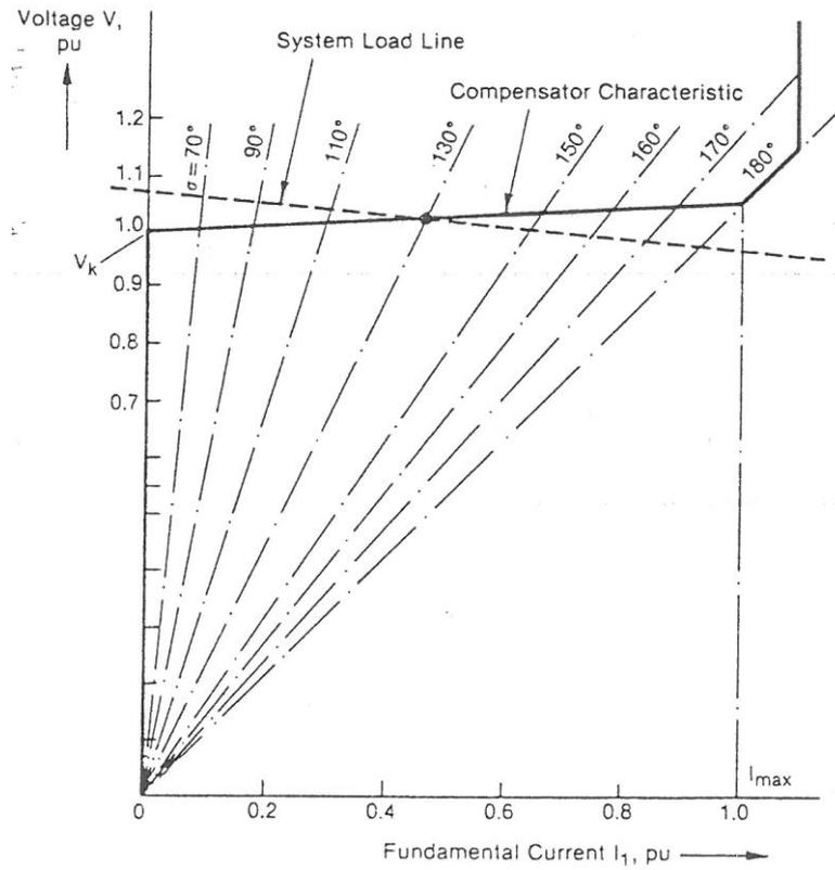
**Figure 2.10:** Formation of fundamental voltage / current characteristics in the TCR compensator [1]
