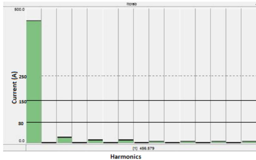
**Figure 4.18:** Harmonic currents inside delta for balanced operation (simulation)
