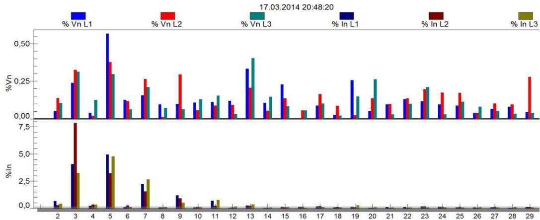
**Figure 5.19:** Current / voltage harmonics at primary side of master with 1MVAR sequential limit (field data)
