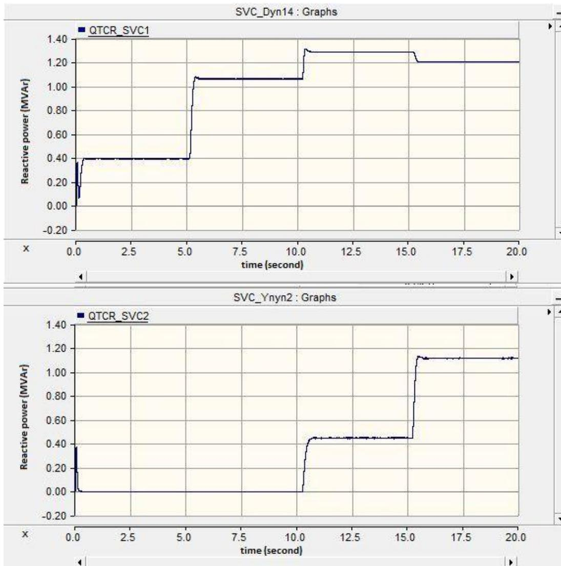
**Figure 4.11:** Variation in reactive power generations of two TCR systems (simulation)
