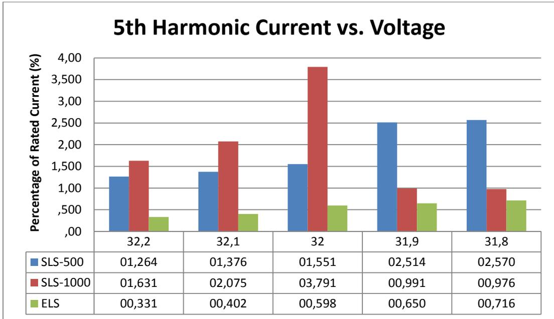
**Figure 5.23:** 5<sup>th</sup> harmonic current as percentage of rated current for different voltage levels and control algorithms (field data)
