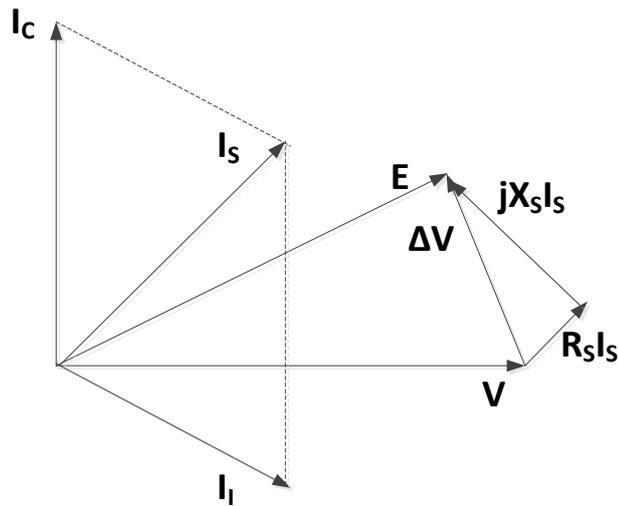
**Figure 2.12:** *Compensated load voltage regulation*
