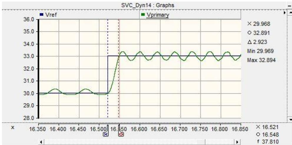
**Figure 4.14:** Under-damped (and oscillatory) response curve from 30kV to 33kV due to improper parameter settings (simulation)
