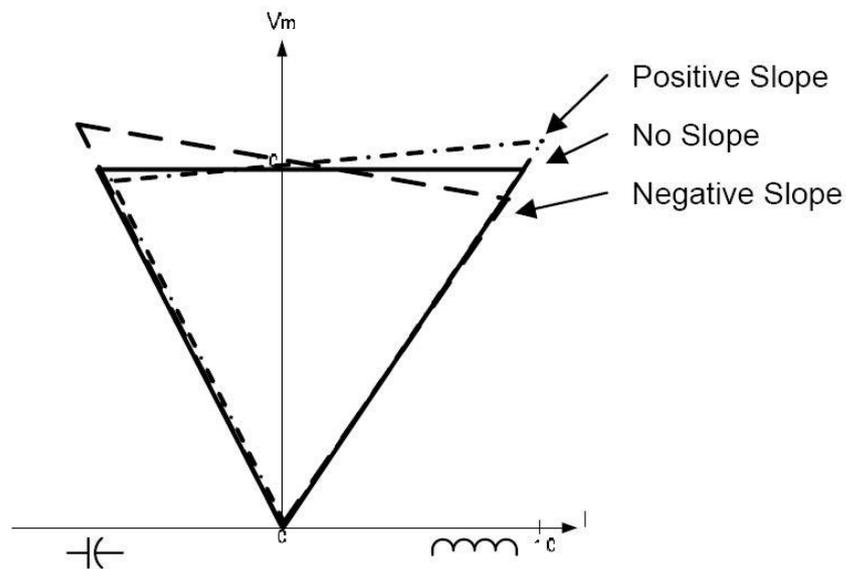
**Figure 4.3:** Slope effect on SVC characteristics
