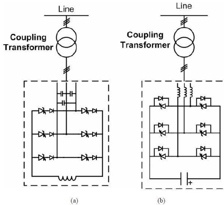
**Figure 1.5:** STATCOM based on (a) Current source converter (CSC) and (b) Voltage source converter (VSC) [4]
