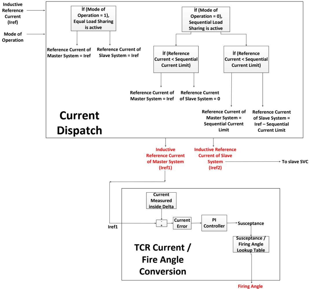
Figure 4.8: Current Dispatch and Firing angle conversion block
