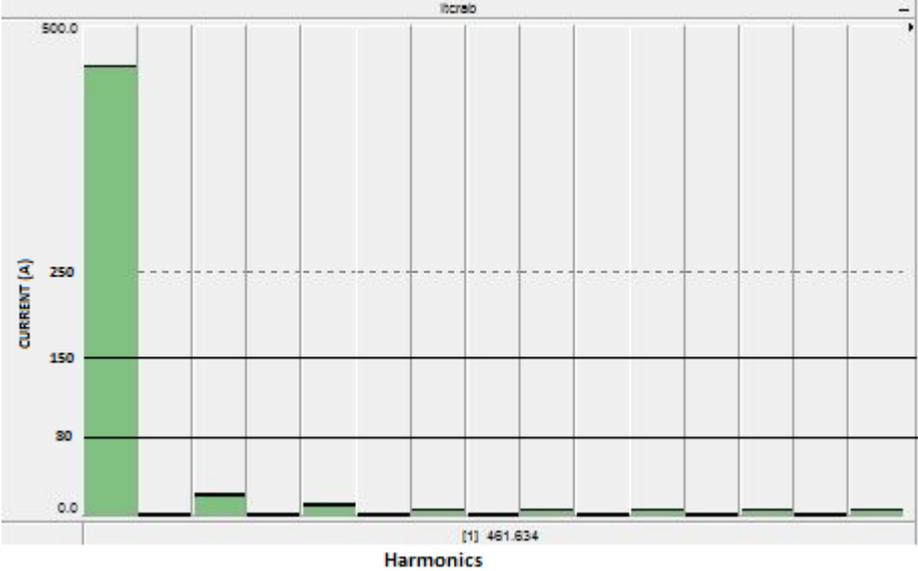
**Figure 4.20:** Harmonic currents inside delta for unbalanced operation (simulation)
