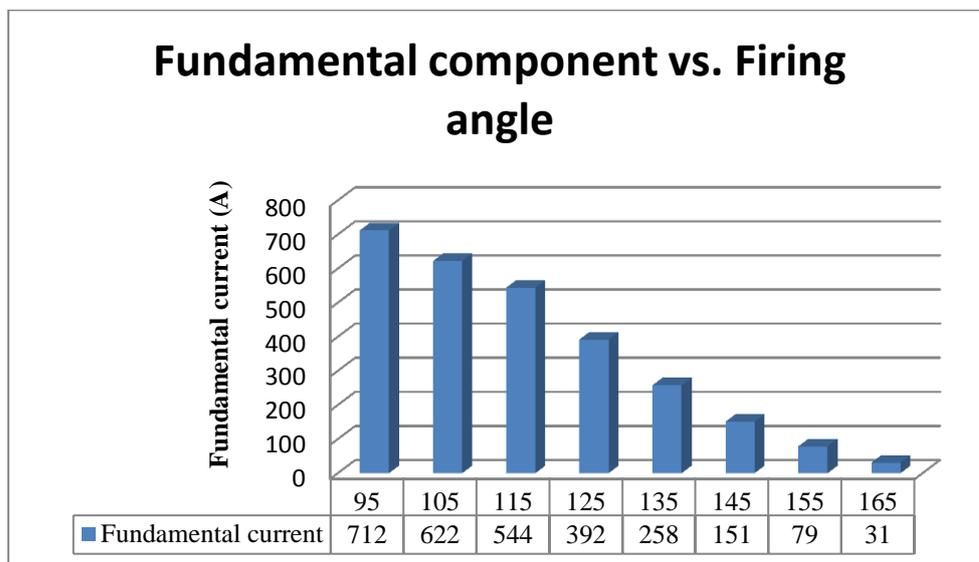
**Figure 5.11:** TCR fundamental current (line) versus firing angle relationship (field data)
