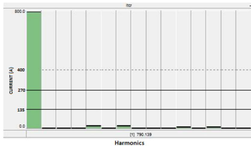
**Figure 4.19:** Harmonic currents going out of delta for balanced operation (simulation)
