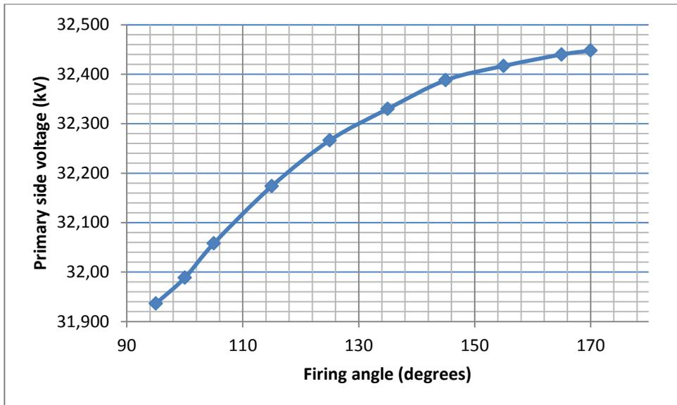
**Figure 5.10:** Voltage versus firing angle relationship with one filter only (field data)
