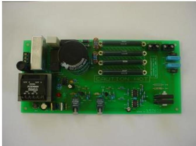
**Figure 3.12:** *Dynex gate driver circuitry*
