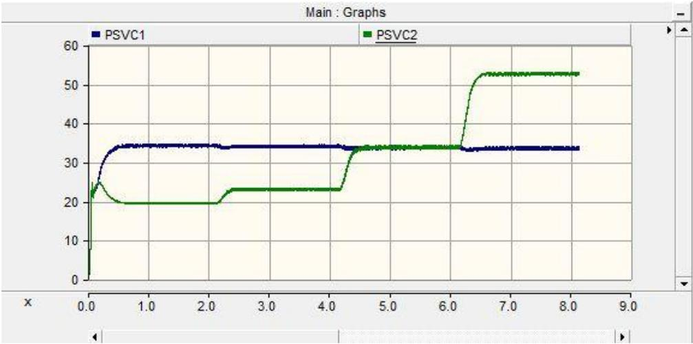
**Figure 4.26:** Losses for each system under sequential load sharing mode of operation (simulation)
