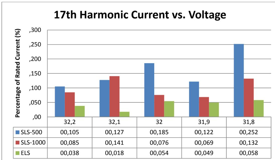
**Figure 5.25:** 17<sup>th</sup> harmonic current as percentage of rated current for different voltage levels and control algorithms (field data)
