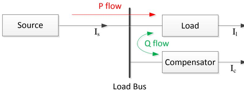
**Figure 2.6:** Reactive power compensation of the load
