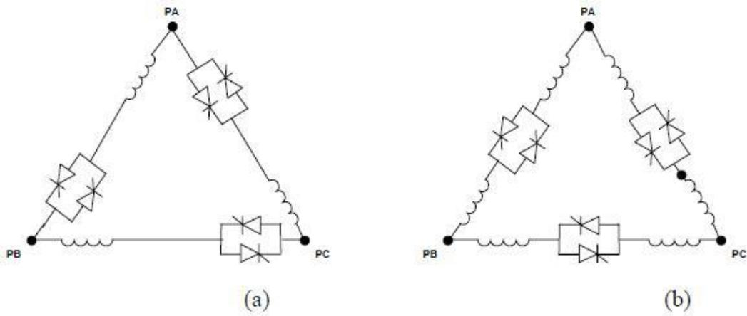
**Figure 3.13:** Reactor alignments, a) single piece, b) two pieces
