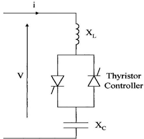
**Figure 1.3:** *Thyristor switched capacitor*
