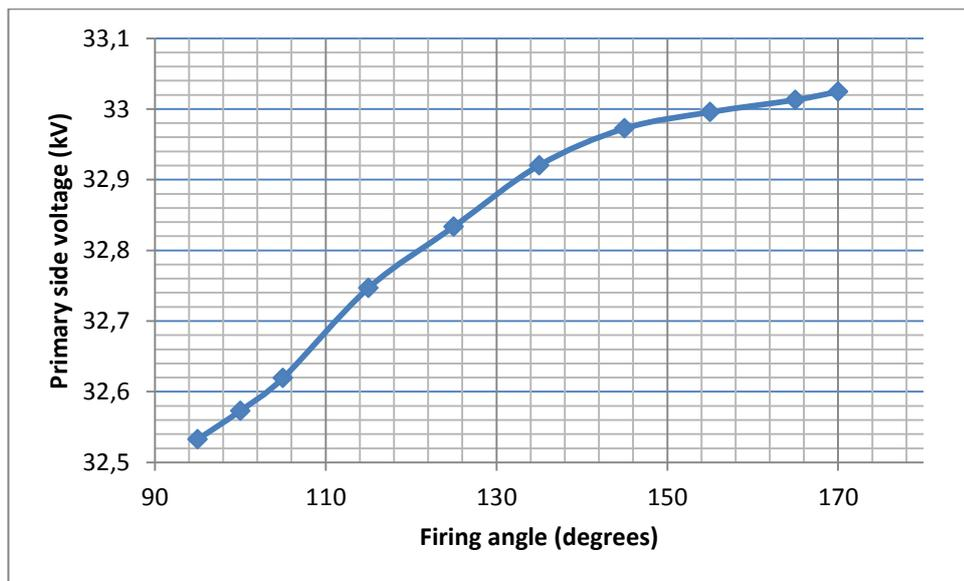
**Figure 5.9:** Voltage versus firing angle relationship with harmonic filters (field data)
