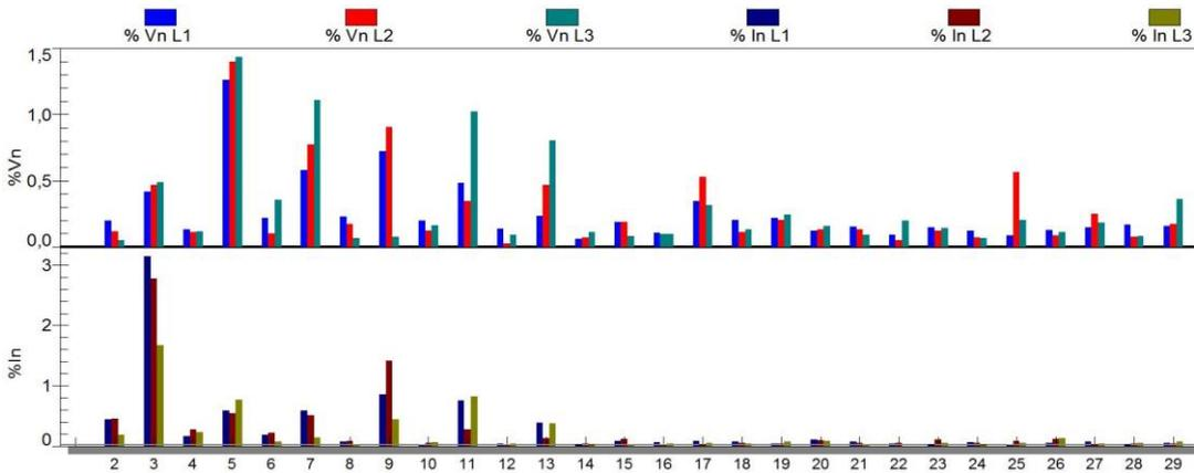
**Figure 5.22:** Current / voltage harmonics at PCC with equal load sharing (field data)
