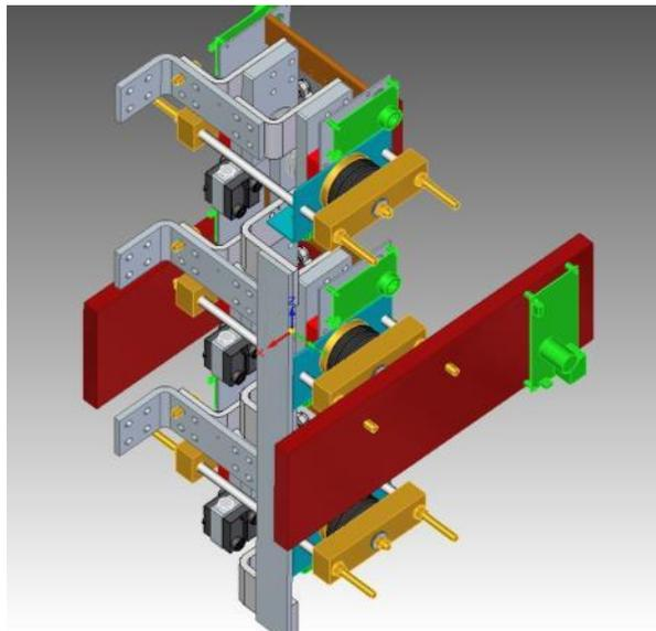
**Figure 3.15:** *Three phase thyristor alignment*
