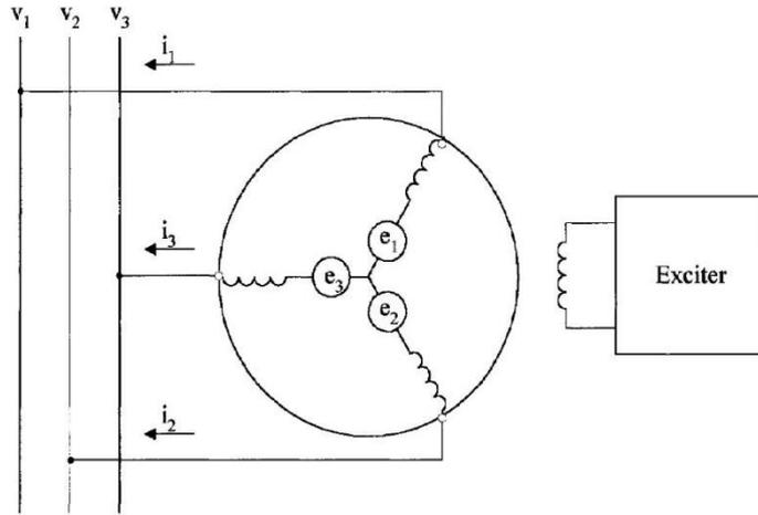
**Figure 1.4:** *Synchronous condenser*
