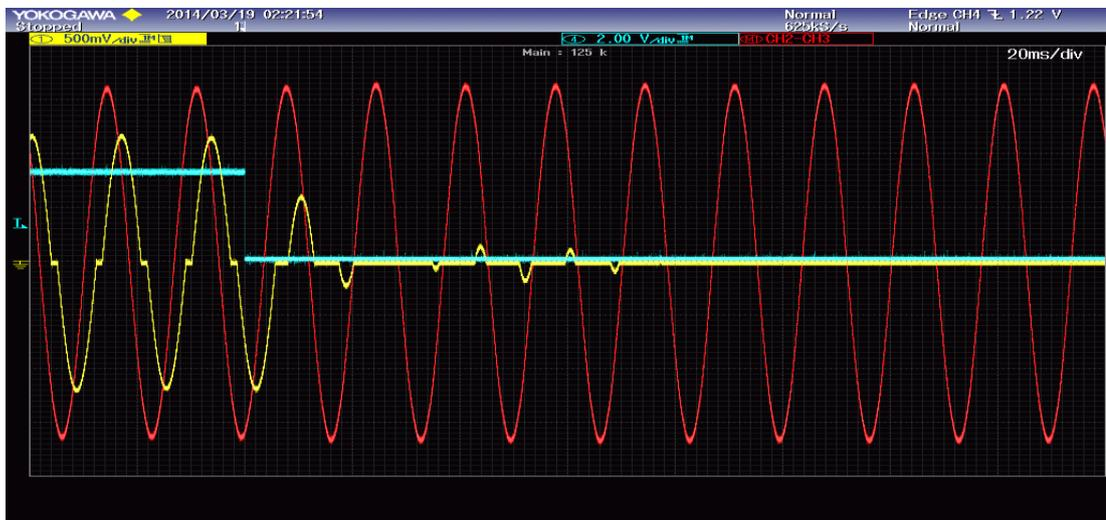
**Figure 5.33:** *Transient response from 32.2kV to 32.9kV*
