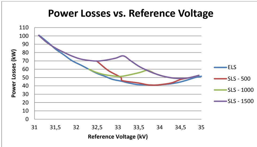
**Figure 4.29:** Power losses according to reference voltage (simulation)
