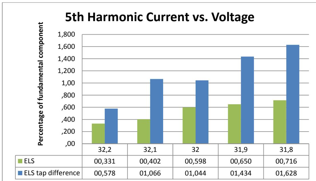
**Figure 5.28:** Relationship between 5<sup>th</sup> harmonic current as percentage of rated current for different taps (field data)
