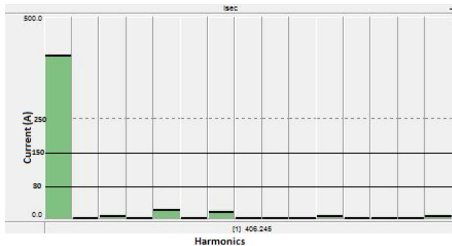
**Figure 4.22:** *Harmonic currents measured from transformer secondary after 3<sup>rd</sup> harmonic filtration (simulation)*
