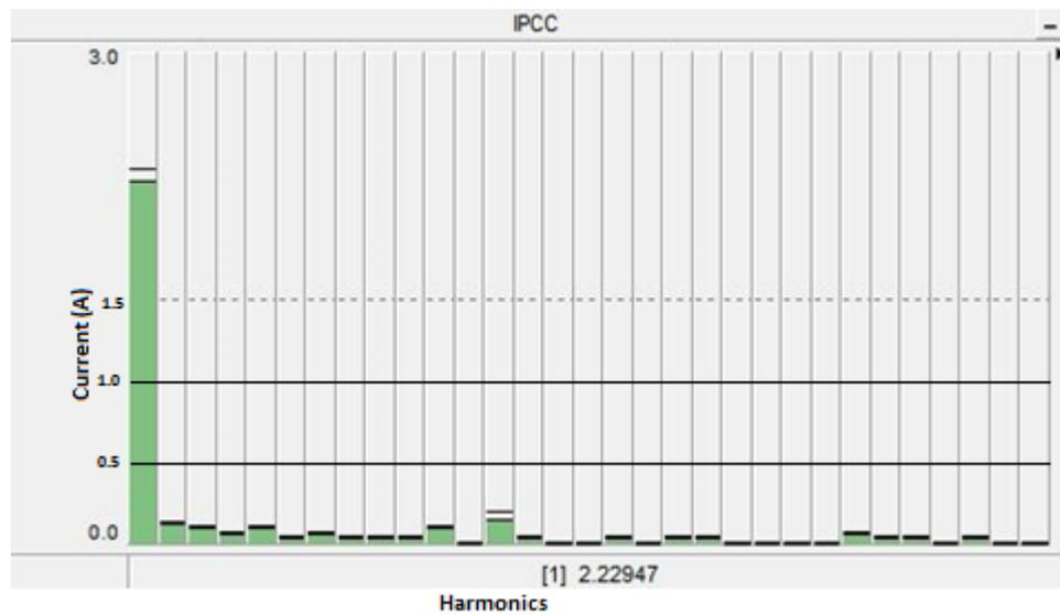
**Figure 4.25:** Current harmonics at PCC with equal load sharing for unbalance (simulation)
