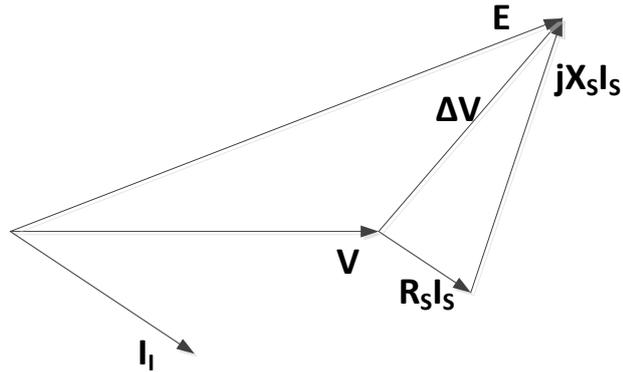
**Figure 2.9:** *Uncompensated load voltage regulation*
