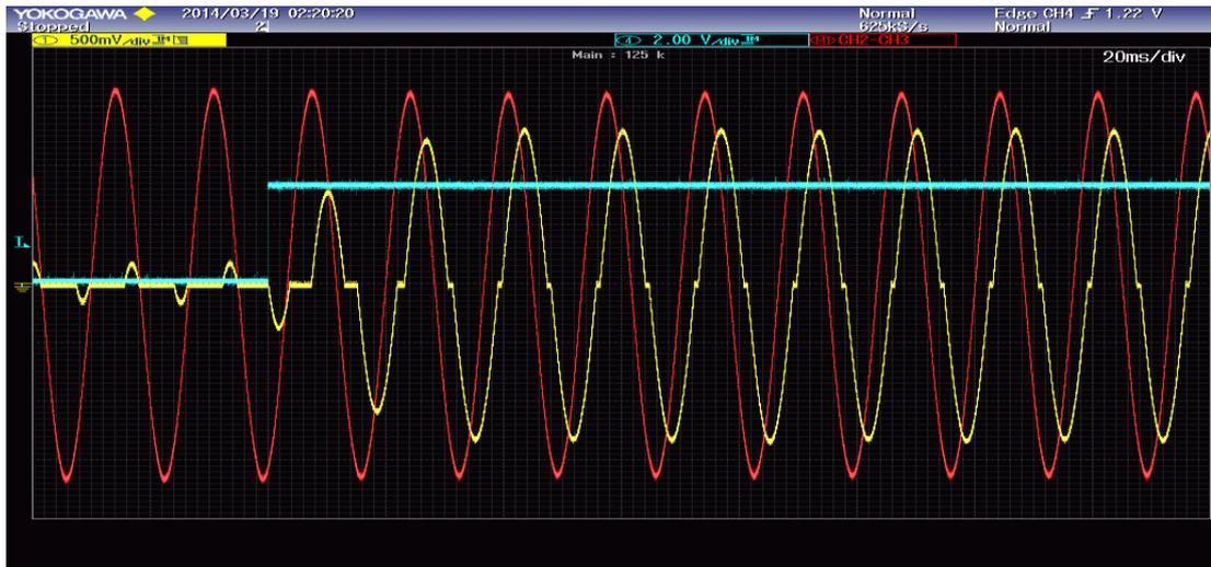
**Figure 5.32:** *Transient response from 32.9kV to 32.2kV*
