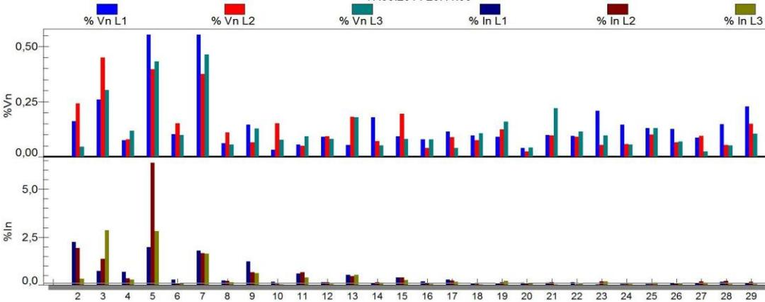
**Figure 5.17:** Current / voltage harmonics at primary side of master with 500kVAr sequential limit (field data)
