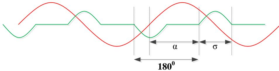
**Figure 2.13:** *Thyristor current and voltage waveforms*
