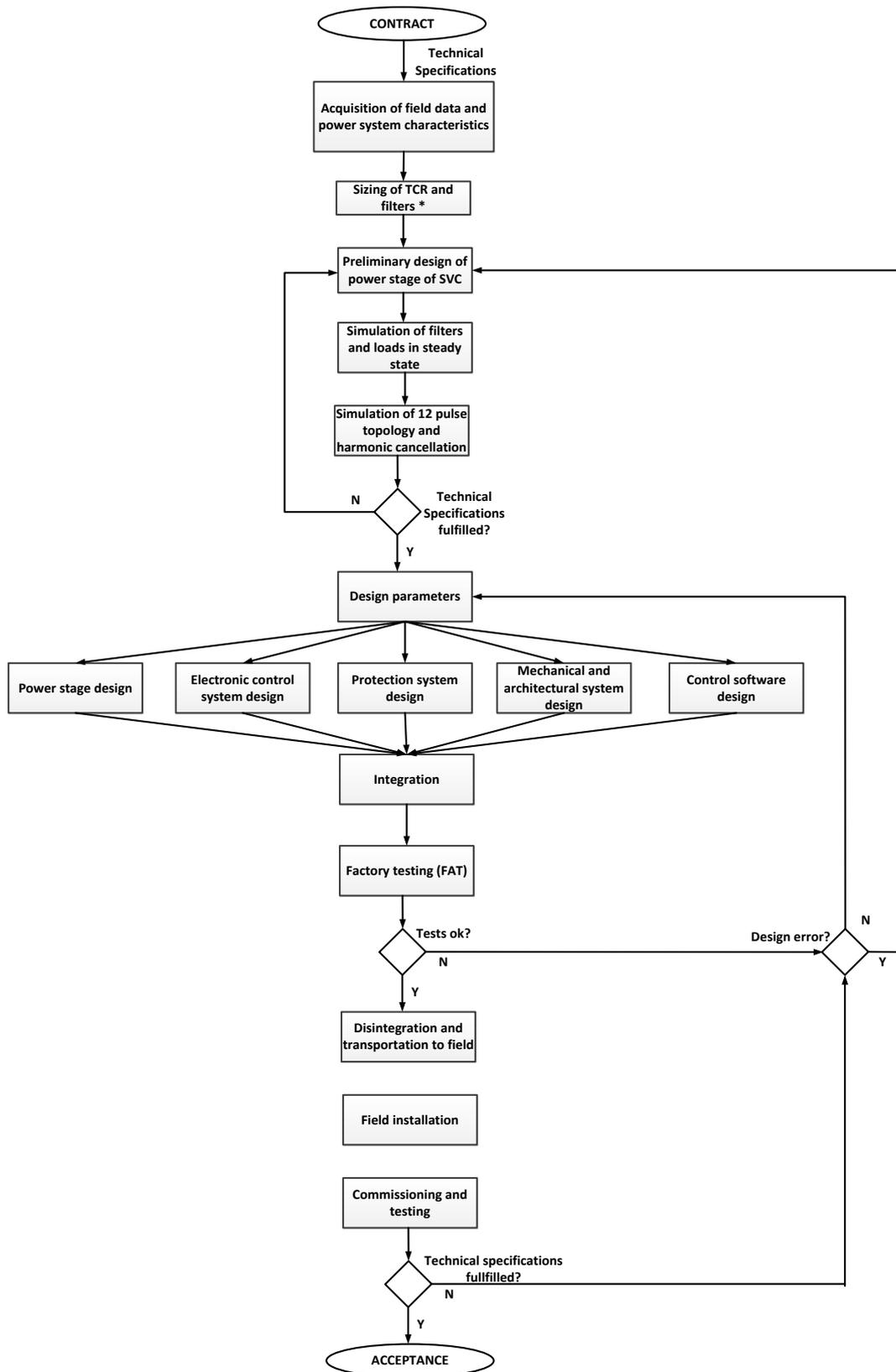
**Figure 3.2:** Design procedure of 12 pulse TCR based SVC for voltage regulation
