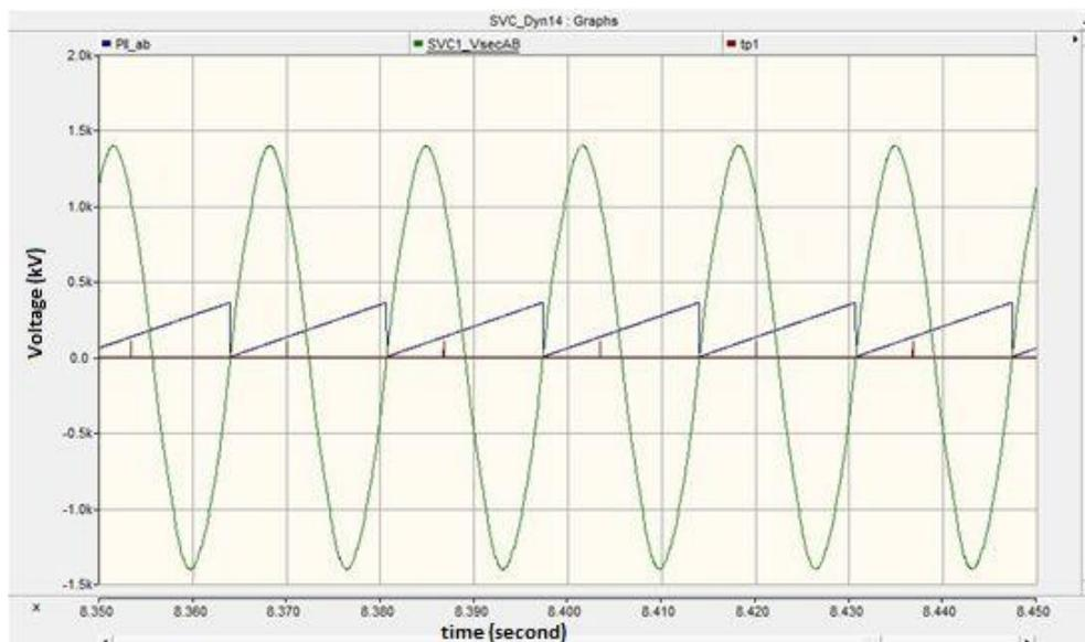
**Figure 4.5:** *Waveforms for firing angle of nearly 115 degrees (simulation)*
