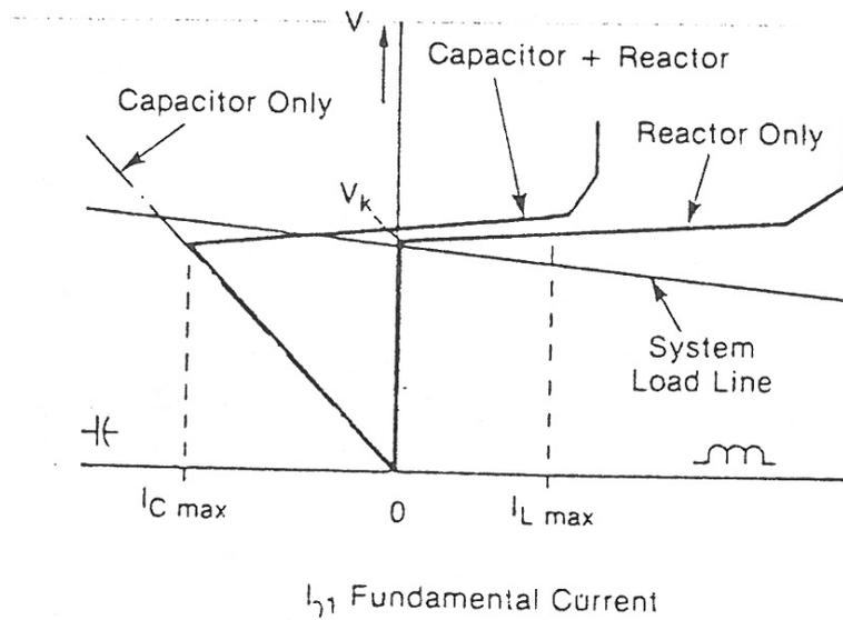
**Figure 2.11:** Voltage / current characteristics of TCR with different combinations [1]
