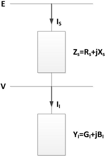
**Figure 2.8:** Basic schematic for load and supply
