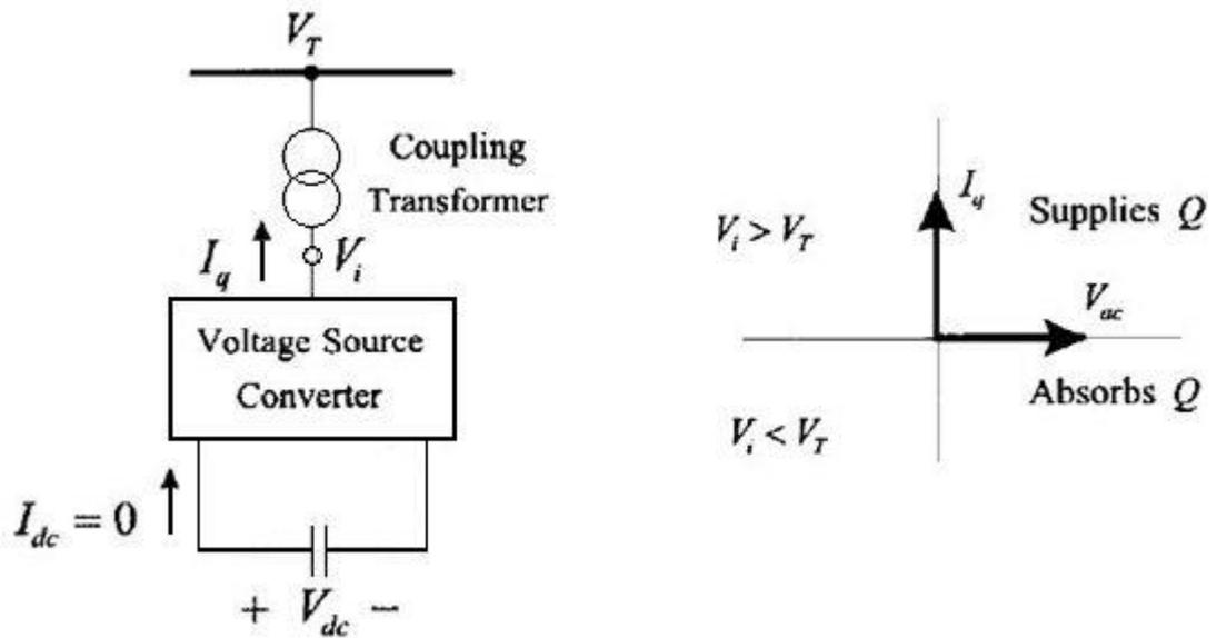
**Figure 1.6:** VSC type STATCOM and its vector diagram
