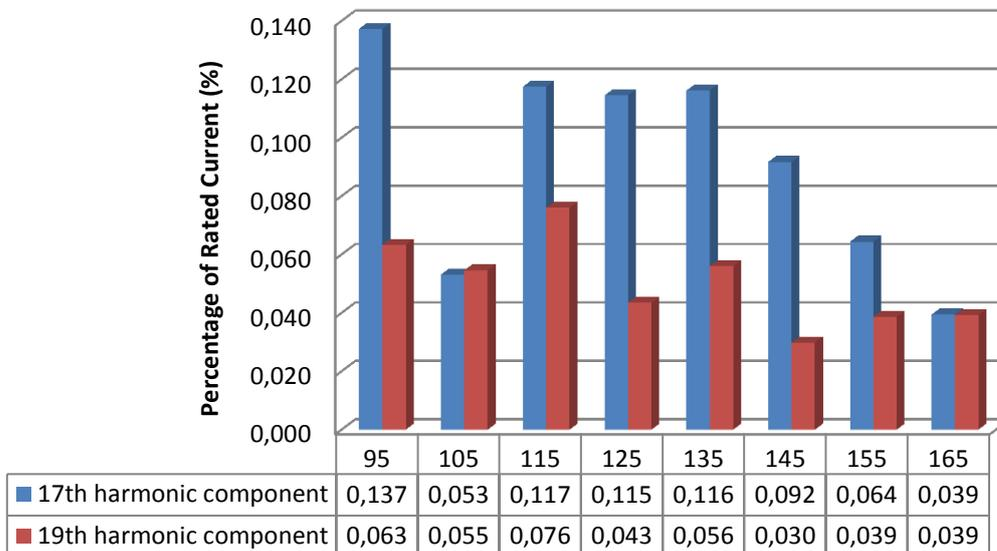
**Figure 5.14:** 17<sup>th</sup> - 19<sup>th</sup> harmonic currents versus firing angle relationship (field data)
