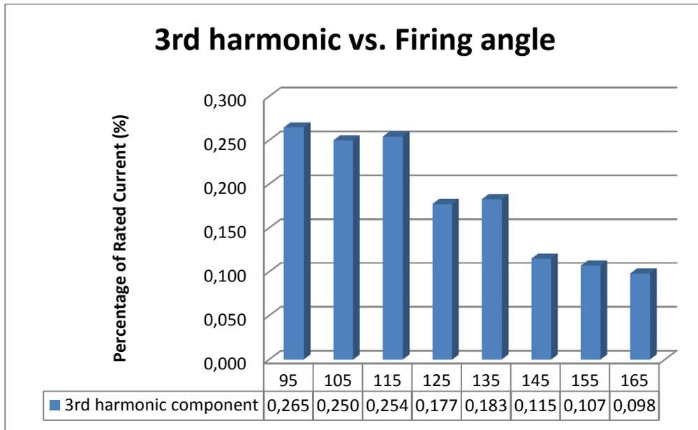
**Figure 5.12:**  $3^{rd}$  harmonic current versus firing angle relationship (field data)
