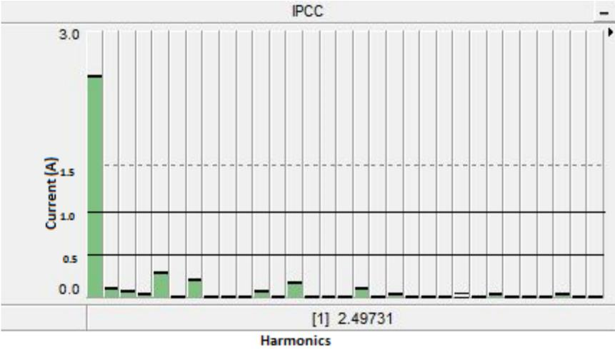
Figure 4.23: Current harmonics at PCC with sequential load sharing (simulation)
