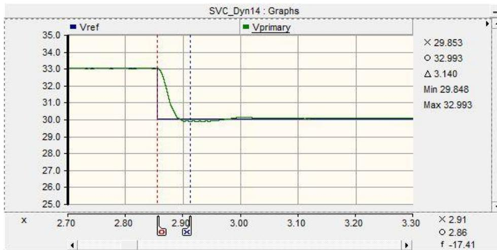
**Figure 4.17:** Critically damped response curve from 33kV to 30kV (simulation)
