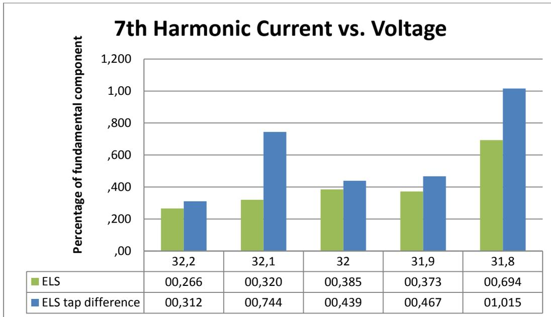
**Figure 5.29:** Relationship between 7<sup>th</sup> harmonic current as percentage of rated current for different taps (field data)
