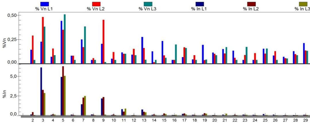
**Figure 5.21:** Current / voltage harmonics at primary side of master with equal load sharing (field data)
