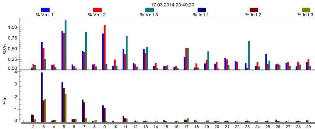
**Figure 5.20:** Current / voltage harmonics at PCC with 1MVAR sequential limit (field data)
