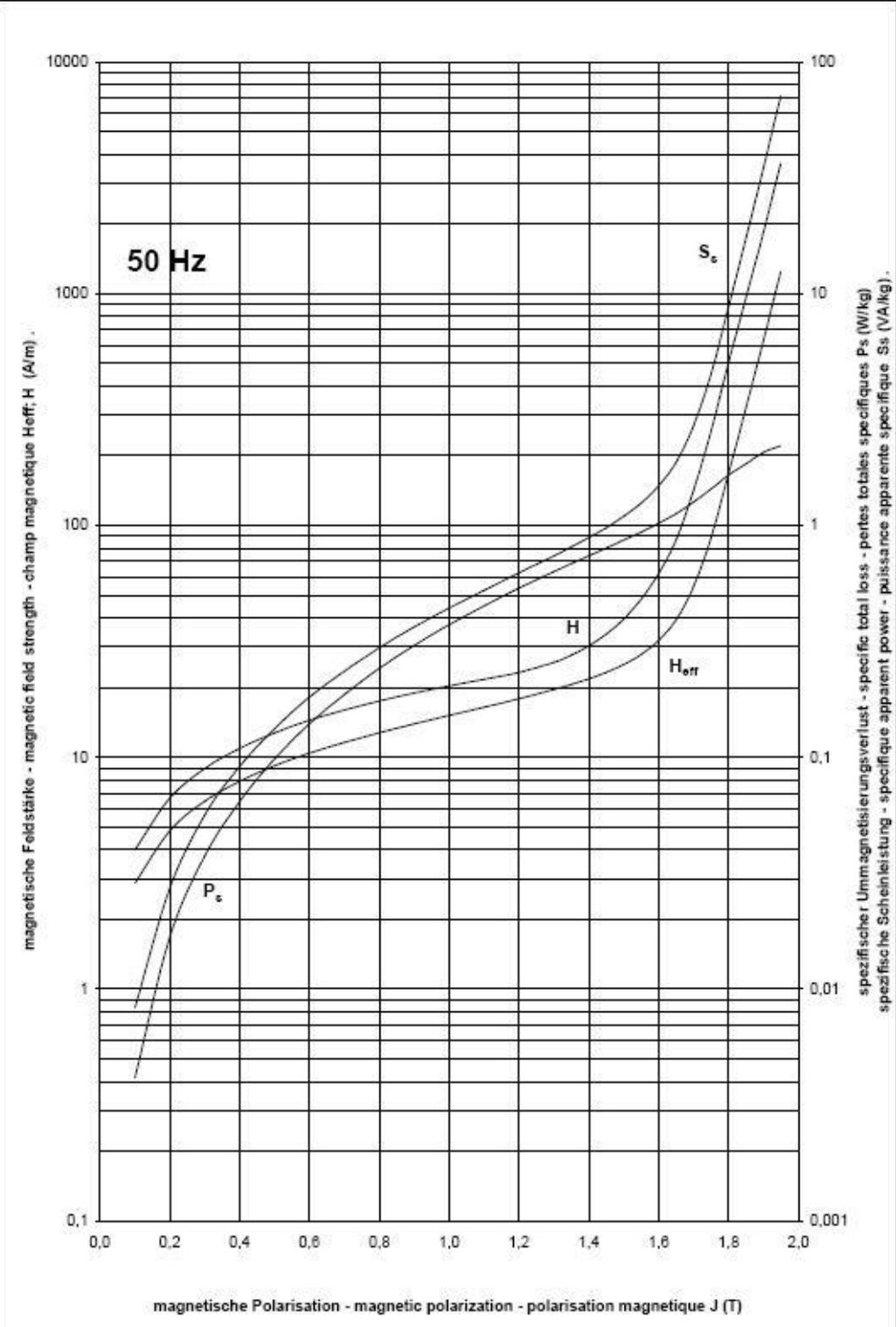
Figure 3.16: B-H characteristics of coupling transformer
