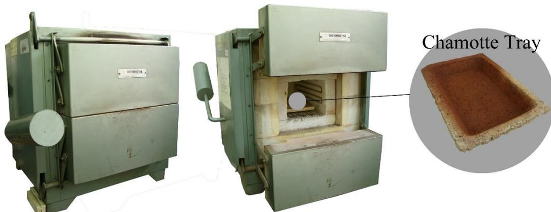
*Figure 3-2. Photograph of the muffle furnace and chamotte tray used in the calcination experiments.*
