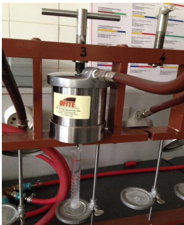
Figure 4. 3: Fluid loss measurement
