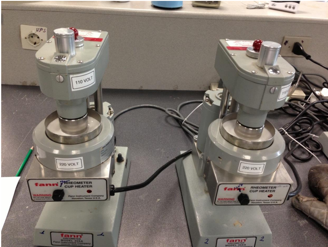
Figure 4. 2: Rheology measurements with Fann viscometers
