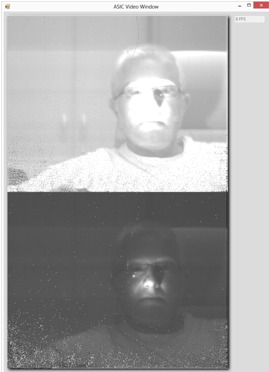
Figure 4.7: Video screen capture with two different exposure settings. The upper picture represents the image with 20 ms exposure time and the bottom picture represents the image with 5 ms exposure time.
