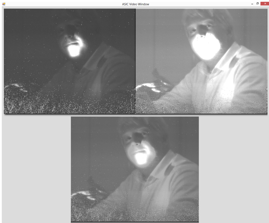
Figure 4.8: Video screen capture with two different exposure settings and average of the two images. The bottom picture is constructed from the top two images which are 5 ms exposed image and 20 ms exposed image, respectively.
