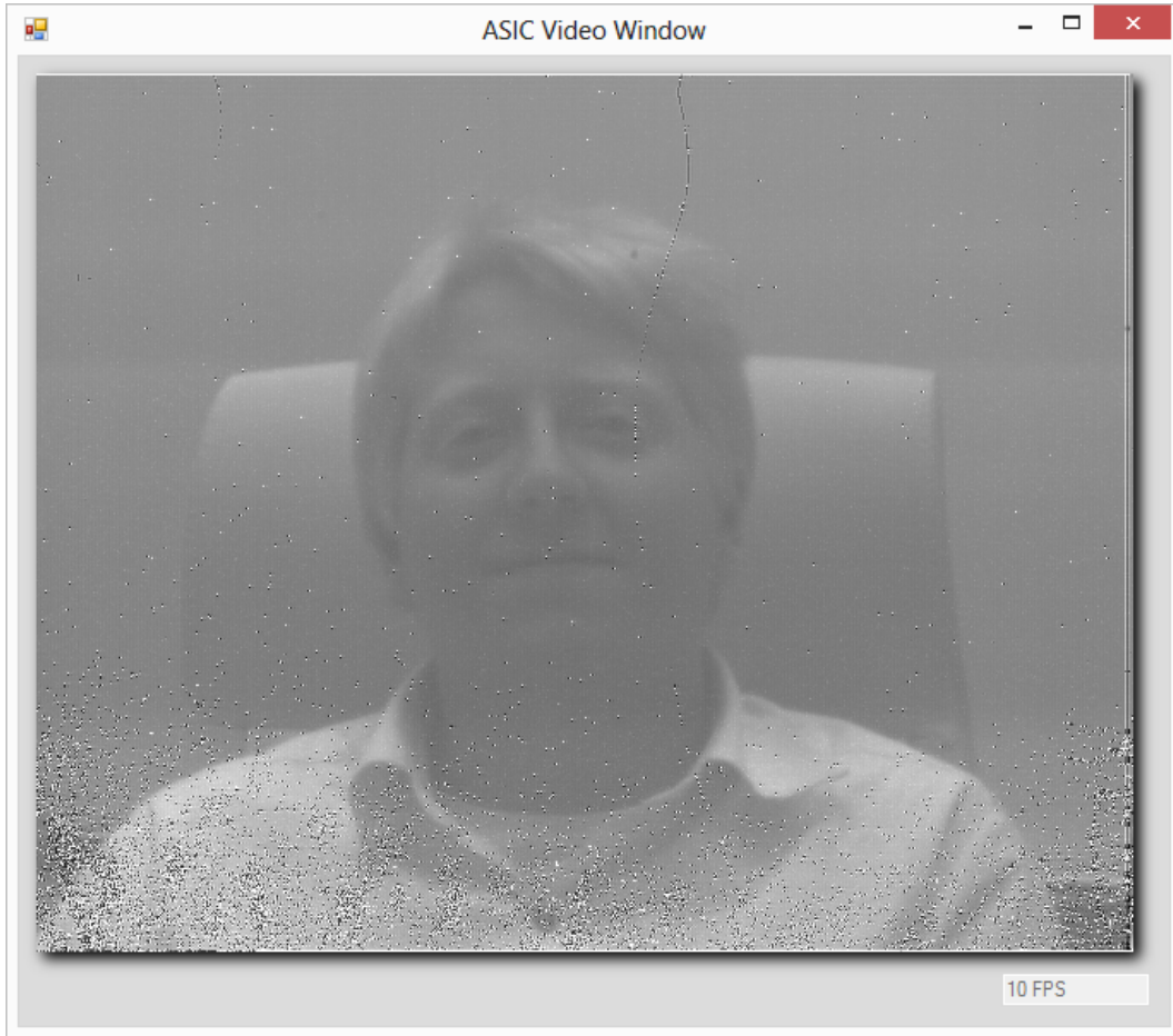
Figure 4.12: Video screen capture of the event for which the normalization is implemented on the video data. For this test, N_{MeanRange} is programmed as 4096 and N_{MeanMin} is programmed as 9000.
