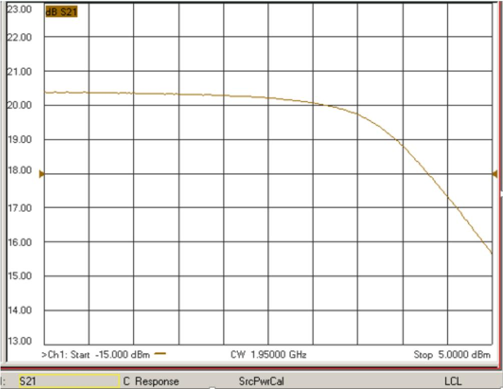
Figure 3-15 AM-AM characteristics of the amplifier GVA-63+
