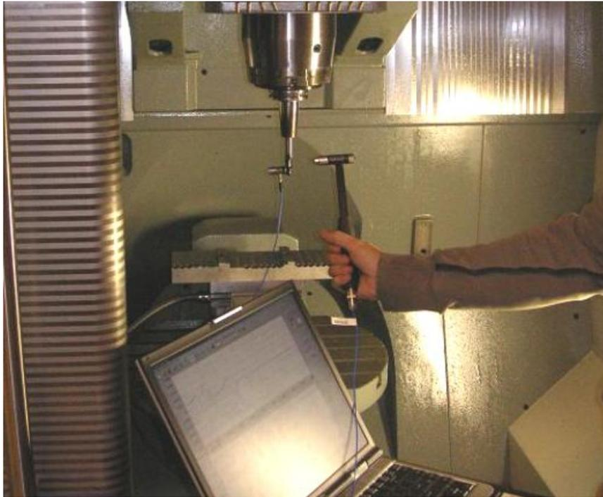
Figure 1-4 Tool point FRF measurement using impact test [14].
