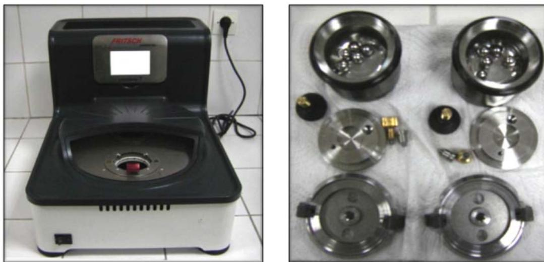
**Figure 31** Fritsch Pulveristte 7 Premium Line High Energy Ball Mill, stainless steel bowls/balls with no controlled atmosphere.
