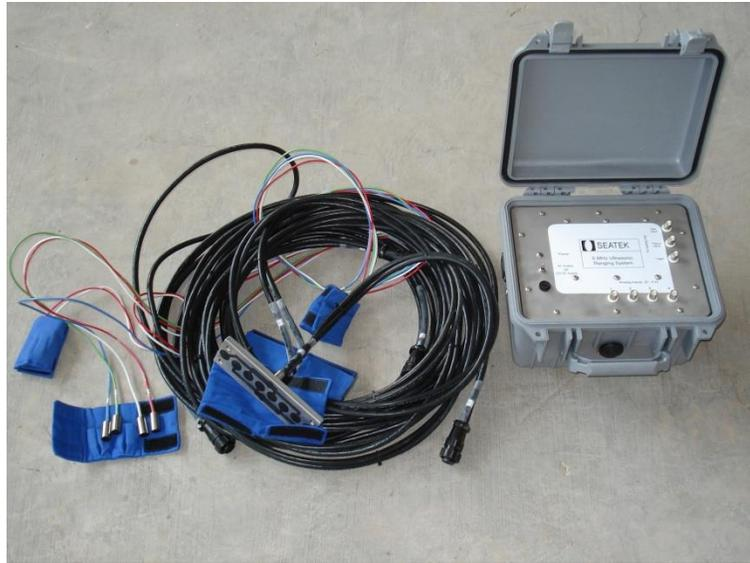
Figure 3.2 Seatek Ultrasonic Ranging System
