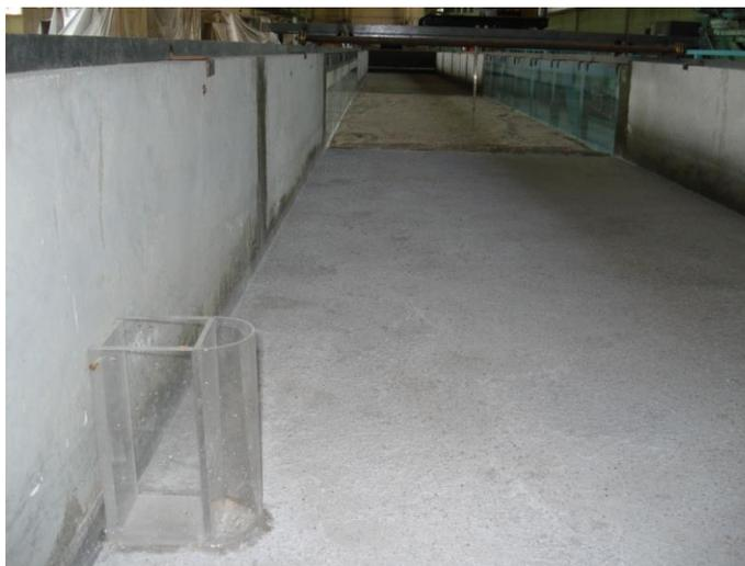
Figure 5.3 Picture of a SCE abutment model at the non-erodible part of the flume
