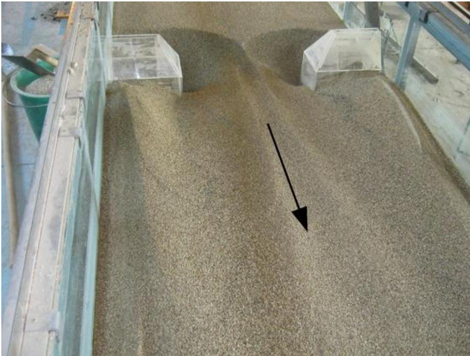
Figure 4.2 A view of the flume and scour pattern when  $\beta= 0.452$  and  $t= 2$  hrs
