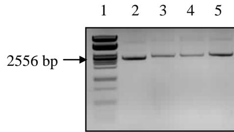
**Figure 11** Isolated plasmids from white colonies. Lane 1: Marker (Lambda DNA/PstI, 24), Lane 2: pQE60 vector as control, Lane 3-4: pGEM®-T carrying *glnH*, Lane 5: pGEM®-T carrying BP0020.
