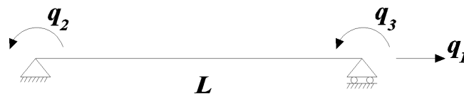
Figure 3 Simply supported basic system for force-based beam element
