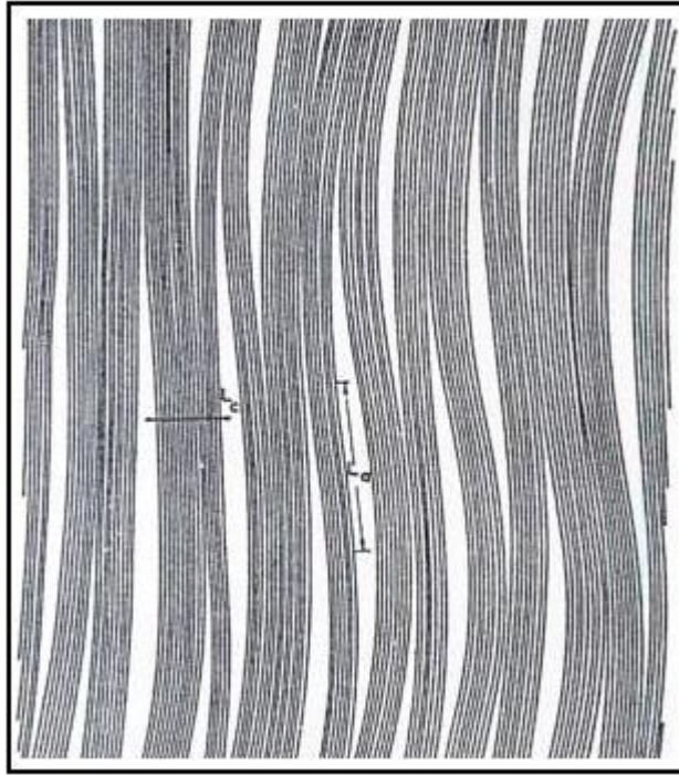
Figure 10. Schematic of PAN-based carbon fiber lied along the fiber axis [39]
