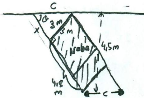
$$\begin{aligned} C. 4,5 \text{ m} &= 3. (x+4,8 \text{ m}) \\ C &= \sqrt{x^2+9} \\ 3 \cdot 4,5 \cdot \sqrt{x^2+9} &= 3 \cdot (x+4,8) \\ 3\sqrt{x^2+9} &= 2(x+4,8) \\ (3\sqrt{x^2+9})^2 &= (2x+9,6)^2 \\ 9(x^2+9) &= 4x^2+38,4x+92,16 \\ 9x^2+81 &= 4x^2+38,4x+92,16 \\ 5x^2-38,4x-92,16 &= 0 \end{aligned}$$
