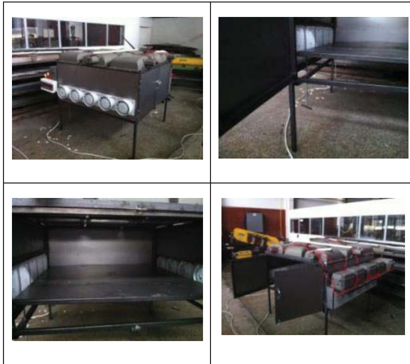
Figure 3-11 The Final Construction of the Light Soaking Station
