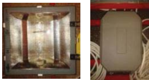
Figure 3-6 Picture of the single light source and the starter
