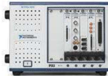
Figure 3-5 Picture of the Chassis with the cards installed
