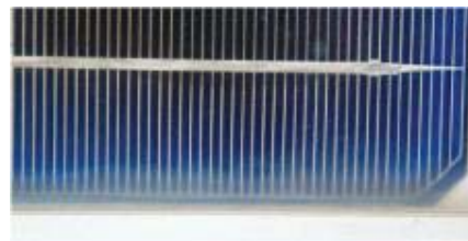
Figure 1-17 Haziness that could be seen at the edge of the cell
