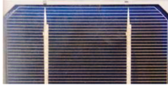
Figure 1-20 AR coating oxidation through the center of the cell
